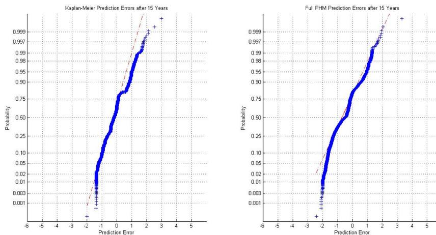
FIGURE 7.6: Normal probability plots associated with prediction errors of Kaplan-Meier and PHM models applied to concrete deck condition rating data
