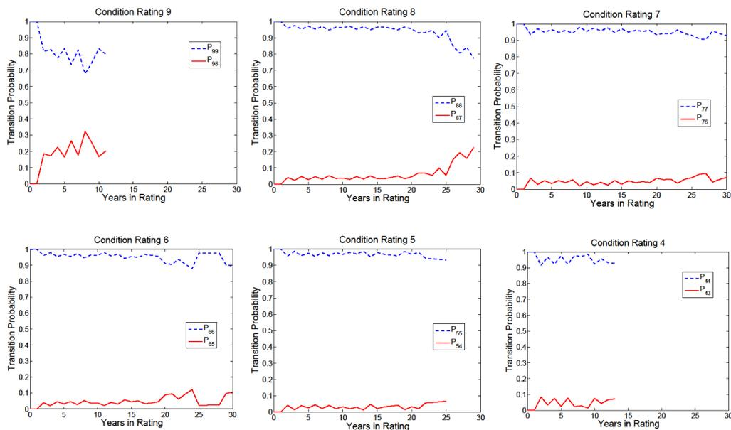
FIGURE 6.7: Timber deck baseline transition probabilities
