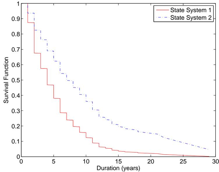
FIGURE 3.4: Survival functions for timber decks in condition rating 4 based on the covariate ‘State System’
