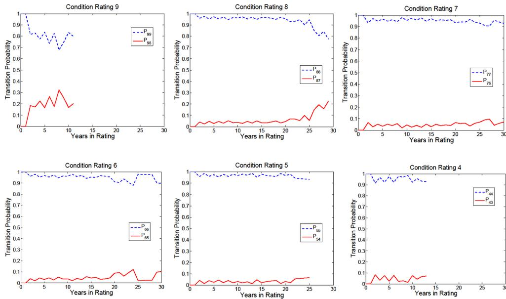
FIGURE 4.5: Baseline transition probabilities for timber deck across condition ratings 9 through 4
