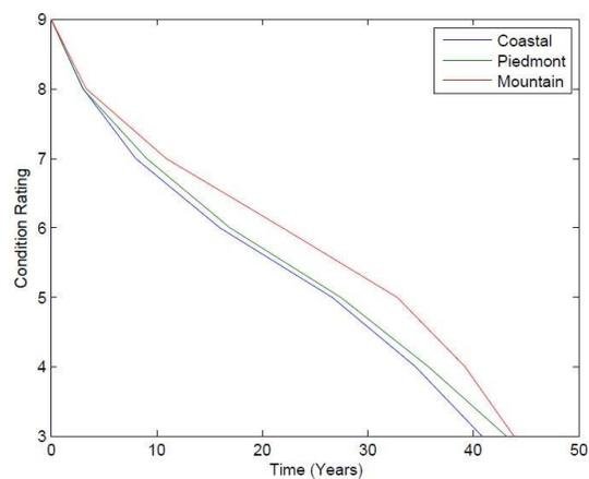
FIGURE 6.43: Concrete substructure deterministic deterioration models
