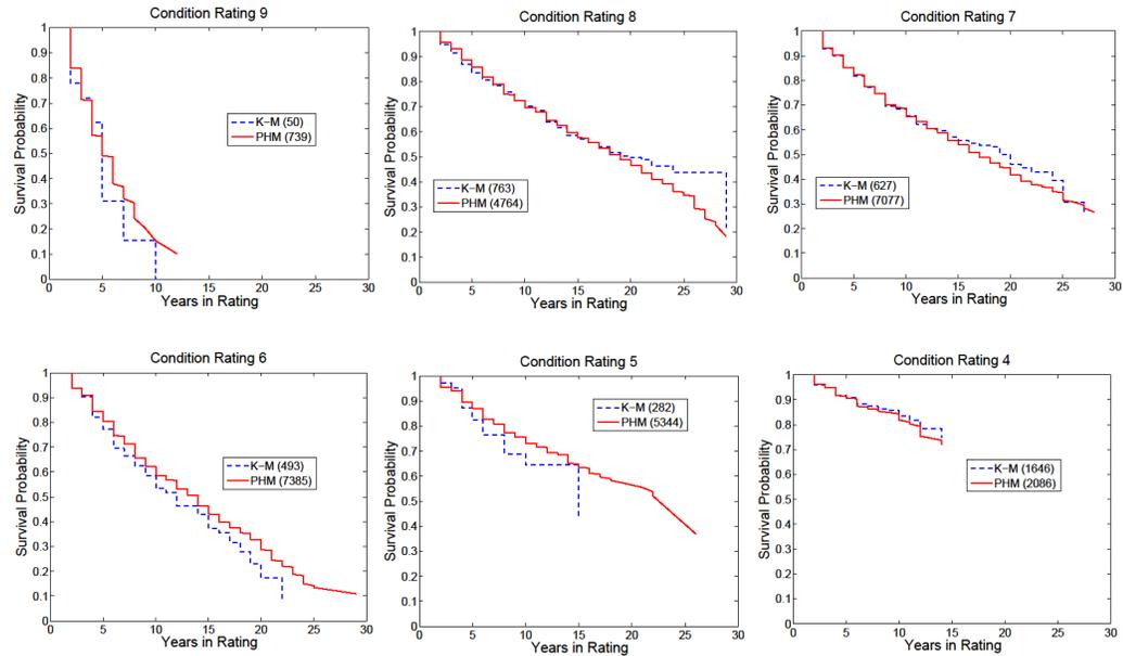
FIGURE 4.4: Timber deck survival functions: model vs empirical
