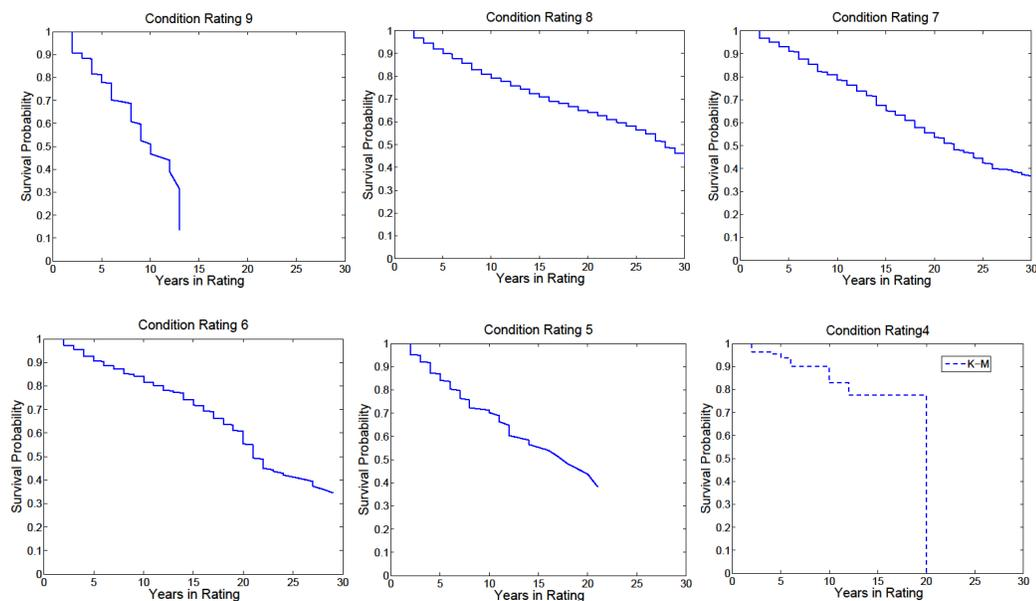
FIGURE 6.27: Prestressed concrete superstructure baseline survival functions
