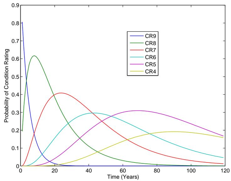
FIGURE 4.7: Condition rating probabilities for timber deck from stationary Markov process
