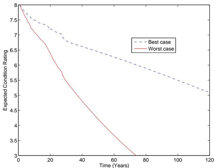
FIGURE 6.41: Concrete superstructure forecast models for best case (State System 1, Mountain region, max span < 3m, single span, age < 32 years) and worst case (State System 2, Piedmont region, max span  $\geq$  5m, multi span, age  $\geq$  58 years) combination of covariates
