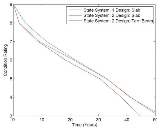
FIGURE 6.21: Concrete superstructure deterministic deterioration models
