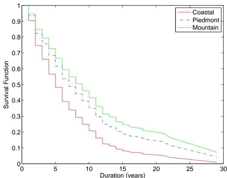
FIGURE 3.5: Timber deck survival functions for condition rating 4 and covariate ‘Region’
