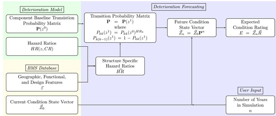
FIGURE 4.10: Proportional hazards model prediction flowchart
