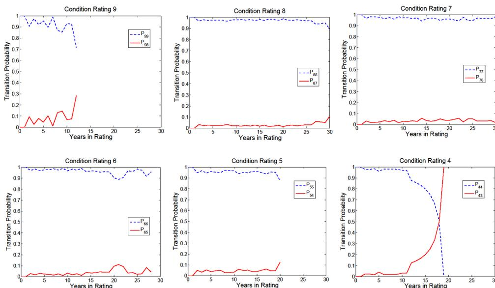
FIGURE 6.37: Prestressed concrete superstructure baseline transition probabilities
