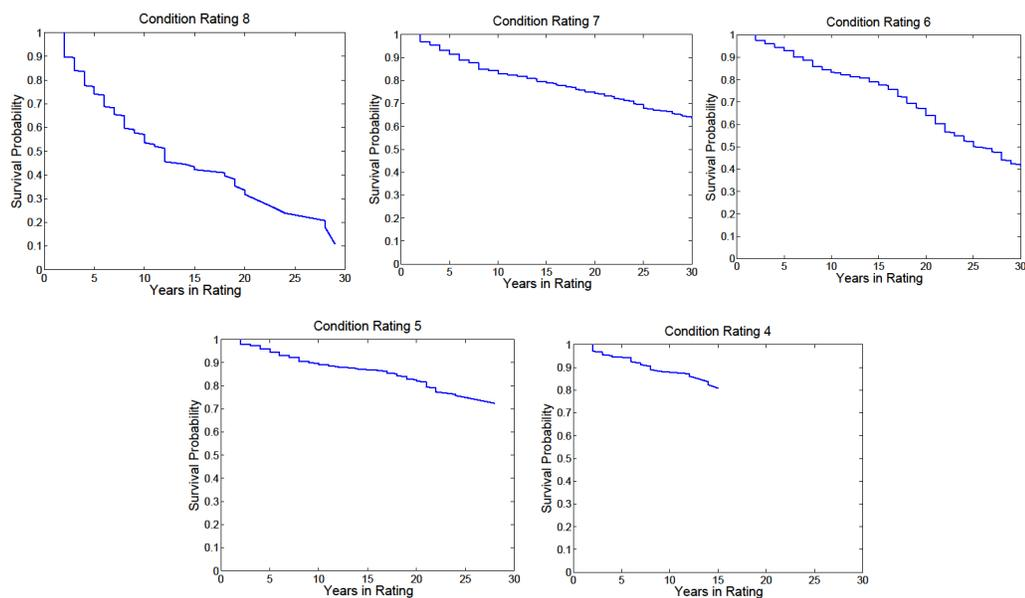
FIGURE 6.25: Concrete superstructure baseline survival functions
