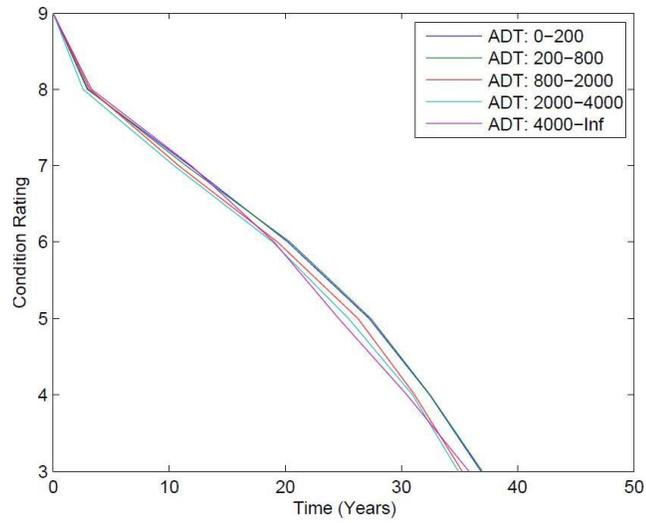
FIGURE 6.1: Timber deck deterministic deterioration models
