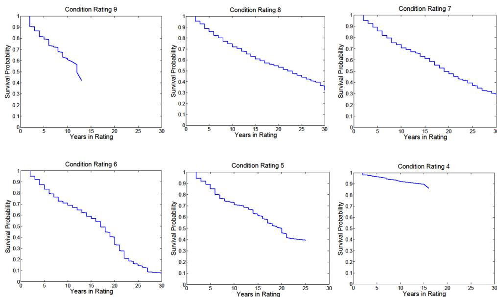
FIGURE 6.48: Steel substructure baseline survival functions
