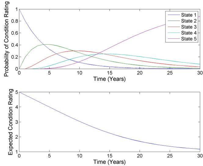
FIGURE 2.2: A Markovian bridge deterioration model.
