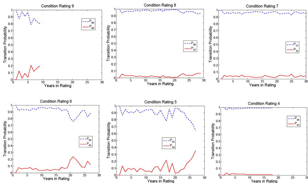
FIGURE 6.59: Prestressed concrete substructure baseline transition probabilities
