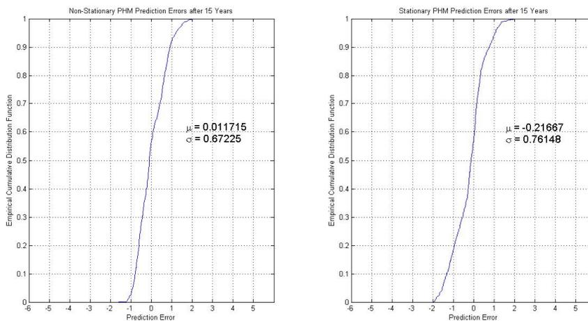
FIGURE 7.10: Empirical cumulative distribution functions associated with prediction errors of non-stationary and stationary PHM models applied to concrete deck condition rating data
