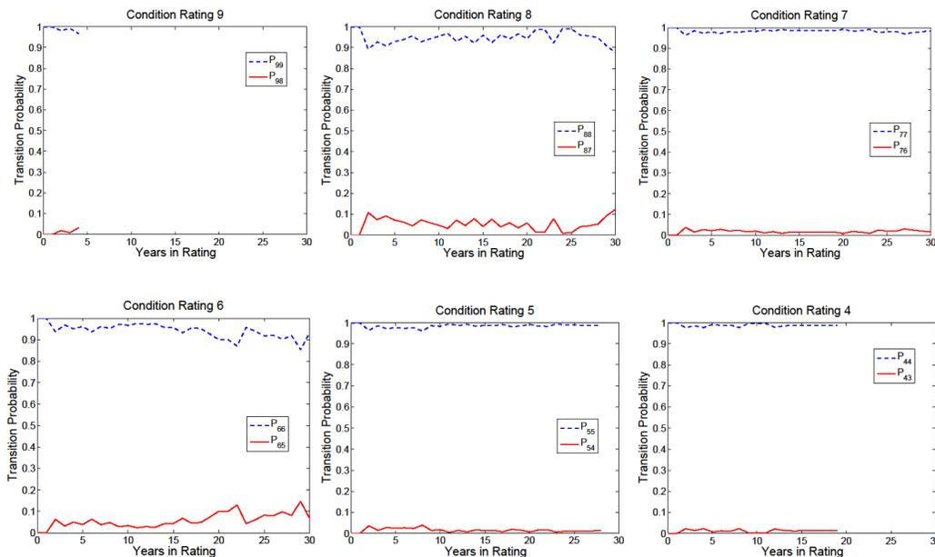
FIGURE 6.53: Concrete substructure baseline transition probabilities
