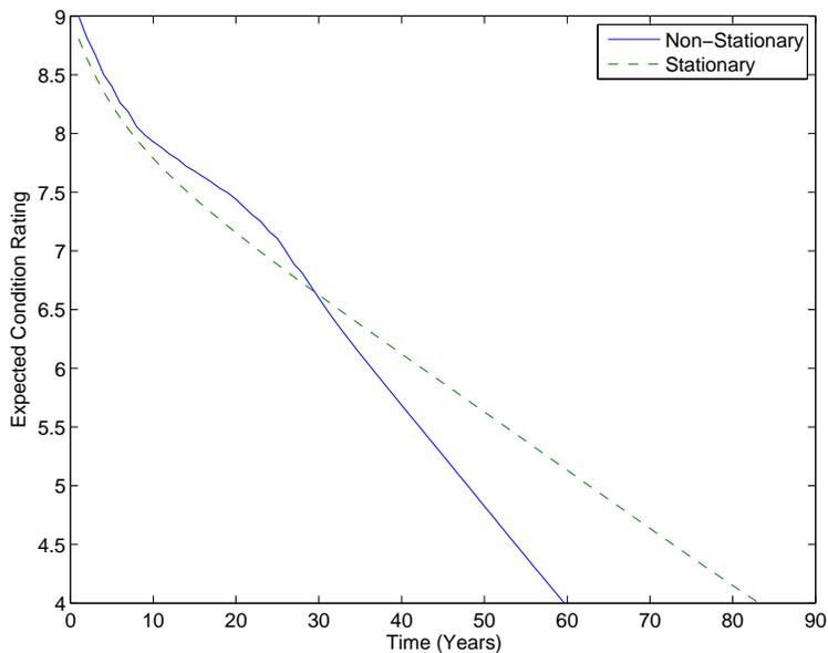
FIGURE 4.8: Expected values of condition rating for timber deck determined using stationary and non-stationary transition probabilities
