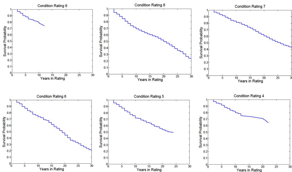
FIGURE 6.26: Steel superstructure baseline survival functions
