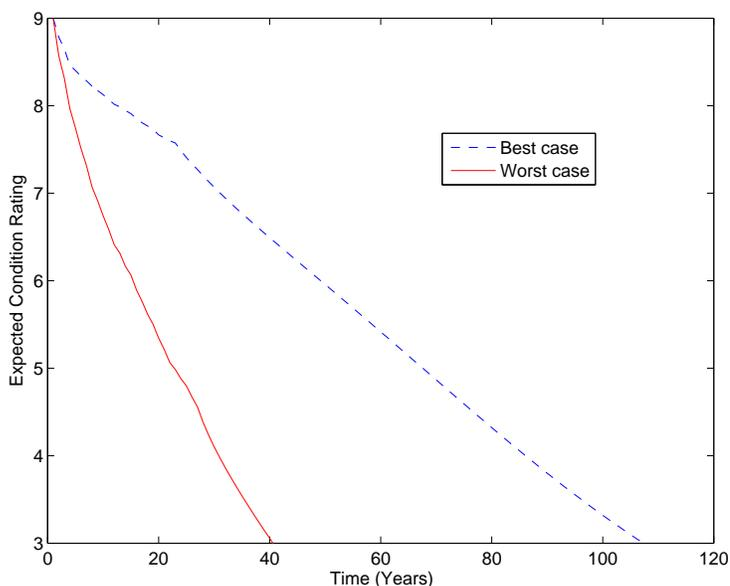
FIGURE 6.62: Timber substructure forecast models for best case (State System 1, original/rebuilt, Mountain region, max span 2 – 3m, single span, age < 21 years) and worst case (State System 2, reconstructed, Piedmont region, max span < 2m, multi span, age  $\geq 36$  years) combination of covariates
