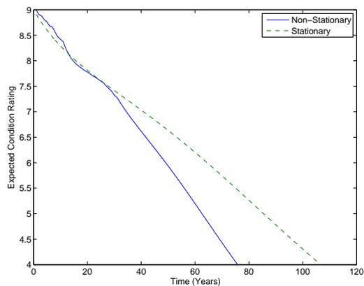
FIGURE 6.39: Prestressed concrete superstructure baseline prediction model
