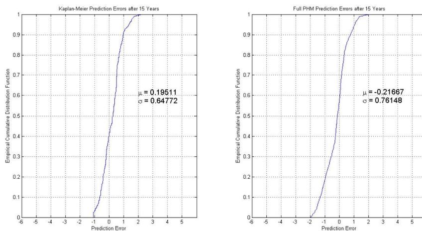
FIGURE 7.9: Empirical cumulative distribution functions associated with prediction errors of concrete deck Kaplan-Meier and PHM models obtained with split probability initial state vector
