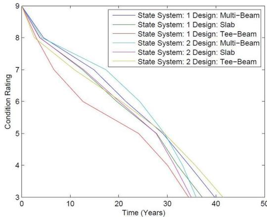
FIGURE 6.23: Prestressed concrete superstructure deterministic deterioration models
