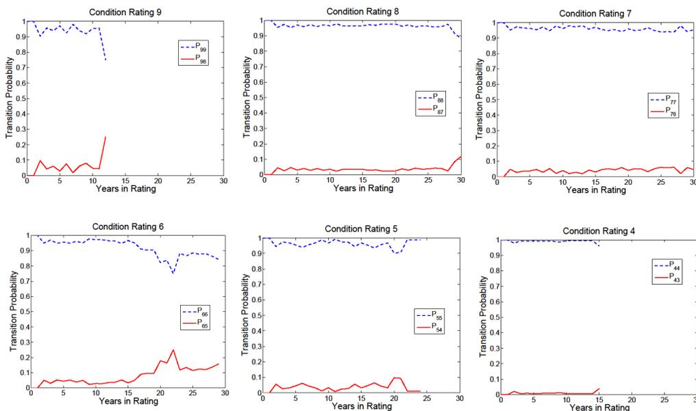
FIGURE 6.56: Steel substructure baseline transition probabilities
