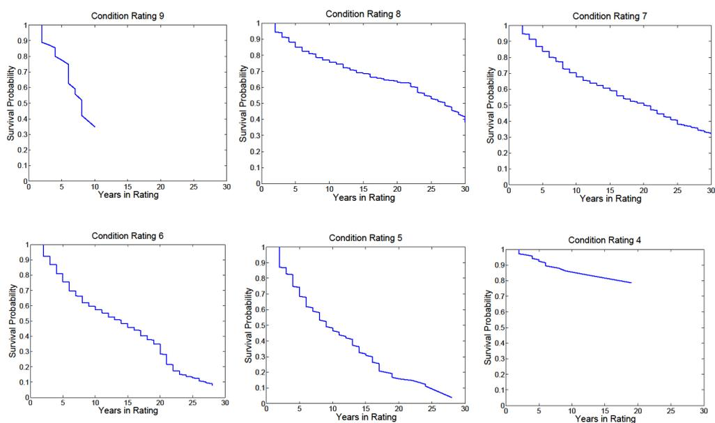
FIGURE 6.49: Prestressed concrete substructure baseline survival functions
