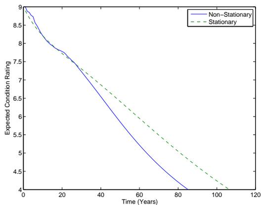
FIGURE 6.61: Prestressed concrete substructure baseline prediction model
