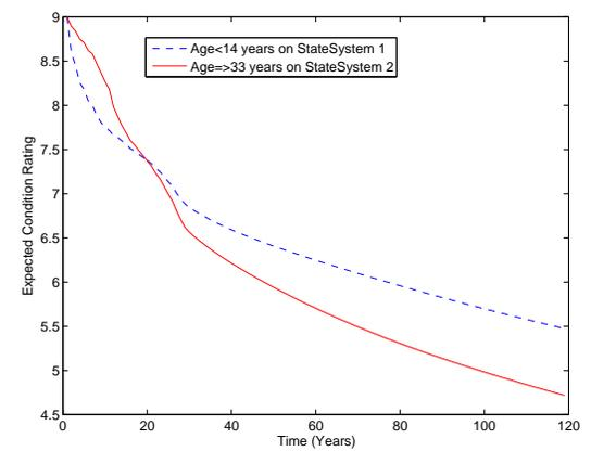
FIGURE 6.19: Effect of age and State System on concrete deck deterioration rates
