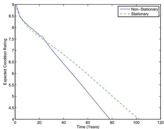
FIGURE 6.52: Timber substructure baseline prediction model
