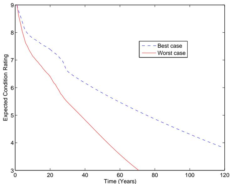
FIGURE 6.40: Timber superstructure forecast models for best case (State System 1, reconstructed, Piedmont region, ADT 239 – 555, ADTT < 6, max span < 2m, single span, age < 22 years) and worst case (State System 2, original/rebuilt, Coastal region, ADT < 102, ADTT 15 – 34, max span  $\geq$  2m, multi span, age  $\geq$  36 years) combination of covariates
