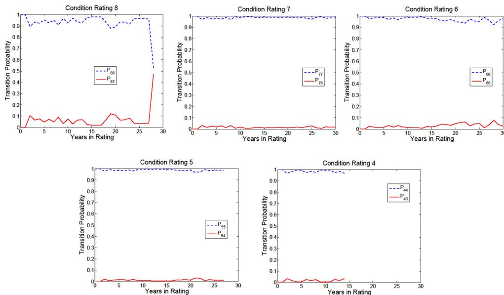
FIGURE 6.31: Concrete superstructure baseline transition probabilities
