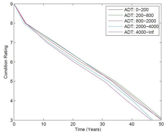
FIGURE 6.2: Concrete deck deterministic deterioration models
