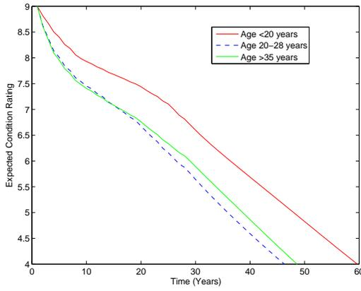
FIGURE 6.16: Effect of age on timber deck deterioration rates
