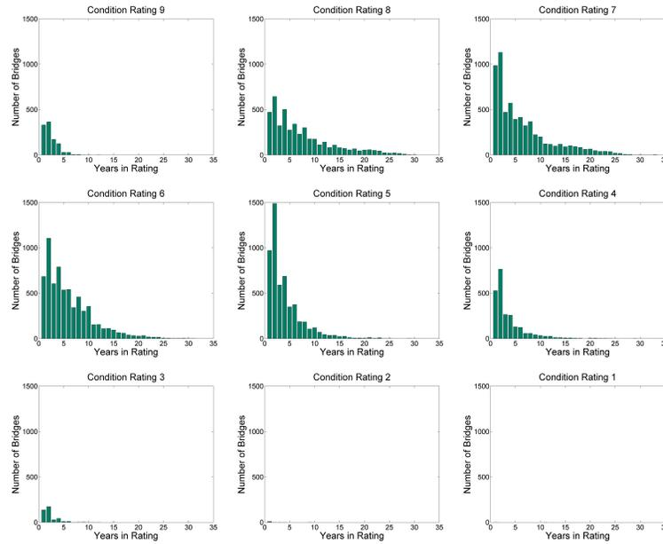
FIGURE 1.2: Distributions of observed continuous condition rating durations for all timber bridge decks in the 1981-2013 NCDOT bridge records
