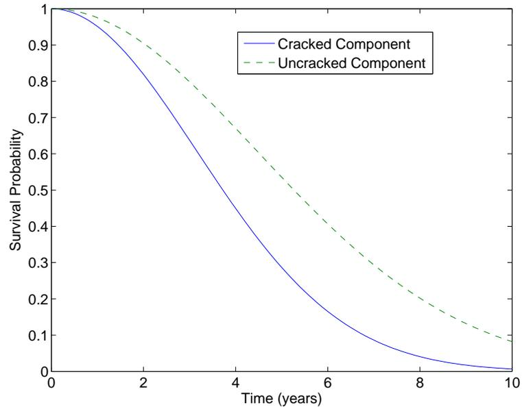
FIGURE 3.3: Survival functions for fatigue failure of structural components
