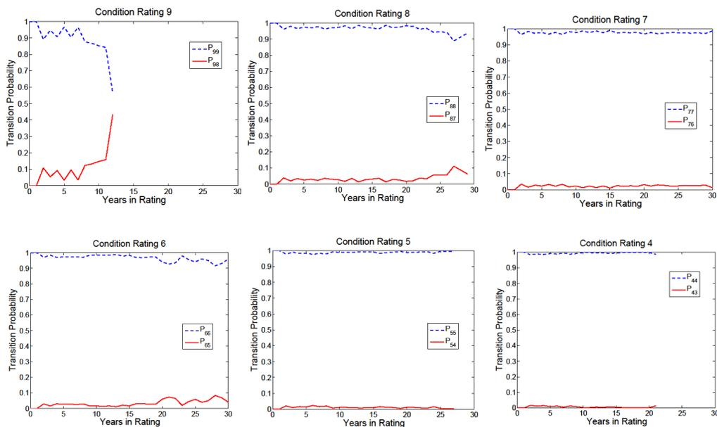
FIGURE 6.10: Concrete deck baseline transition probabilities
