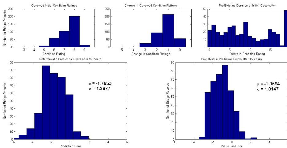
FIGURE 7.4: Histograms of steel deck condition rating data in observation period and prediction errors
