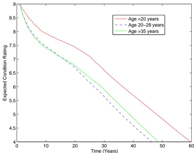
FIGURE 4.9: Expected condition rating prediction of timber deck bridges in different age groups
