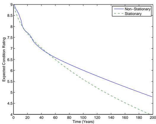
FIGURE 6.12: Concrete deck baseline prediction model
