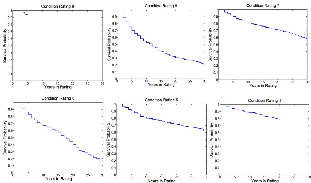
FIGURE 6.47: Concrete substructure baseline survival functions
