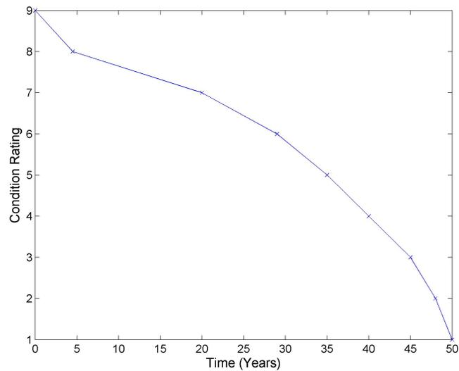
FIGURE 2.1: A deterministic bridge deterioration model.
