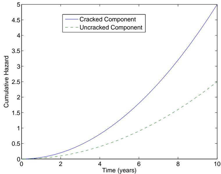
FIGURE 3.2: Cumulative hazard functions for fatigue failure of structural components
