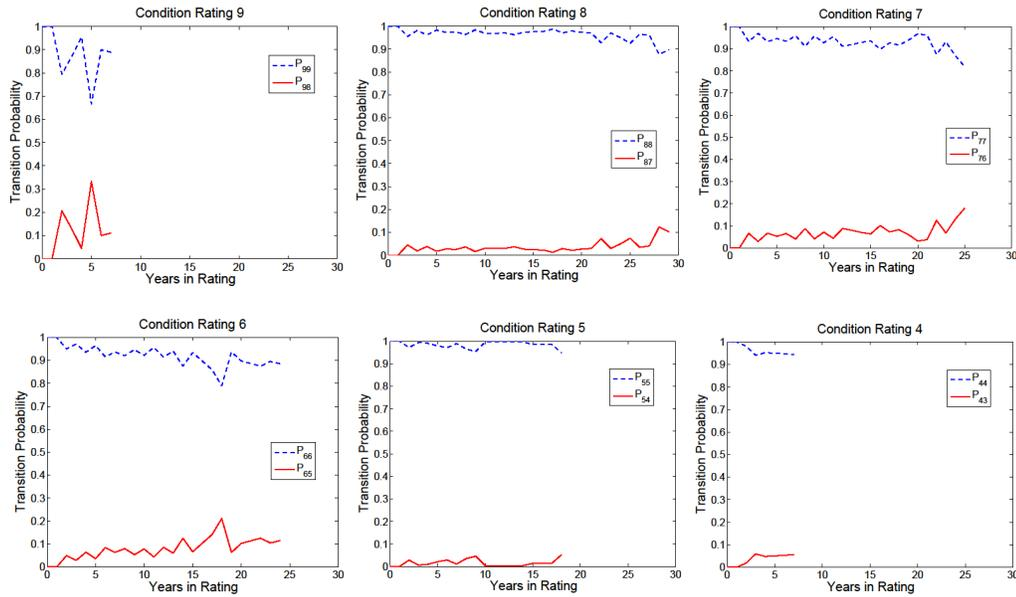
FIGURE 6.13: Steel deck baseline transition probabilities
