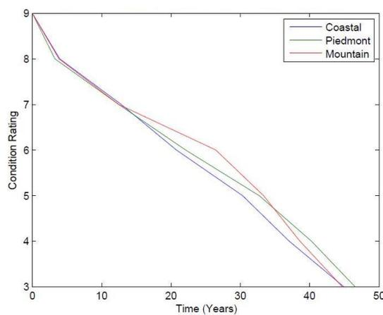
FIGURE 6.45: Prestressed concrete substructure deterministic deterioration models
