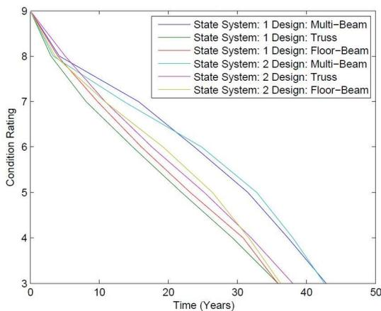
FIGURE 6.22: Steel superstructure deterministic deterioration models
