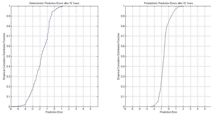
FIGURE 7.2: Empirical cumulative distribution functions associated with prediction errors of deterministic and probabilistic models applied to timber deck condition rating data
