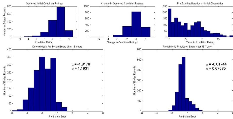
FIGURE 7.1: Histograms of timber deck condition rating data in observation period and prediction errors
