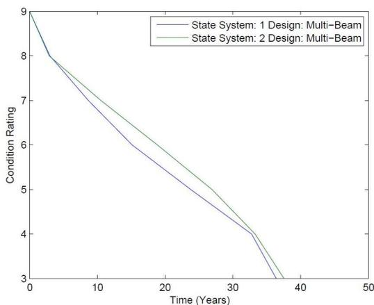
FIGURE 6.20: Timber superstructure deterministic deterioration models
