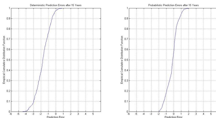
FIGURE 7.8: Empirical cumulative distribution functions associated with prediction errors of concrete deck deterministic and probabilistic models obtained with split probability initial state vector
