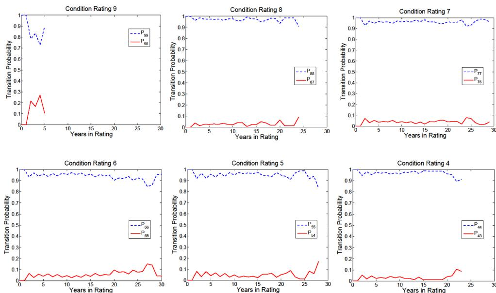
FIGURE 6.50: Timber substructure baseline transition probabilities
