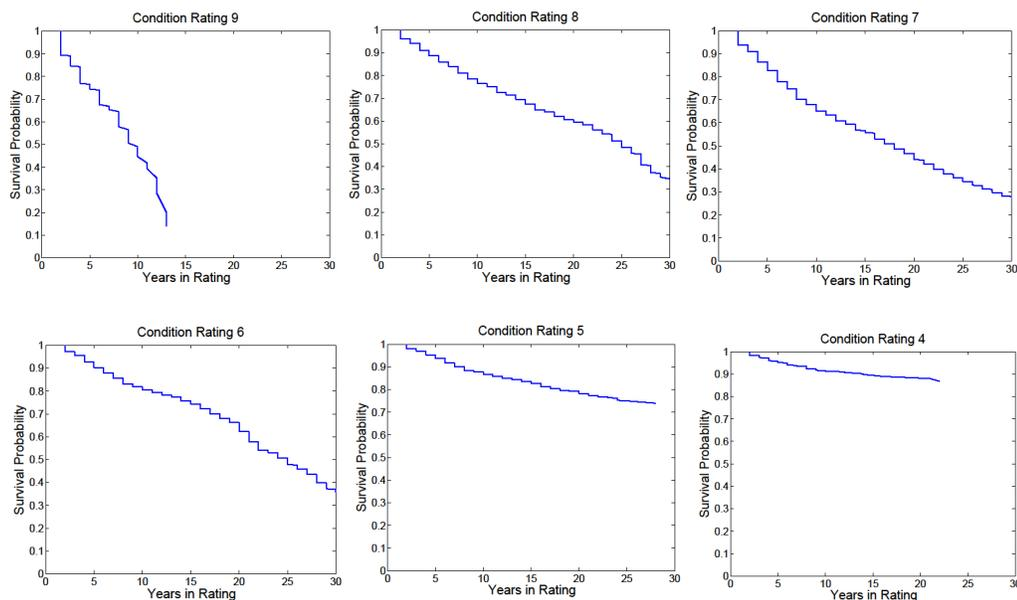
FIGURE 6.5: Concrete deck baseline survival functions
