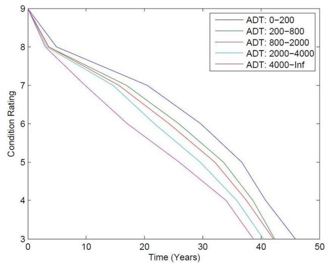
FIGURE 6.3: Steel deck deterministic deterioration models
