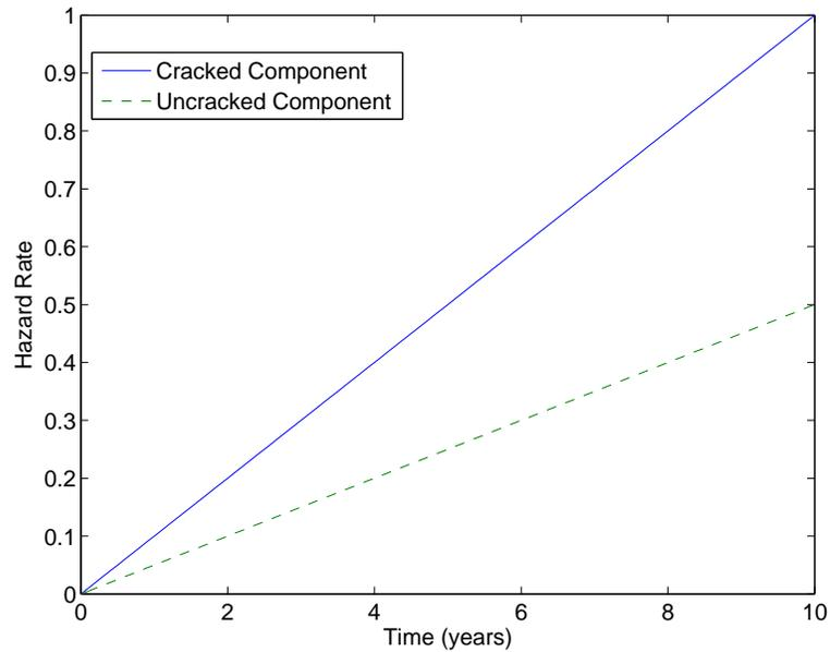
FIGURE 3.1: Hazard functions for fatigue failure of structural components
