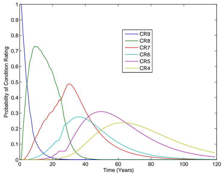
FIGURE 4.6: Condition rating probabilities for timber deck from semi-Markov process
