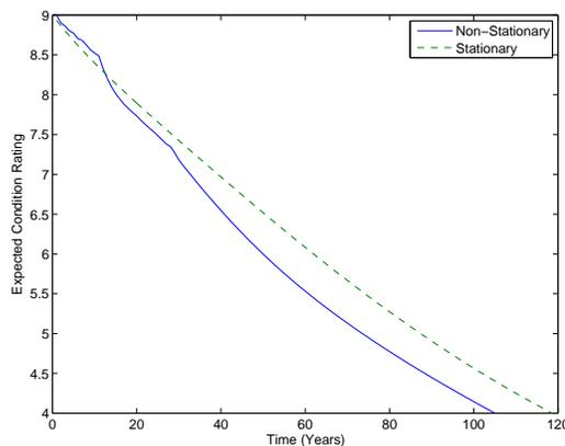
FIGURE 6.58: Steel substructure baseline prediction model
