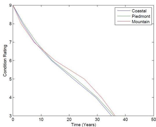
FIGURE 6.42: Timber substructure deterministic deterioration models
