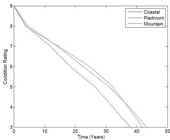
FIGURE 6.44: Steel substructure deterministic deterioration models
