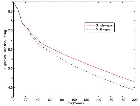
FIGURE 6.17: Effect of number of spans on concrete deck deterioration rates
