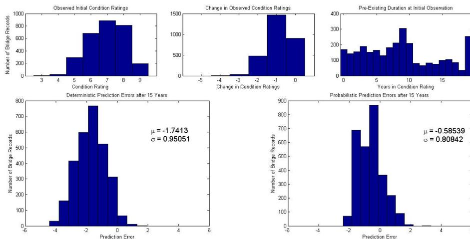
FIGURE 7.3: Histograms of concrete deck condition rating data in observation period and prediction errors
