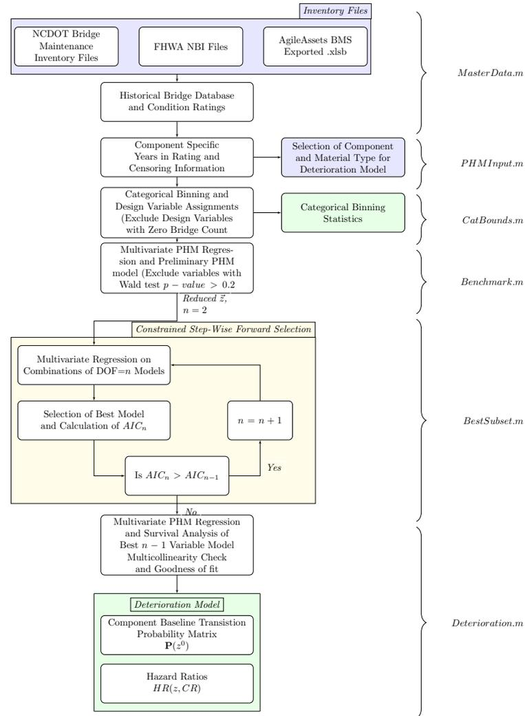
FIGURE 4.2: Proportional hazards model development flowchart
