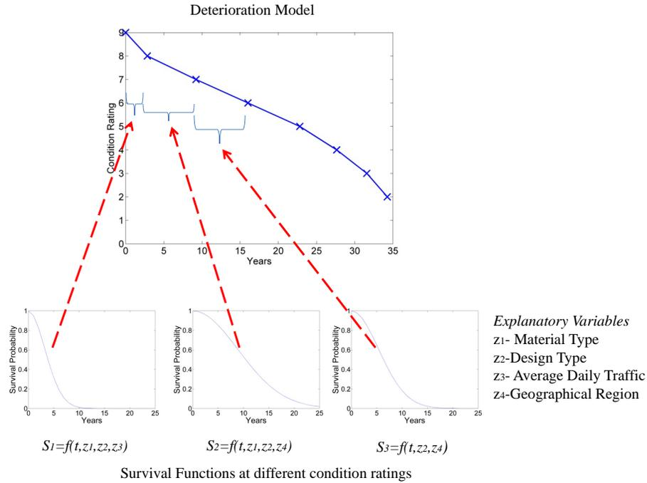
FIGURE 4.1: Deterioration model from survival analysis across individual condition ratings
