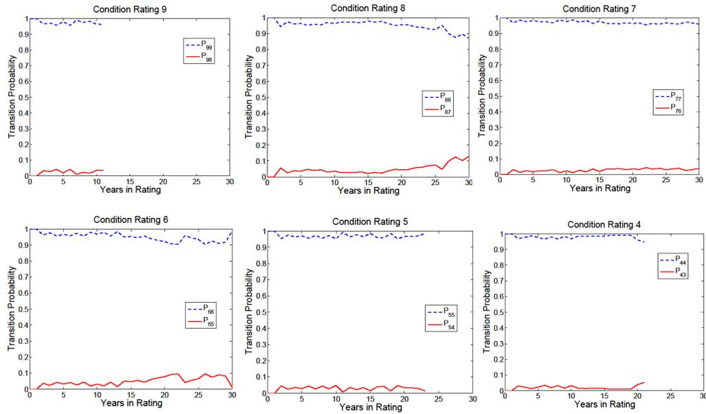
FIGURE 6.34: Steel superstructure baseline transition probabilities
