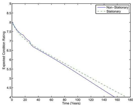
FIGURE 6.33: Concrete superstructure baseline prediction model
