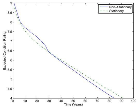
FIGURE 6.30: Timber superstructure baseline prediction model
