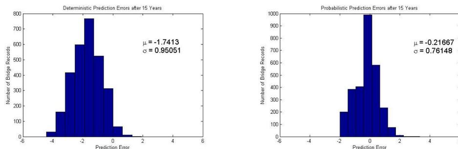
FIGURE 7.7: Histograms of concrete deck condition rating prediction errors obtained with split probability initial state vector
