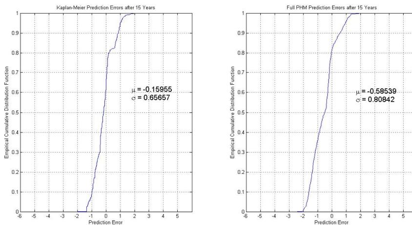
FIGURE 7.5: Empirical cumulative distribution functions associated with prediction errors of Kaplan-Meier and PHM models applied to concrete deck condition rating data
