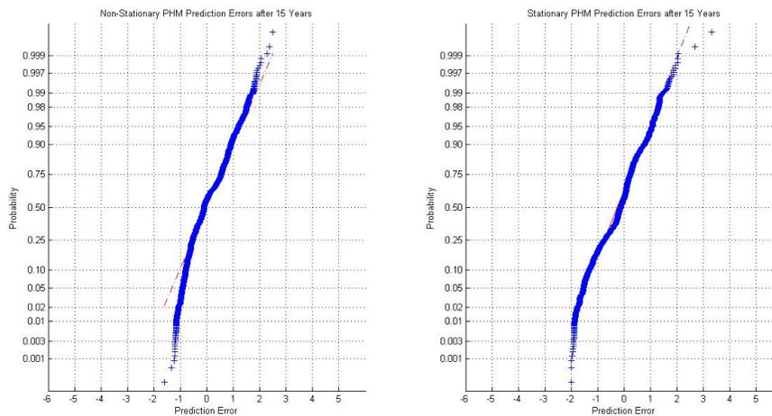
FIGURE 7.11: Normal probability plots associated with prediction errors of non-stationary and stationary PHM models applied to concrete deck condition rating data
