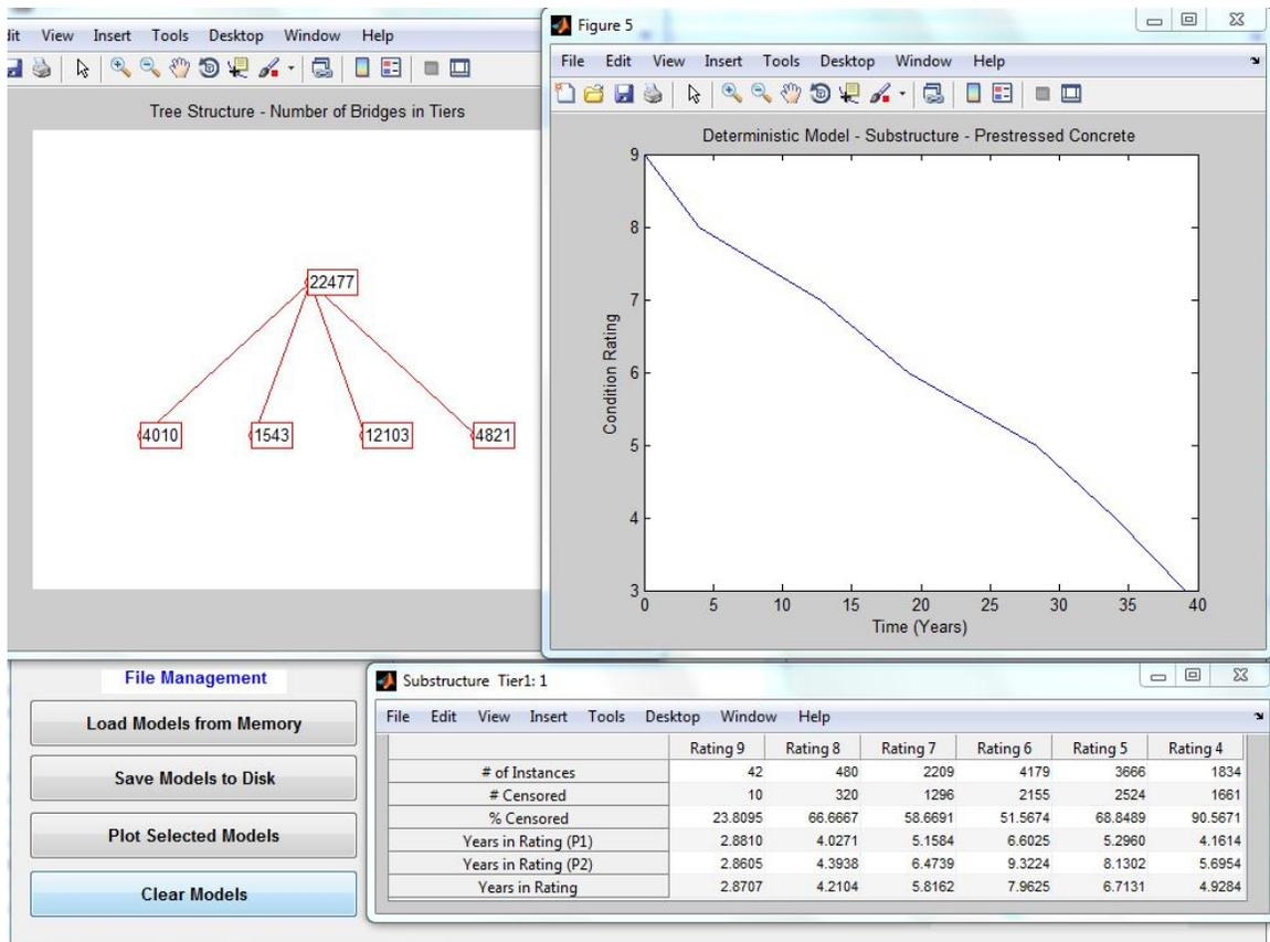
FIGURE 5.3: Representative output from deterministic deterioration modeling functions
