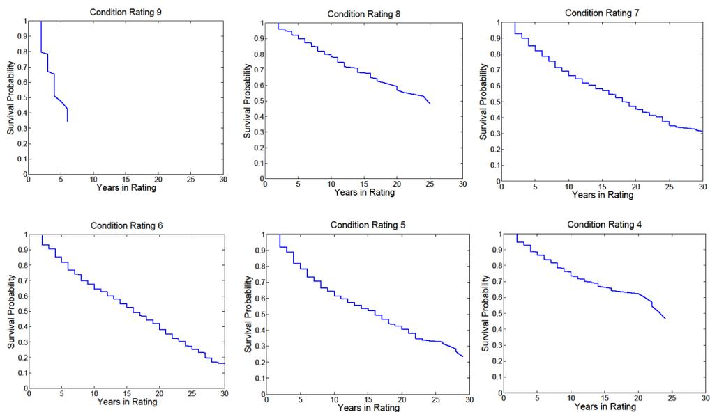
FIGURE 6.46: Timber substructure baseline survival functions
