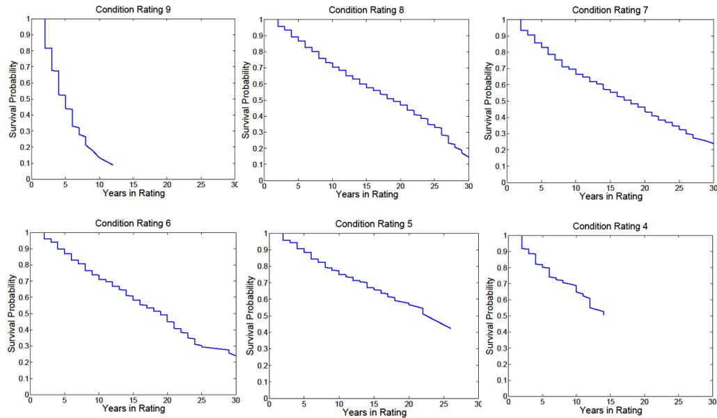
FIGURE 4.3: Baseline survival functions for timber deck across condition ratings 9 through 4
