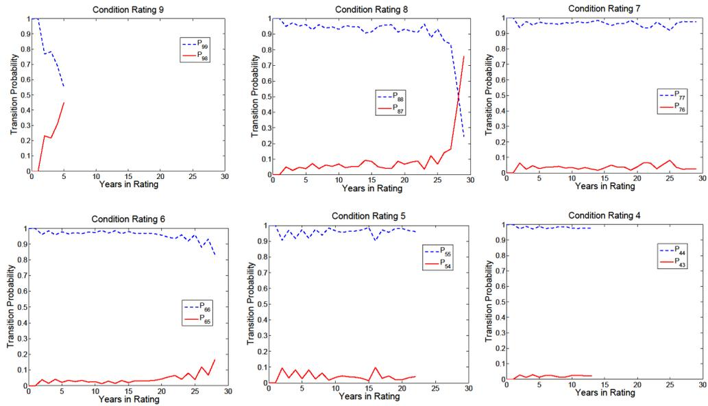
FIGURE 6.28: Timber superstructure baseline transition probabilities
