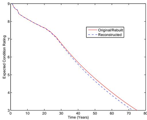
FIGURE 6.18: Effect of reconstruction on steel deck deterioration rates
