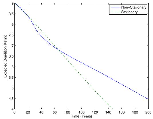
FIGURE 6.36: Steel superstructure baseline prediction model
