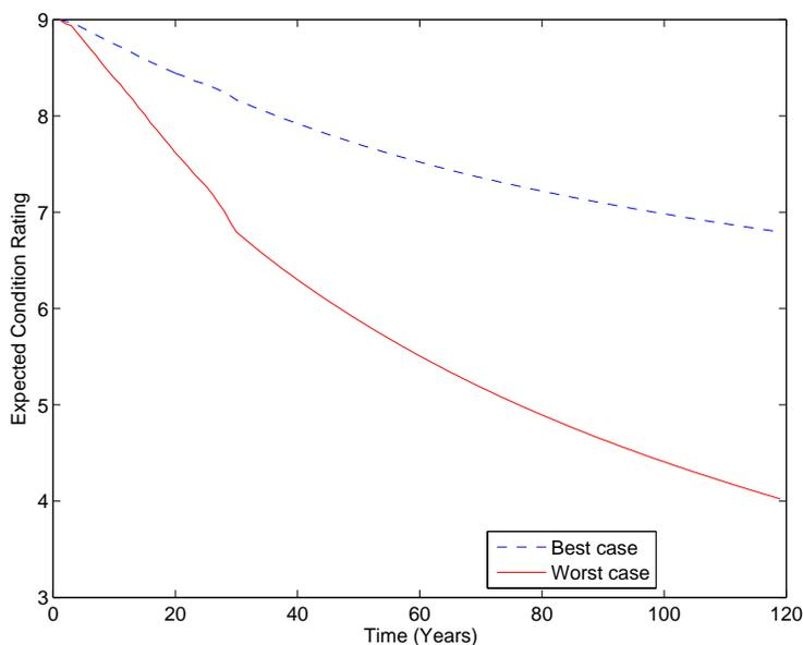
FIGURE 6.63: Concrete substructure forecast models for best case (State System 1, original/rebuilt, Piedmont/Mountain region, ADT  $\geq 1100$ , ADTT19 – 514, max span < 4m, single span, age < 15 years) and worst case (State System 2, reconstructed, Coastal region, ADT < 289, ADTT  $\geq 514$ , max span  $\geq 5$ m, multi span, age  $\geq 39$  years) combination of covariates
