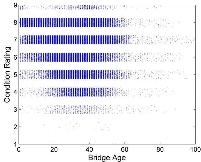
FIGURE 1.1: Deck condition ratings plotted against bridge age for all timber deck bridges in the 1981-2013 NCDOT bridge records
