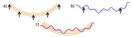
Figure 1-2: Cylindrical shell a) design condition CAD model, b) measurement data, and c) evaluation of profile deviation
