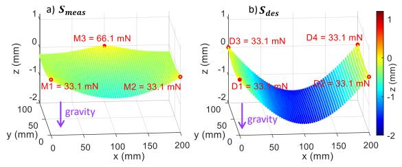
Figure 6-3: Defect-free flat plate under the influence of gravity in the a) *measurement condition* and b) *design condition*. Reaction forces represent predicted forces in the fixtures when supporting the nominal defect free part.
