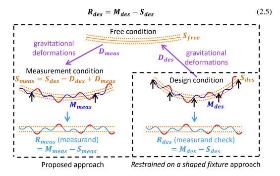
Figure 2-4: Parallel execution of the proposed approach and the *restrained on a shaped fixture* approach
