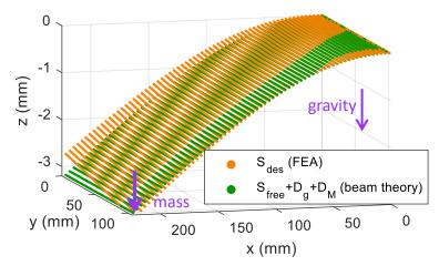
Figure 5-3: FEA versus beam theory predictions design condition
