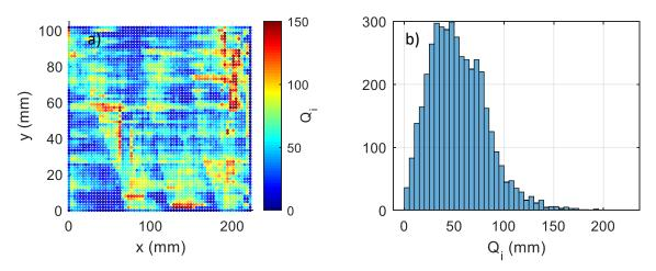
Figure 4-12: The number of nearest cloud point neighbors per node for the *measurement condition* (gravity only) represented a) graphically and b) in a histogram
