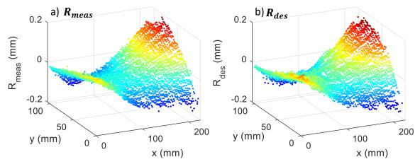
Figure 4-8: Profile deviation from a) *measurement condition* (measurand) and b) *design condition* (check of measurand)
