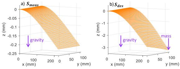
Figure 4-6: Deformed FE meshes reproduced from Figure 4-5 with different orientations and scaling
