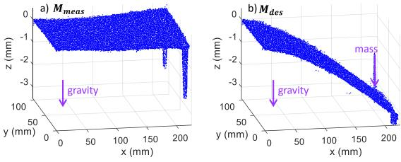
Figure 4-2: Unprocessed point clouds in a) *measurement condition* and b) *design condition*
