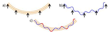
Figure 1-4: Cylindrical shell a) design condition CAD model, b) *restrained on a shaped fixture*, and c) evaluation of profile deviation
