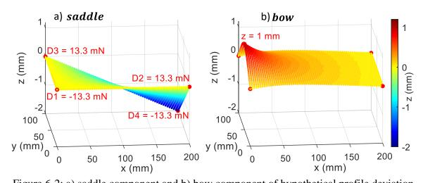
Figure 6-2: a) saddle component and b) bow component of hypothetical profile deviationIn accordance with the Figure 2-4 performance check, gravity was applied in FEAto predict the defect-free surfaces in the *measurement* and *design conditions* as shown in
