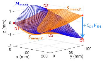
Figure 6-9: Mode shape adjusted  $S_{meas}$  to create D4 contact with  $M_{meas}$
