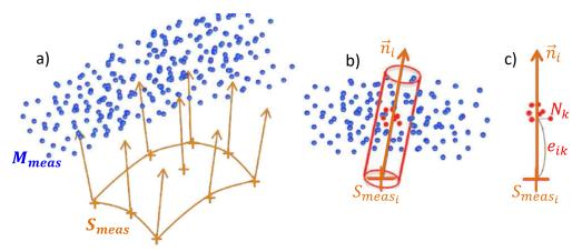
Figure 2-3: Evaluation of  $R_{meas}$  by a) registration of scan data to CAD, b) identification of nearest neighbors, and c) calculation of the profile deviation (adapted from Thiébaut et al. [34])
