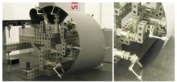
Figure 1-5: Measurement fixture for winch faring (reproduced from Ascione and Polini [4])
