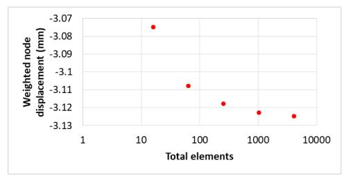
Figure 4-3: Total elements versus nodal displacement of the weighted node
