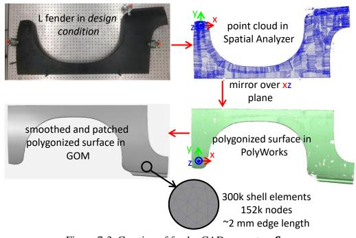
Figure 7-3: Creation of fender CAD geometry, *S*<sub>des</sub>
