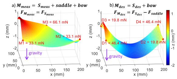
Figure 6-4: Hypothetical point clouds in the a) *measurement condition* and b) *design condition*, reaction forces represent "real" forces in the fixtures when measuring the "real" defect laden part. Quotation marks are added to "real" as a reminder that the measured point clouds with profile deviations were artificially generated.
