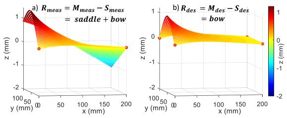
Figure 6-5: Hypothetical measured profile deviations in the a) *measurement condition* and b) *design condition*
