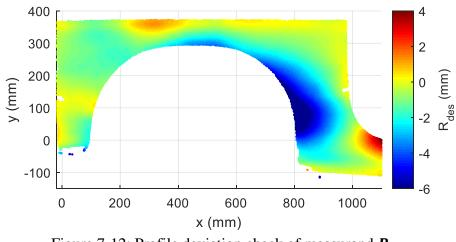
Figure 7-12: Profile deviation check of measurand  $R_{des}$
