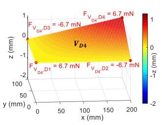
Figure 6-7: Saddle plate mode shape and reaction forces
