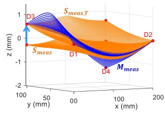
Figure 6-8: Transformation of  $S_{meas}$  to contact D3
