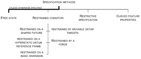
Figure 1-3: Categorization of inspection specification methods for nonrigid parts (reproduced from Abenhaim et al. [2])
