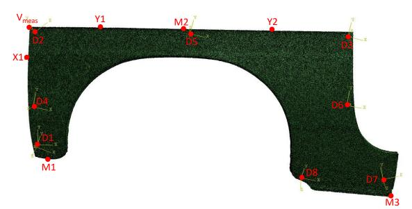
Figure 7-4: FE boundary condition nodes
