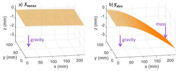
Figure 4-5: Deformed FE meshes in a) measurement condition and b) design condition
