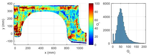
Figure 7-15: The number of nearest cloud point neighbors per node for the *measurement* condition
