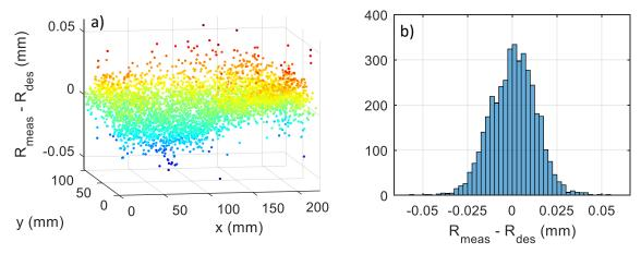
Figure 4-9: Deltas between  $R_{meas}$  (measurand) and  $R_{des}$  (check of measurand) represented a) graphically and b) in a histogram
