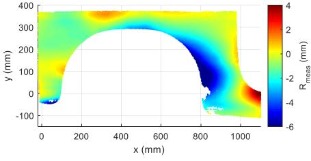
Figure 7-11: Profile deviation measurand  $R_{meas}$
