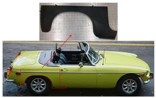
Figure 7-1: 1973 MGB rear fender section (source: sportscarshop.com/yellow-mgb/)
