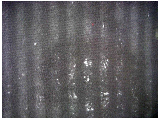
Figure 13: Fringe pattern of moiré part from first prototype. The area is approximately 1 \text{ mm}^2
