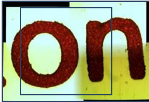
Figure 72: Object is a printed “on” letters. The region inside the box is the part that is sampled and reconstructed using transmissive compressive imaging system.
