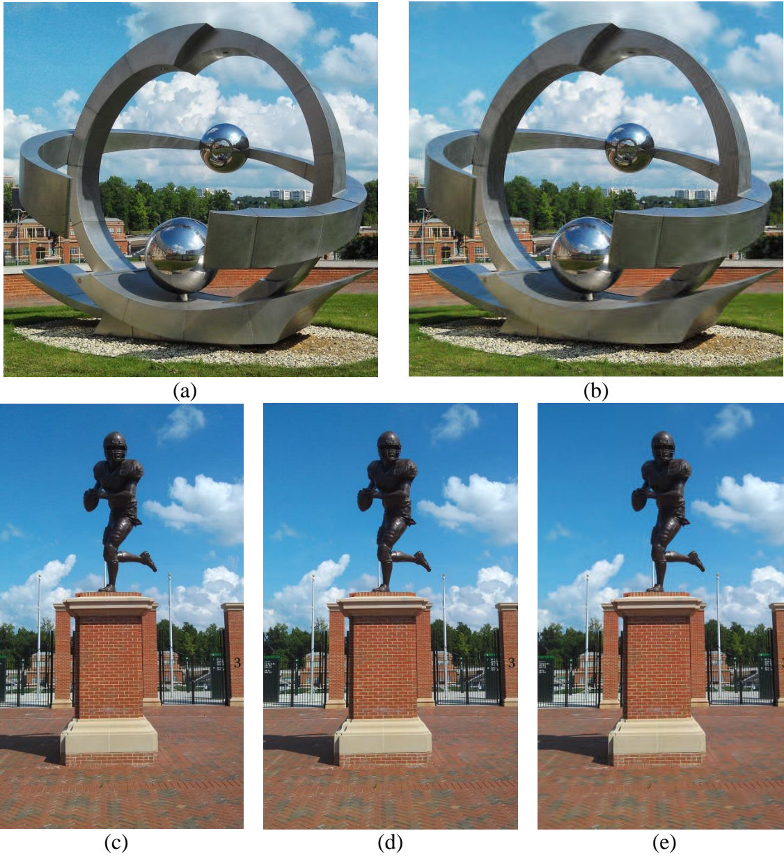
Figure 59: Image compression using wavelet packet. The original images (a) and (c) were compressed using wavelet packet tree at level 5 and Symlet wavelet of order 8. (b) is the compressed image of (a) when 99% of wavelet coefficients are set to zero; the compressed image preserves about 99% of energy. (d) is the compressed image of (c) when 96% of wavelet coefficients are set to zero; the remaining coefficients keep 99.86% of original image energy. (e) is the compressed image of (c) when 99.43% of coefficients are set to zero; the nonzero coefficients retain 99.43% of original image energy.
