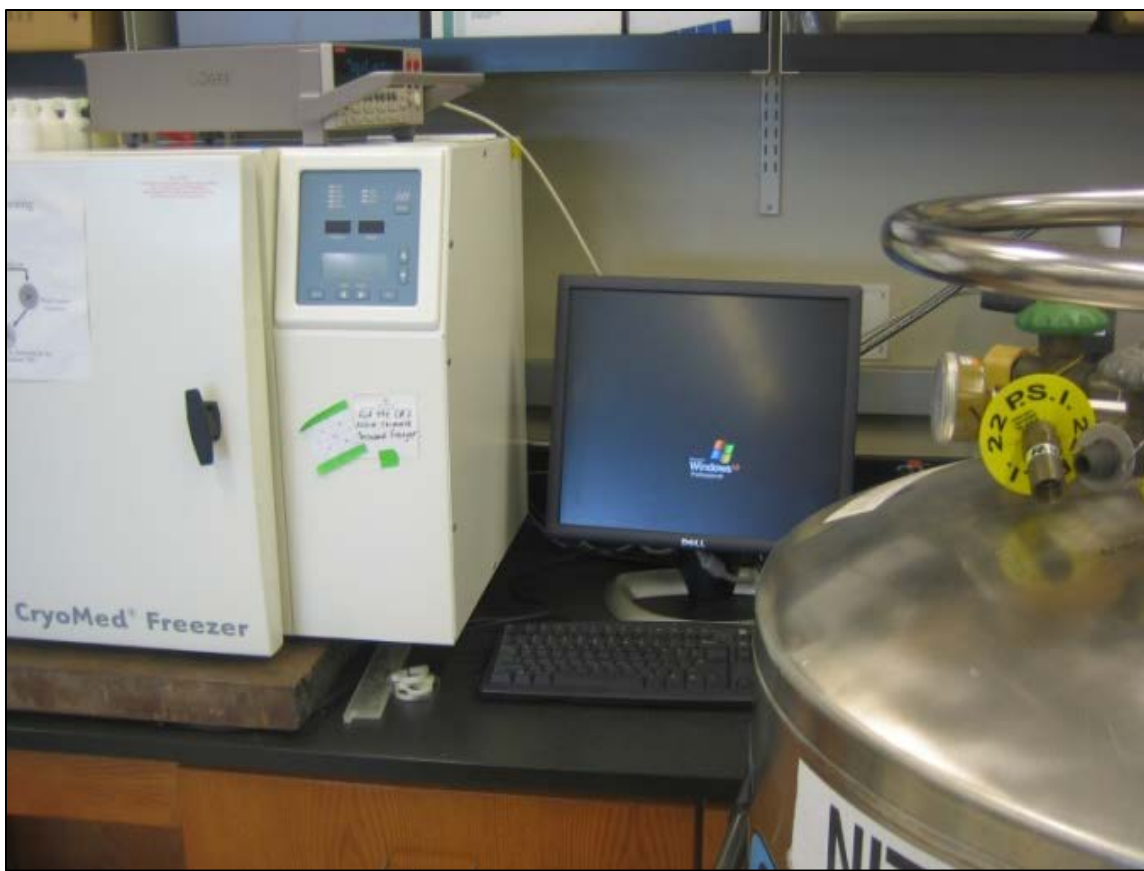
FIGURE 4.1: Equipment used for the controlled freezing of the samples. Shows the CryoMed Control Rate Freezer connected to the liquid nitrogen tank and the computer used to program and operate the freezer.
