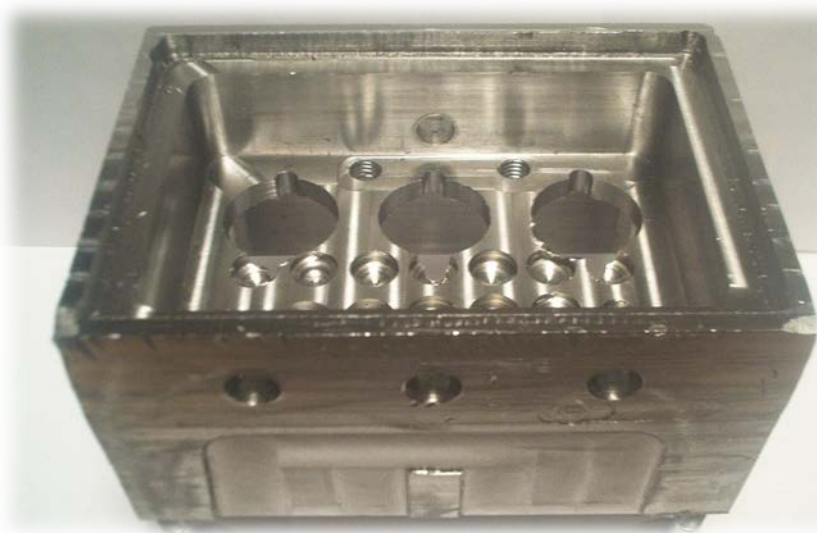
FIGURE 2.3: The experimental test device fabricated from a steel block based used to perform the benchmarking experiments † .
