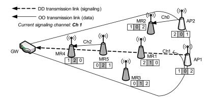
Figure 5.6: Working principles of the proposed MAC design.
