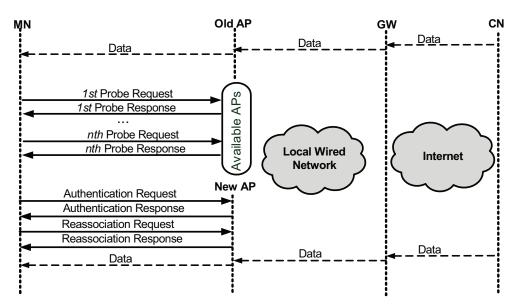
Figure 1.5: Handoff procedures in WLANs.
