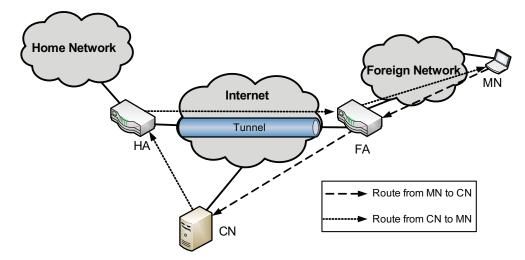
Figure 1.2: Triangular routing in Mobile IP.
