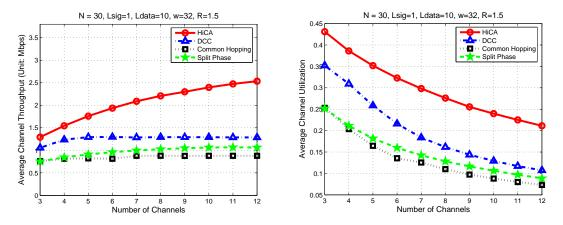
(a) Average channel throughput vs. number of channels (b) Average channel utilization vs. number of channels Figure 6.17: Channel reservation bottleneck scenario.
