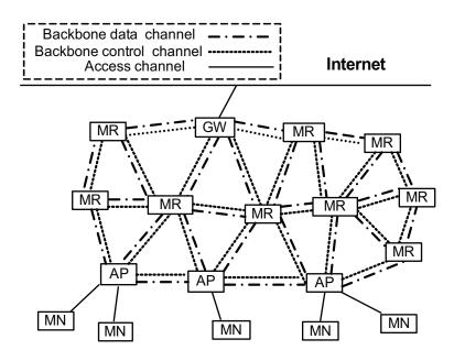
Figure 4.2: WMN architecture based on split channels.
