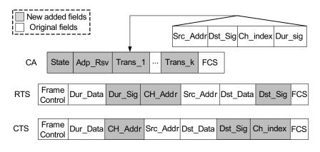
Figure 6.4: The CA frame and modified RTS/CTS frames.
