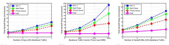
(a) Handoff delay vs. number of hops (b) Handoff delay vs. traffic volume (c) Handoff delay vs. number of MNs Figure 5.10: Handoff performance evaluation.
