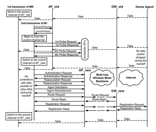
Figure 4.4: Proposed handoff procedures when an MN has two radios.
