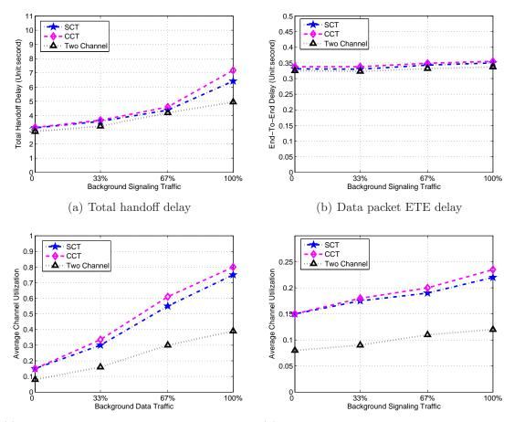
(c) Channel utilization under background *data* (d) Channel utilization under background *sig*traffic *naling* traffic
