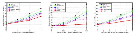
(a) Handoff delay vs. number of hops (b) Handoff delay vs. traffic volume (c) Handoff delay vs. number of MNs Figure 6.16: Total handoff delay.
