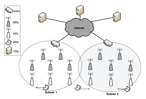
Figure 1.1: Architecture of infrastructure wireless mesh networks.
