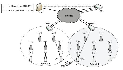
Figure 1.6: An inter-gateway handoff in wireless mesh networks.
