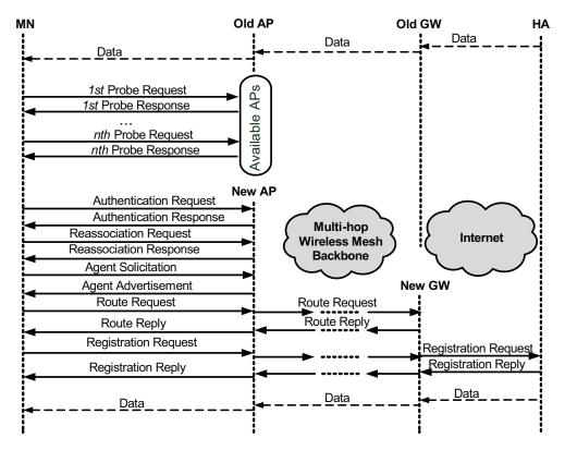
Figure 1.7: Inter-gateway handoff procedures in wireless mesh networks.
