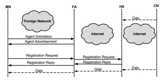
Figure 1.3: Handoff procedures in Mobile IP.
