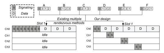
Figure 5.5: Temporary data transmission bottleneck scenario.
