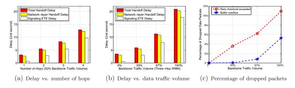
Figure 1.8: Handoff delay in 802.11-based WMNs.
