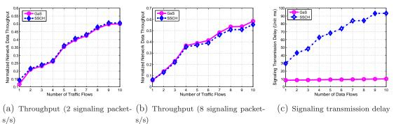
Figure 5.9: Data throughput and signaling transmission delay.
