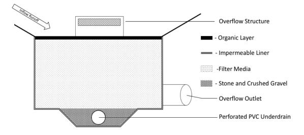
Figure 1: Charlotte, NC rain garden design adapted from the Charlotte Mecklenburg BMP design manual. Note Bruns Academy's overflow structure is an overflow spillway (Charlotte-Mecklenburg Storm Water Services, 2014).
