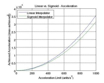
Figure 2.13: Achieved acceleration. The upper blue curve is the Linear Interpolator and the lower green curve is the E/S interpolator.
