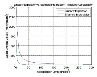
Figure 2.12: Tracking error comparison. The upper blue curve is the Linear Interpolator and the lower green curve is the E/S interpolator.
