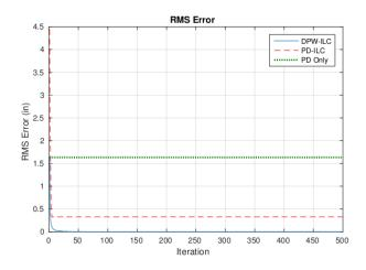
Figure 4.9: Comparison of RMS error values for DPW-ILC, PD-ILC, and PID Controls for Thermal Expansion Example
