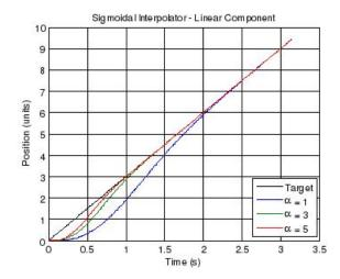
Figure 2.3: Exponential Startup for a Linear Move. As  $\alpha$  increases from 1 to 5, the exponential function more closely approximates the targeted linear move.
