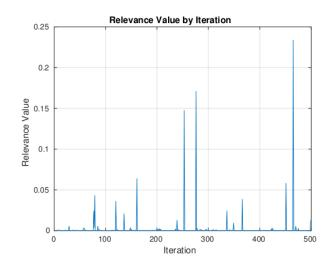
Figure 4.5: The final Relevance Index for the last iteration of 500 for Thermal Resistance example (i.e., the graph shows all of the elements of  $N_{500}$ ). The handful of indices with high relevance values share a disturbance (temperature) that is similar to the measured temperature at iteration 500 and exhibit good tracking performance.
