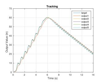
Figure 4.2: Thermal Resistance DPW-ILC example - Tracking. Only the initial PD iteration is high enough in error to be seen. All other iterations are very close to the target.
