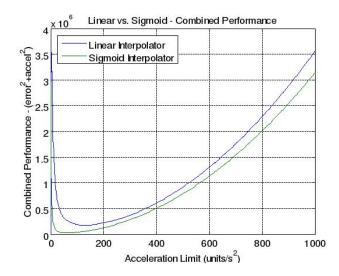
Figure 2.14: Combined tracking error and acceleration performance indices for both interpolators.
