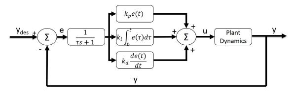
Figure 3.1: PID control system block diagram.
