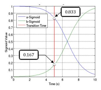
Figure 2.6: Corrected Sigmoid values at transition. The blue curve is the interpolated value of the incoming segment, and the green curve is the outgoing one.
