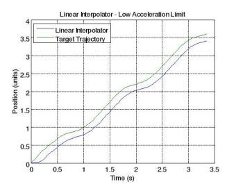
Figure 2.8: Low acceleration limit - Linear Interpolator.
