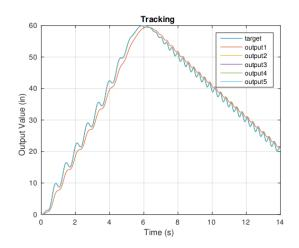
Figure 4.7: Tracking of DPW-ILC algorithm for Thermal Expansion example.
