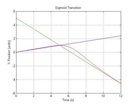
Figure 2.7: Sigmoid transition at t = 5, from a 1:5 slope to a -1:1 slope. Note that the sigmoid curve does not exceed the intersection of the two lines.
