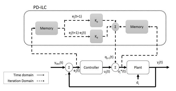
Figure 3.4: PD-ILC system block diagram.
