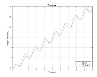
Figure 3.2: PID control of an exponentially growing ramped sinusoid MTP trajectory.
