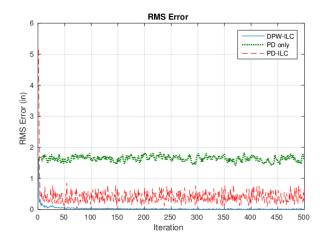
Figure 4.6: Comparison of RMS error values for DPW-ILC, PD-ILC, and PID Controls for Thermal Resistance Example.
