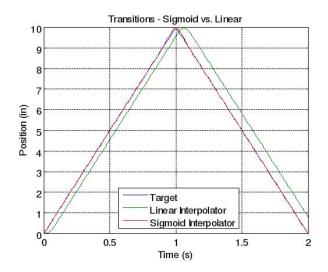
Figure 2.16: Interpolator comparison at transition.
