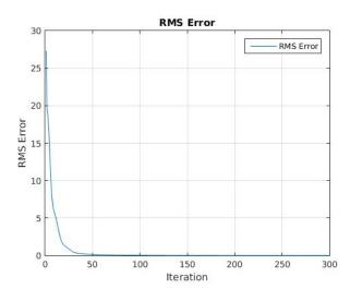
Figure 3.5: A typical application of PD-ILC over 500 iterations with zero/constant disturbance.
