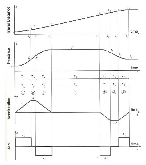
Figure 2.1: Profile of Altintas's Jerk-Limited Linear Interpolation Strategy [4].
