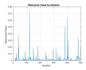
Figure 4.8: The final Relevance Index for the last iteration (500) for the thermal expansion example (i.e., the graph shows all of the elements of  $N_{500}$ ). Similar to the first example, this last run has some high relevance values, which are iterations that have both close proximity to the current measured disturbance and a low error and error rate.
