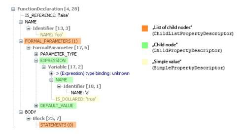
Figure 12: AST illustration of a function declaration in Eclipse PDT [24].
