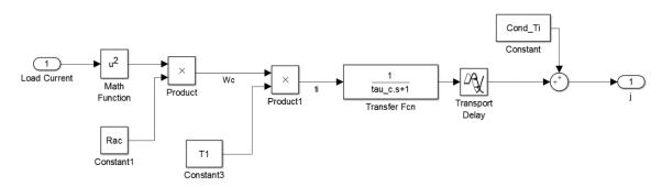
Figure 21: Jacket temperature model with current as input
