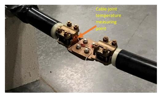
Figure 13: Cable joint temperature measurement
