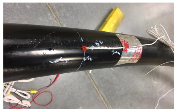
Figure 10: Conductor thermocouple installation
