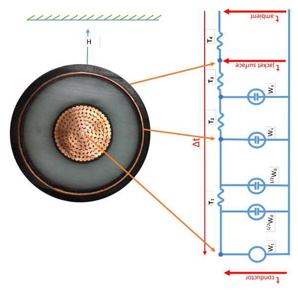
Figure 3: Extruded underground Cable Thermal to Electrical equivalent circuit
