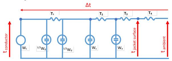
Figure 4: Extruded underground cable electrical equivalent circuit
