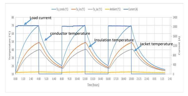
5.6.2. Cable temperature profile @ 2030A pulse load current
