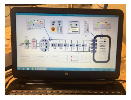
Figure 14: Load cycle heat test operator screen
