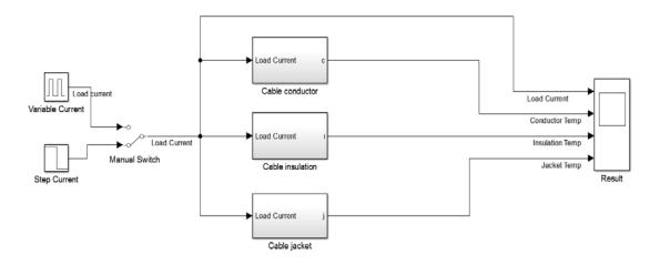
Figure 22: XLPE Cable model with current as input
