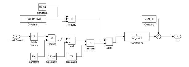
Figure 19: Conductor temperature model with current as input
