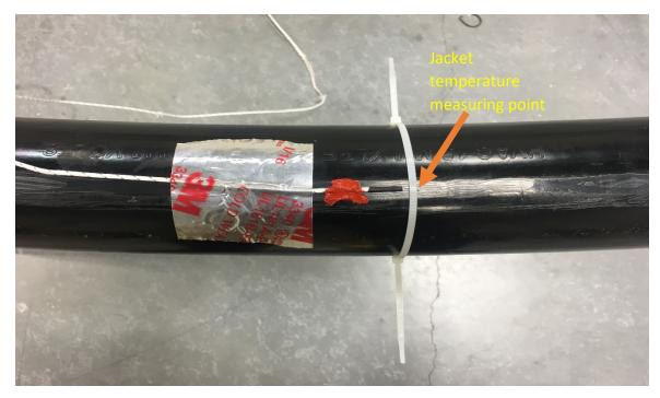
Figure 11: Jacket thermocouple installation
