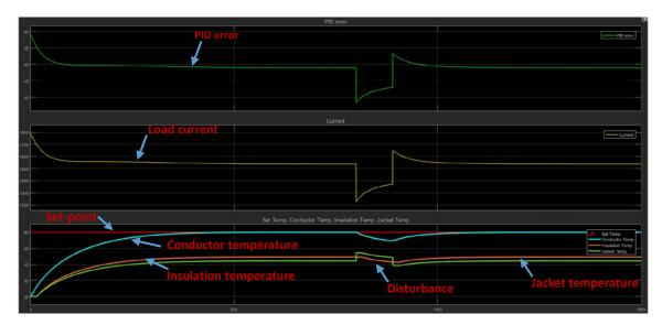
Figure 27: 60-degree desired conductor temperature response with PID control and disturbance verification.
