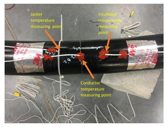
Figure 12: Complete Thermocouple installation location A
