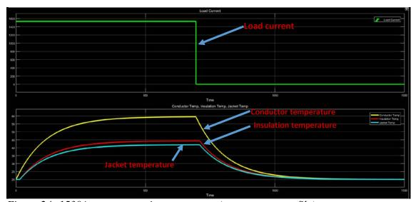
*Figure 24: 1530A current step input response (temperature profile)*
