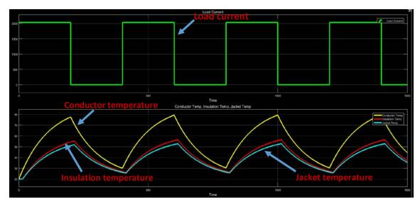
Figure 25: 2030A Pulse current input response
