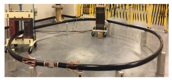
Figure 5: Sample cable looped as secondary
