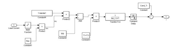
Figure 20: Insulation temperature model with current as input
