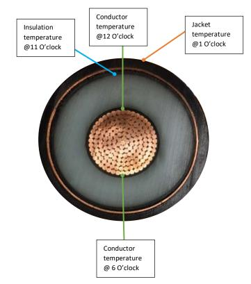
Figure 9: Cross-section A-A; Thermocouples installation positions
