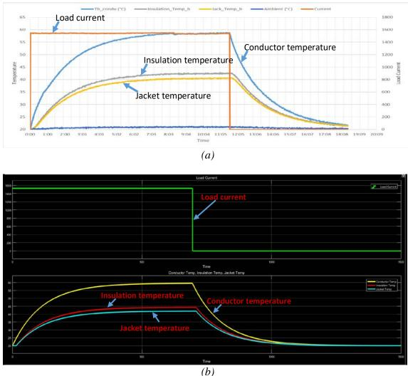
Figure 28: Cable temperature profile @ 1530A step-load current; (a) Measured *result;(b) Model result*
