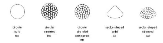
Figure 2: (b) Conductor construction
