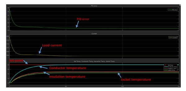
Figure 26: 60-degree desired conductor temperature response with PID control
