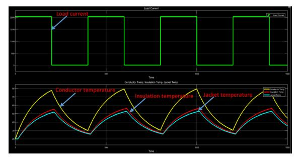
*Figure 29: Cable temperature profile @ 2030A step load current; (a) Measured result;(b) Model result*
