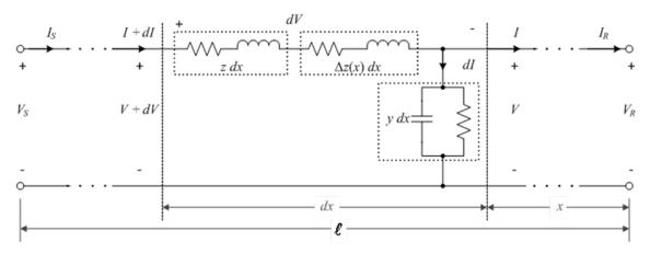
FIGURE 3.1:Non-uniform distributed line model [20]
