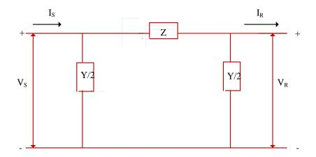
FIGURE 2.2 : Lumped type- nominal transmission( $\pi$ ) line model with V<sub>S</sub>,V<sub>R</sub>,I<sub>S</sub>,I<sub>R</sub>,Z,Y/2 being sending, receiving end voltage, sending end current ,receiving end current , impedance, admittance respectively [15]
