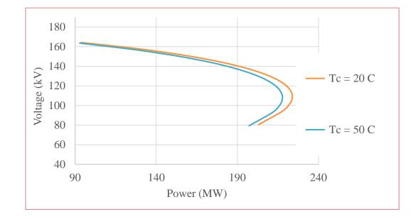
FIGURE 5.1: PV (voltage (kV) v/s power (MW)) curves for two conductor temperatures (T<sub>C</sub>=20 and 50 °C)
