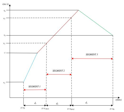
FIGURE 4.9: Wind profile v(x) v/s Position(x) plotted along the line based on wind speed measurements obtained along length of transmission line.
