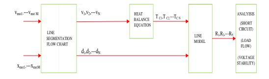
FIGURE 4.6: Proposed modeling approach with wind speed measurement inputs: measurement value ( $v_{mst1}, v_{mst2}, \ldots, v_{mstM}$ ) and measurement location ( $x_{mst1}, x_{mst2}, \ldots, x_{mstM}$ ), resulting line model segmentation: segment lengths and conductor temperatures ( $d_1, d_2, \ldots, d_N, T_{C1}, T_{C2}, \ldots, T_{CN}$ ), and resulting resistance of each segment ( $R_1, R_2, \ldots, R_N$ ).
