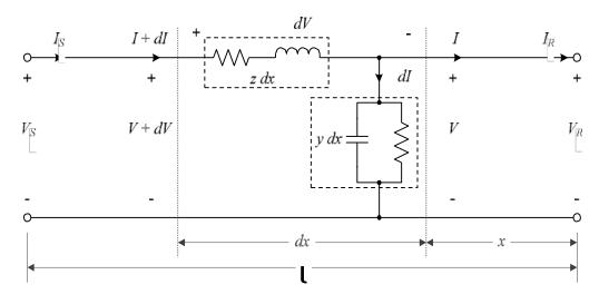
FIGURE 2.1: Uniform distributed parameter line model [22]
