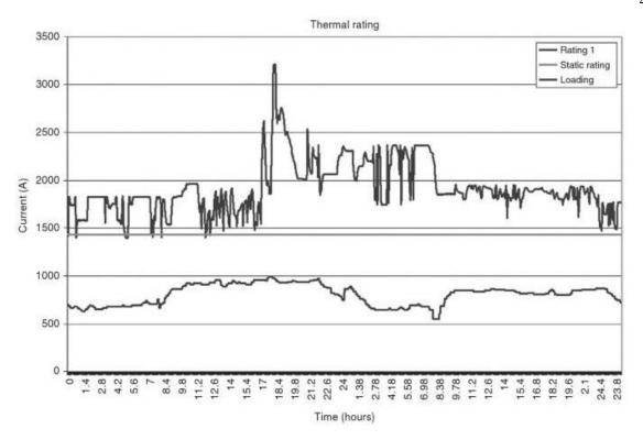
FIGURE 1.1: Dynamic thermal rating profile of a transmission line in Malaysia [14] The figure 1.1 indicate the static line rating and dynamic line ratings for specific load variations.
