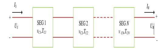
FIGURE 4.1: Block diagram of *N*-segment line model with each line segment at a corresponding wind speed ( $v_{C1}$ ,  $v_{C2}$  ---- $v_{CN}$ ) in m/s and corresponding conductor temperatures( $T_{C1}$ ,  $T_{C2}$ ---- $T_{CN}$ ) in degrees Celsius (°C) and  $I_{S}$ ,  $I_R$ ,  $U_S$ ,  $U_R$  being sending end current, receiving end current, sending end voltage and receiving end voltage respectively
