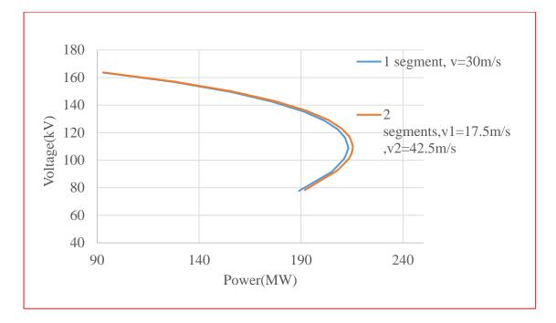
FIGURE 5.9: PV curves for line segments operated at their average wind speeds
