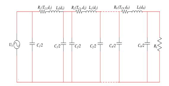
FIGURE 4.3: N-segment line model with each line segment modeled at a specific wind speed ( $v_{C1}$ ,  $v_{C2}$ , ...,  $v_{CN}$ ), each segment resistance is dependent on corresponding conductor temperature ( $R(T_{C1})$ ,  $R(T_{C2})$ , ...,  $R(T_{CN})$ ), inductance ( $L_1(d_1)$ ,  $L_2(d_2)$ , ...,  $L_N(d_N)$ ) and capacitance ( $C_1/2$ ,  $C_2/2$ , ...,  $C_N/2$ ) are independent of wind speed but depend on segment length, the load resistance is indicated by  $R_L$ .
