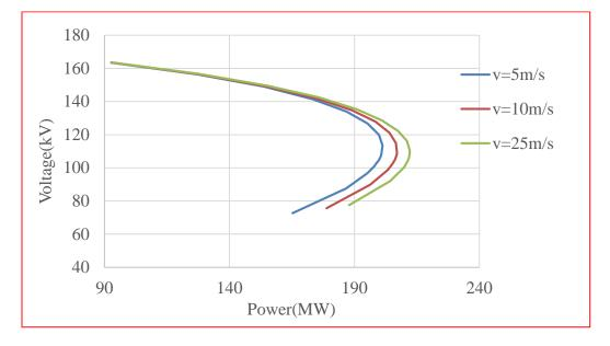
FIGURE 5.5: PV (voltage (kV) v/s power (MW)) curves for different wind speeds (v=5, 10, 25m/s)
