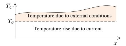
FIGURE 1.2: Example graphical representation of conductor temperature,  $T_{c}$ , vs. distance along the line, x [19]
