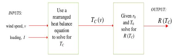
FIGURE 4.2: Proposed modeling approach with inputs (wind speed (v) in m/s, current (I) from steady state equation and ( $R_O$ ) being reference resistance,( $T_O$ ) being reference conductor temperature, with conductor temperature ( $T_C$ ), line resistance of conductor  $R(T_C)$ ) and outputs (power in (MW) and receiving end voltage ( $U_R$ )),d is the length of the line
