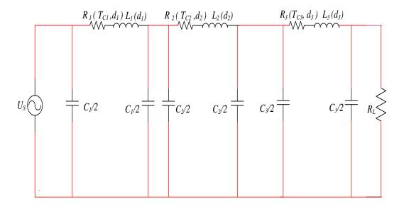
FIGURE 4.10: 3-segment line model with each line segment modeled at wind speeds ( $v_{C1}$ ,  $v_{C2}$ ,  $v_{C3}$ ) and corresponding resistances calculated at conductor temperatures  $R_1(T_{C1},d_1)$ ,  $R_2(T_{C2},d_2)$ ,  $R_3(T_C,d_3)$ , inductances ( $L_1(d_1)$ ), ( $L_2(d_2)$ ), ( $L_3(d_3)$ ), capacitances ( $C_1/2$ ,  $C_2/2$ ,  $C_3/2$ ), sending-end voltage ( $U_S$ ) and resistive load ( $R_L$ ).
