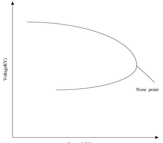
Power(MW) FIGURE 4.11: A simple PV curve with its nose point [29]
