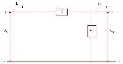
FIGURE 2.3: Lumped type- nominal transmission(τ) line model with V<sub>S</sub>,V<sub>R</sub>, I<sub>S</sub>,I<sub>R</sub>,Z,Y being sending ,receiving end voltage, sending end current, receiving end current, impedance, admittance respectively [15]
