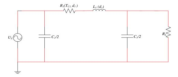
FIGURE 4.5: ( $\pi$ ) Line model with single line segment having sending end voltage(U<sub>S</sub>), resistance of line dependent on conductor temperature (T<sub>C1</sub>), with inductance (L<sub>1</sub>), capacitance divided in two halves (C<sub>1</sub>/2), (C<sub>1</sub>/2), load resistance (R<sub>L</sub>).
