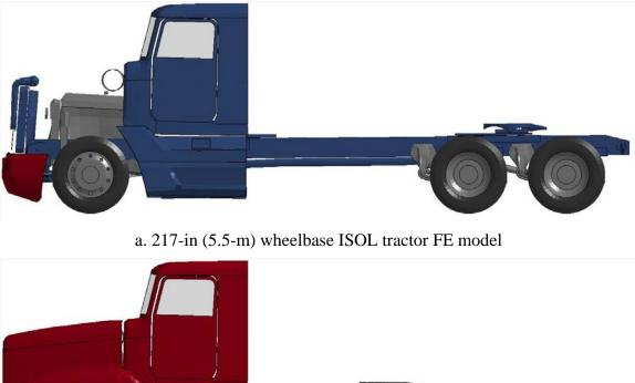
b. 154.7-in (3.9-m) wheelbase ISOL tractor FE modelFigure 3.17: ISOL tractor FE model wheelbases
