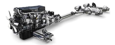
Figure 3.1: Tractor powertrain system (URL1)
