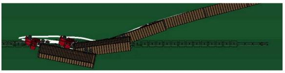
e. Case m: sloped median W-beam guardrail backside impact
