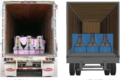
a. MwRSF full-scale test b. NTRCI FE model Figure 3.26: Ballast load configuration
