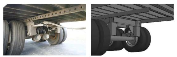
a. NTRCI purchased trailer b. FE model Figure 3.21: Trailer tandem bogie assembly
