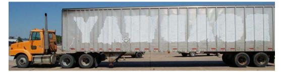
Figure 3.28: 1991 White/GMC WG64T tractor with a 1988 Pines 48-ft (14.6-m) trailer used in the MwRSF full-scale crash test
