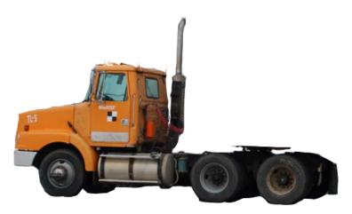
Figure 3.16: 1991 White/GMC WG64T conventional day-cab tractor used in the MwRSF full-scale crash test
