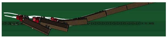
g. Case o: sloped median wood-blockout Thrie-beam guardrail backside impact
