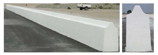
Figure 3.29: Vertical-faced concrete barrier used in the MwRSF full-scale crash test
