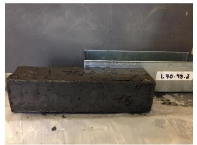
Figure: E.6 Sample 1.70.48.2 at 99 of 264 cycles.
