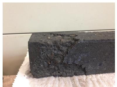
Figure: E.16 Sample 2.80.24.1 at 231 of 231 cycles.
