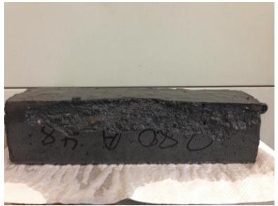
Figure: E.21 Sample 2.80.48.1 at 198 of 198 cycles.
