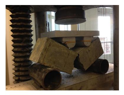
Figure: 4.14 Testing setup for modulus of rupture per ASTM C78.
