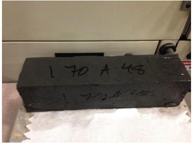
Figure: E.5 Sample 1.70.48.2 at 66 of 264 cycles.
