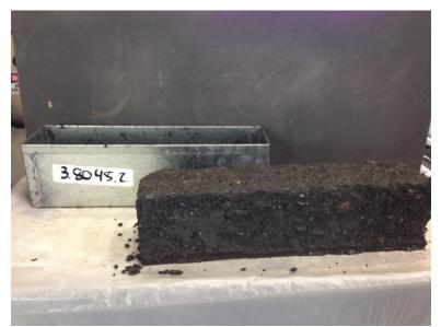
Figure: E.22 Sample 3.80.48.2 at 33 of 132 cycles.
