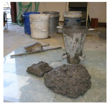
Figure: 3.1 Slump flow test setup using Procedure B of ASTM C1611.
