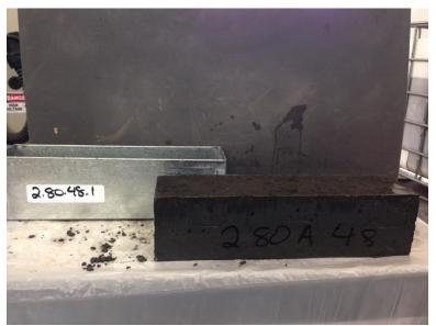
Figure: E.20 Sample 2.80.48.1 at 33 of 198 cycles.
