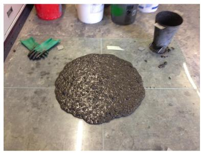
Figure: 3.2 Slump flow test sample once allowed to flow completely per ASTM C1611.
