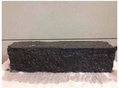
Figure: E.19 Sample 1.80.48.2 at 231 of 231 cycles.
