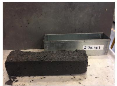
Figure: E.12 Sample 2.70.48.1 at 264 cycles, 66 cycles past the 60% of initial dynamic modulus.
