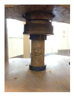
Figure: 4.4 Standard testing setup for compressive strength testing per ASTM C39.
