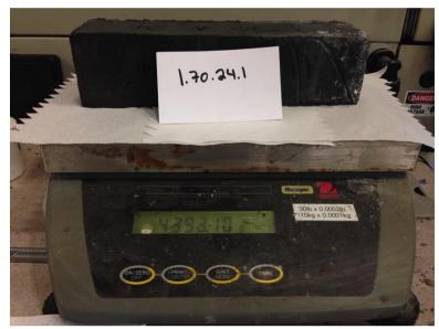
Figure: 6.8 Sample weight measurement following removal from environmental chamber.
