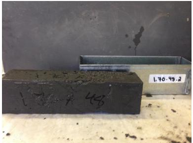
Figure: E.7 Sample 1.70.48.2 at 198 of 264 cycles.
