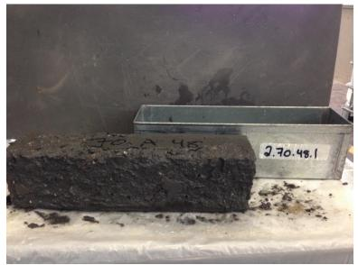
Figure: E.10 Sample 2.70.48.1 at 165 of 198 cycles.
