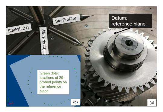
Figure 6.3: Measurement of datum features on the gear artifact using 8-star-probe: (a), measurement of datum reference plane; (b), locations of the probed points.
