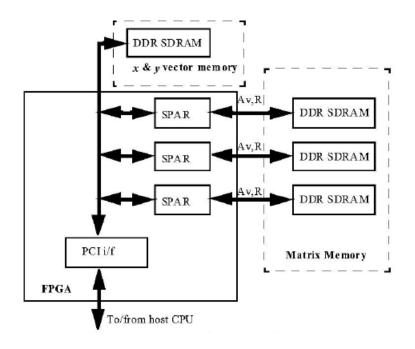
Figure 4.24: Version 2.0: SpMV reduction hardware [7]
