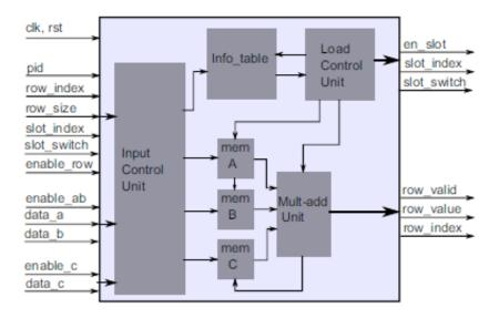
Figure 4.25: Version 3.0: SpMV multiply hardware [8]
