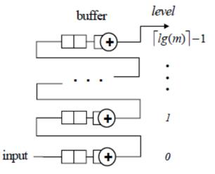
Figure 4.22: Version 1.0: SpMV reduction hardware [6]
