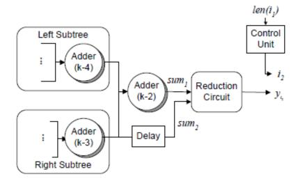
Figure 4.21: Version 1.0: SpMV multiply hardware [6]
