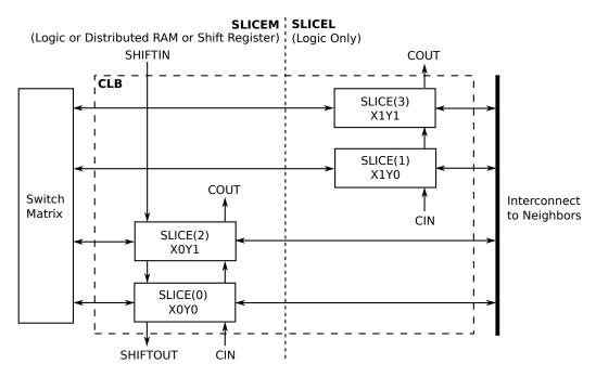
Figure 2.1: Configurable logic blocks and slices of a Virtex 4 FPGA
