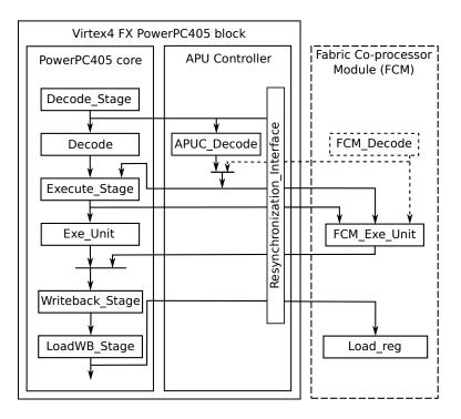
Figure 2.2: PPC, APU, and FCM interaction
