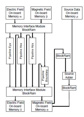
Figure 4.16: Version 2.0: 2D-FDTD overall hardware design [4]
