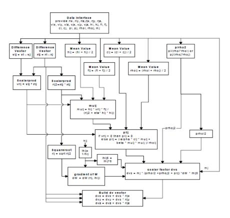
Figure 4.34: N-body hardware design [14]
