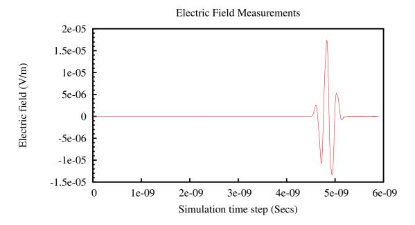
Figure 5.11: Electric field at receiver port for 2D-FDTD GFHD PEC Model
