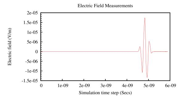
Figure 5.6: Electric field at receiver for 2D-FDTD LFHD PEC Model
