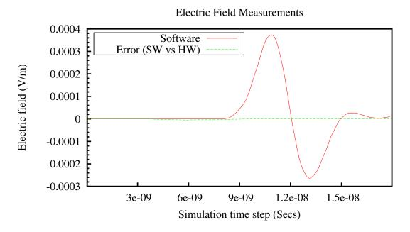
Figure 5.8: Electric field at receiver port for 2D-FDTD Mur Model
