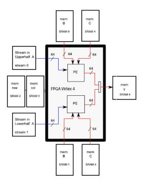
Figure 4.26: Version 3.0: SpMV overall hardware [8]
