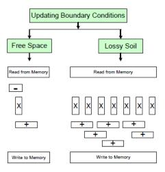
Figure 4.15: Version 2.0: 2D-FDTD boundary updating hardware design [4]
