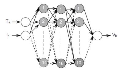
Figure 4.6: Version 2.0: P-V battery charging NN model [2]
