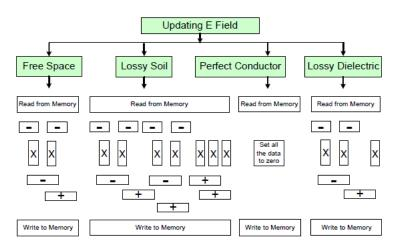
Figure 4.13: Version 2.0: 2D-FDTD 'E' field updating hardware design [4]
