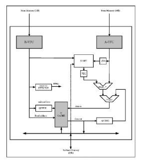
Figure 4.23: Version 2.0: SpMV multiply hardware [7]
