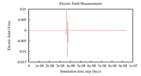
Figure 5.14: Electric field at receiver port for 2D-FDTD UMPL GFHD Model
