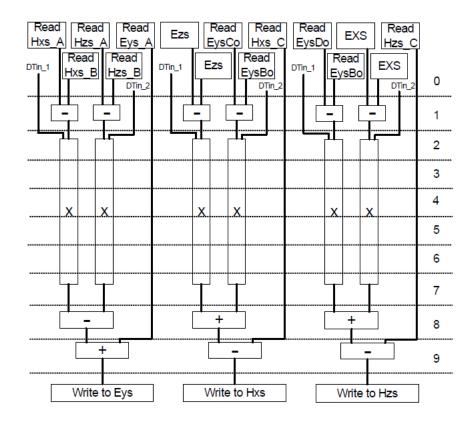
Figure 4.14: Version 2.0: 2D-FDTD 'H' field updating hardware design [4]
