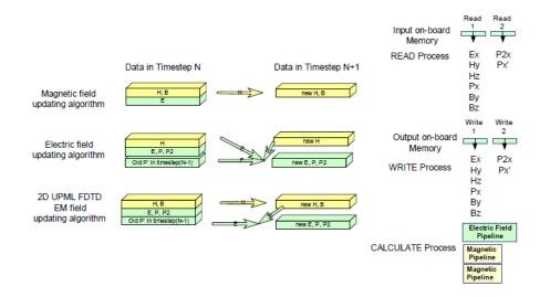
Figure 4.19: Version 3.0: 2D-FDTD UPML overall hardware design [5]
