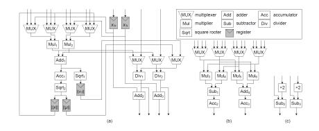
Figure 4.32: Hessenberg reduction design [12]
