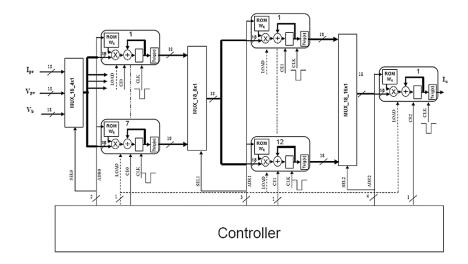
Figure 4.10: Version 2.0: P-V regulator hardware design [2]
