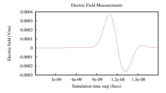
Figure 5.13: Electric field at receiver port for 2D-FDTD Mur GFHD Model
