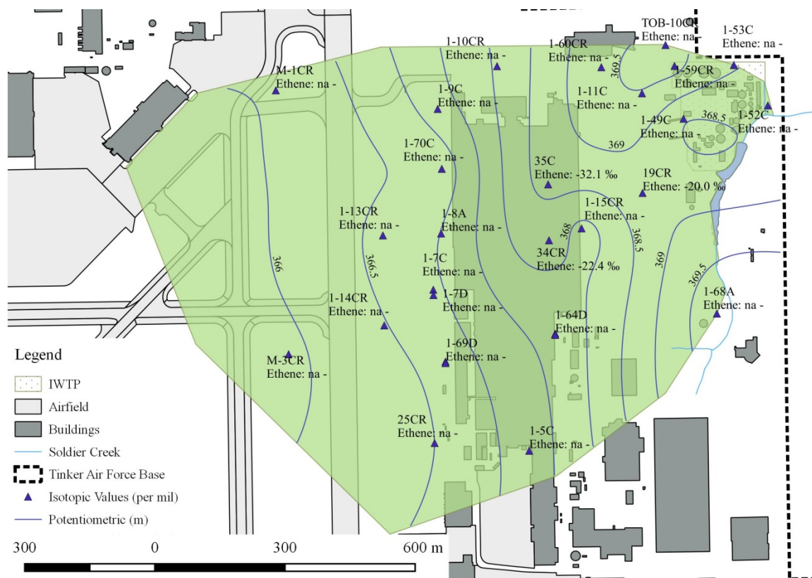
FIGURE 3-43: LLSZ potentiometric surface and ethene isotopic composition, 2008 Map illustrating groundwater potentiometric surfaces and ethene isotope results in the LLSZ within the study area.
