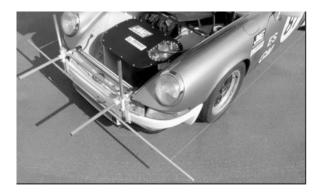
Figure 2.18: Toe alignment using strings [29].
