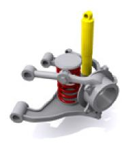
Figure 2.4: Multi-link suspension [6].
