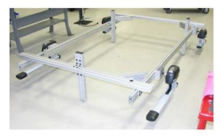
Figure 3.20: Aluminum alignment head test fixture.
