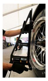
Figure 2.22: Camber measurement using camber/caster Gauge [29].
