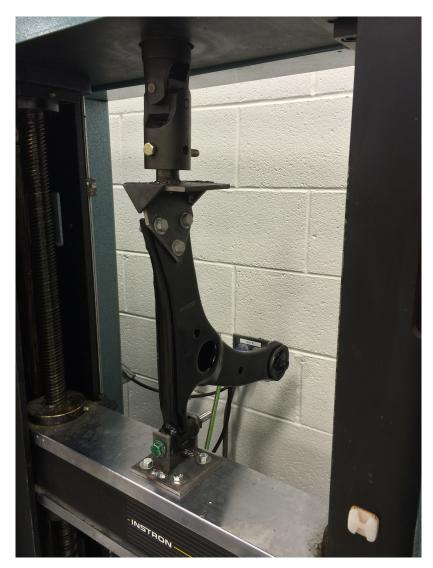
Figure 3.25: Bushing stiffness test setup.
