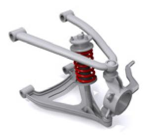
Figure 2.3: Double wishbone suspension type 1 [6].
