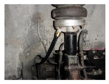
Figure 2.7: Air suspension of a Cadillac DeVille.
