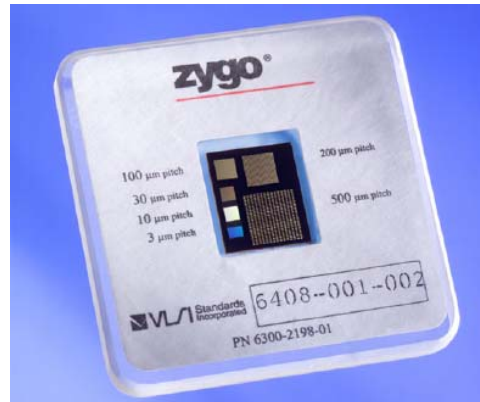
FIGURE 2.1.4: Lateral calibration standard [99].
