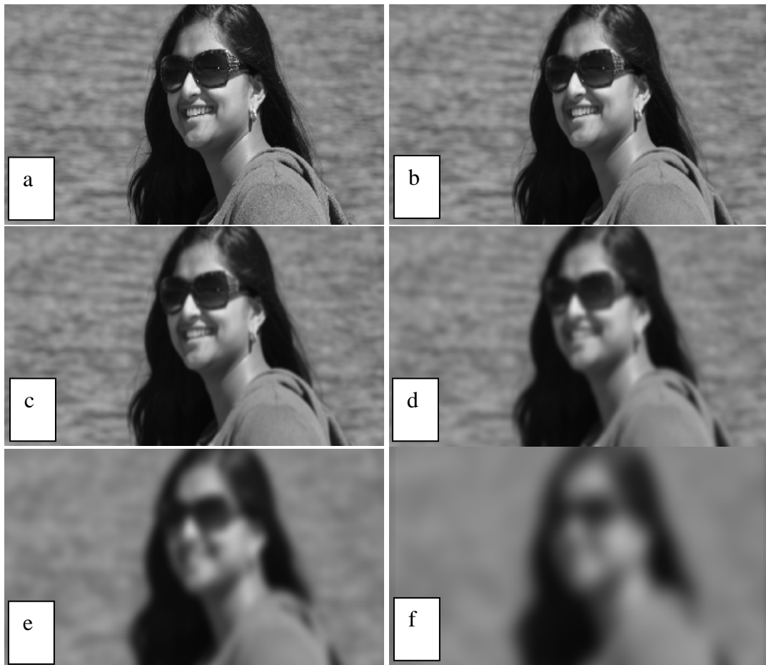
FIGURE 1.4.10: 6-level DWF based decomposition of image ‘Haritha’ using B3 spline as mother wavelet.
