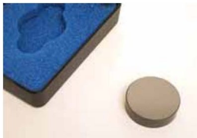
FIGURE 2.1.2: Silicon Carbide reference flat standard [97].
