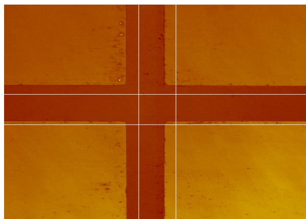
FIGURE 2.4.2: Grid plate measurement, showing variation between target and actual locations.
