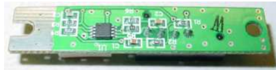
Figure 49c. The TDS PCB. A series of resistors and capacitors combined with a rail-to-rail output (RRO) dual op amp generates a measurable signal.
