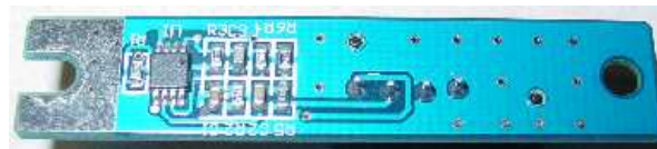
Figure 49d. The final TDS PCB. The PCB layout changed due to avoid high failure rate when IR reflow soldering. The PCB color was changed to avoid confusion with the previous version.
