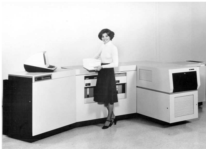
Figure 1 [2]. The Xerox laser printer model 9700 ca. 1977. The figure is a picture of one of the first laser printers manufactured.
