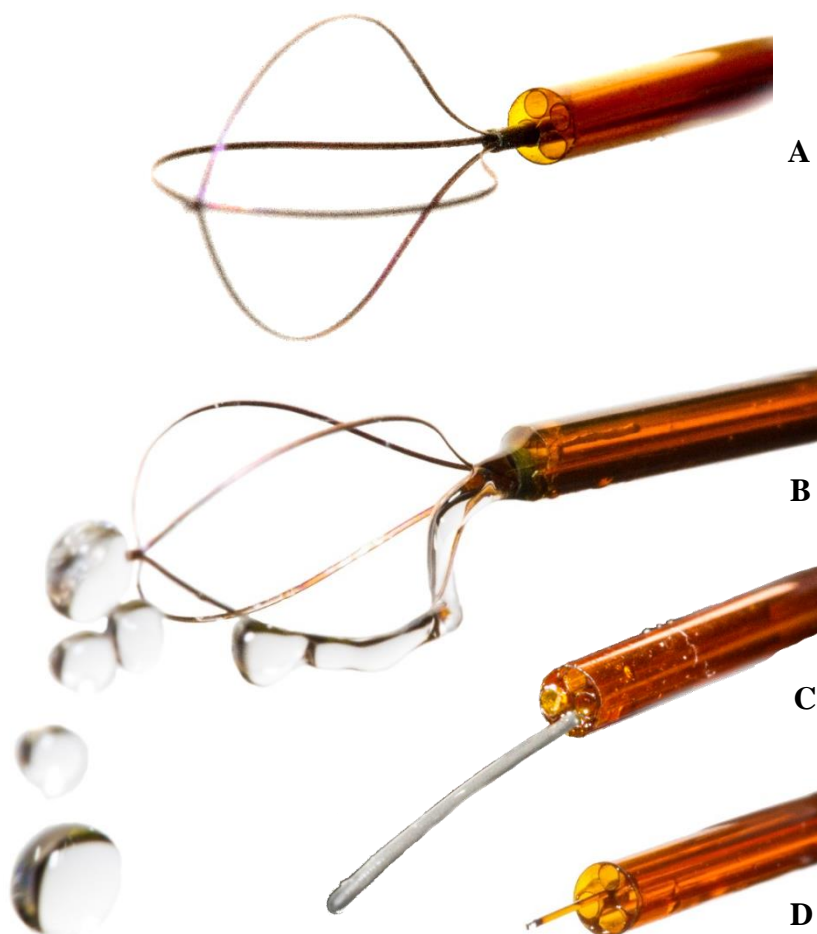
Figure 6.2: Miniaturized ureterscope tip with device demonstrations: (A) 1.3 Fr stone basket insertion (B) Stone basket insertion with saline flow (C) Guidewire insertion (D) 100- \mu\text{m} -core (170- \mu\text{m} -OD) delivery fiber insertion through central channel.
