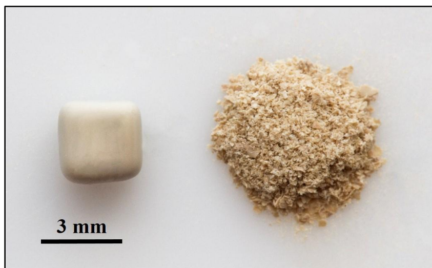
Figure 7.3: Human urinary stone with remaining stone dust from single ball tip fiber study with 3 urinary stone samples.
