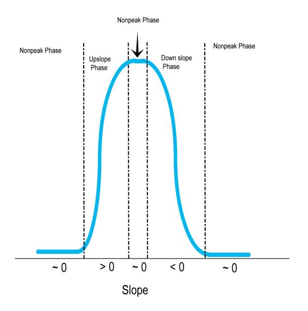
FIGURE 2.4: Example of the 4 phases of peak identification in the linear interpolation algorithm. Linear interpolation and peak calling algorithm designed and written by Dr. Anthony Fodor.
