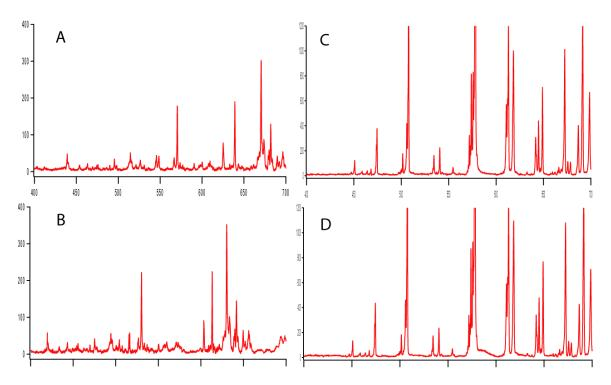
FIGURE 2.7: Zoomed in regions of electropherograms that demonstrate QC correlation Performance: A&B: Low correlating pair of technical replicates ( $r^2 = 0.04$ ) where the top spectra has shifted and been stretched relative to the lower panel producing a poor match. C&D: High correlating pair of technical replicates  $r^2 = 0.99$ ).
