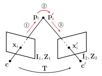
Figure 3.1: The warp function that map pixels between images through: (1) reconstruction (inverse projection with known depth), (2) transformation of the reconstructed point, and (3) projection projection of the transformed point into the other image. Figure modified from [20].
