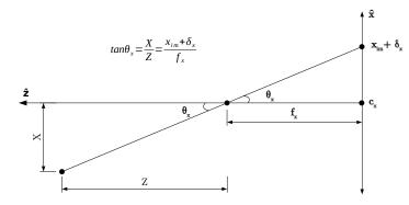
Figure 5.4: Note the relationship formed by the tangent of the angle  $\theta_x$ . A similar relationship exists in the y direction.
