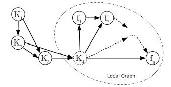
Figure 4.3: DVO SLAM graph structure showing the local graph in relation to the global keyframe graph.
