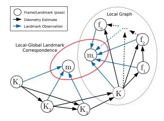
Figure 5.3: The local-to-global graph merge procedure for landmark vertices. A correspondence has been established between the local landmark vertex  $m_l$ , and the global vertex m. The merge procedure maps the observations associated with  $m_l$  onto m, and  $m_l$  is subsequently removed from the graph.
