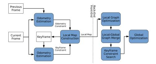
Figure 4.1: A high-level overview of the DVO SLAM algorithm showing RGBD image data in white and processes in blue. Note the separation of responsibilities between the front-end and the back-end.
