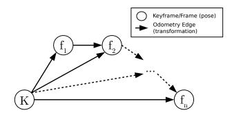
Figure 4.2: DVO SLAM local graph structure showing odometry constraints between consecutive frames/poses and the keyframe.
