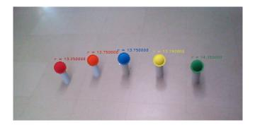
Figure 5.10: Output from the object appearance detector showing colored circle detections in the RGB image.
