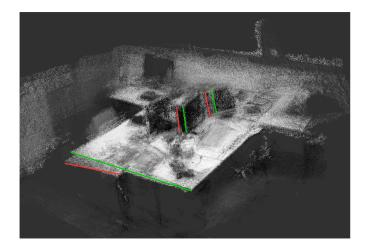
Figure 5.1: Reconstructed point cloud of the fr1/desk dataset using DVO SLAM with default settings [17, 36]. Some errors in the reconstruction are highlighted in red with the green lines showing the correctly reconstructed surface. We seek to reduce this mapping error and enhance map semantics by considering detected object poses in the SLAM optimization.
