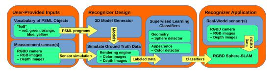
Figure 5.6: Overview of the framework used to semantically model and detect object instances. Detected object instances can be leveraged for a variety of purposes including SLAM.
