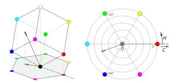
Figure 5.9: The hue-chroma plane formed by the projection of the RGB space onto the intensity axis. This polar space is used for pixel color classification. Images courtesy J. Rus, Creative Commons, Licensed under CC BY-SA 3.0, Modified.
