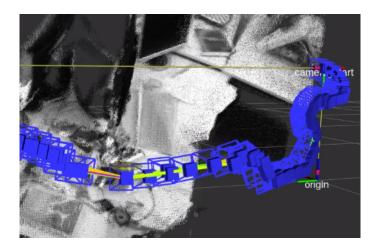
Figure 4.5: Visualization of the camera trajectory and the dense point cloud map of DVO SLAM.
