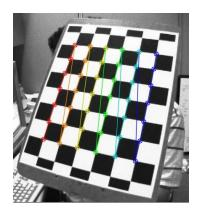
Figure 2.2: A checkerboard pattern used for camera calibration. [1]
