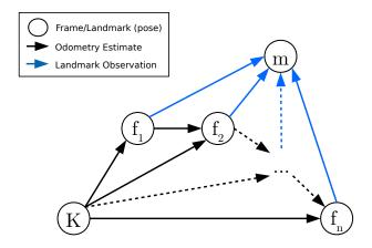
Figure 5.2: DVO SLAM local graph structure showing odometry constraints between frames/poses as well as landmark observations of a map feature labeled m.
