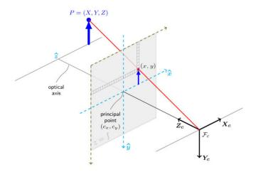
Figure 2.1: Pinhole camera model showing the relationship between 3D world points and their projection onto the image plane. Modified from OpenCV API Reference: Camera Calibration and 3D Reconstruction [1].
