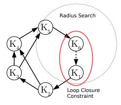
Figure 4.4: DVO SLAM identifies candidate keyframes for loop closure constraints. When a new keyframe is added to the global graph, a radius identifies existing nearby keyframes as candidates to build constraints from. Dense odometry estimation is then performed between the keyframe and candidate keyframes.
