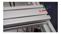
Fig. 3.7. Coordinate system for reporting straightness measurement
