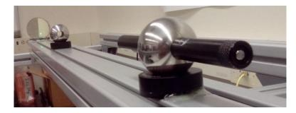
Fig. 5.3. Use of laser pointer for alignment of tracker's beam
