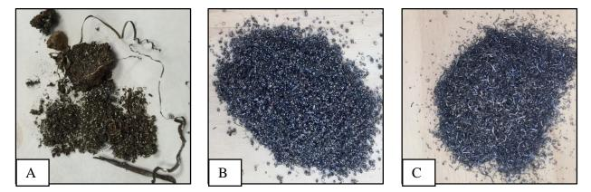
Figure 5-1 Recycled Steel Residuals in Raw Form (A), Retained on No. 8 Sieve (B), and Passing Through No. 8 Sieve (C)
