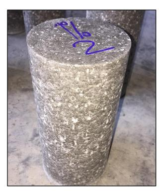
Figure D-2 Cylinder used for Testing Containing 1% RSR Concentration
