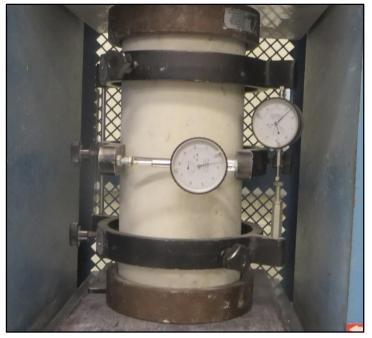
Figure D-8 Modulus of Elasticity Testing – 6x12-in. Cylinder
