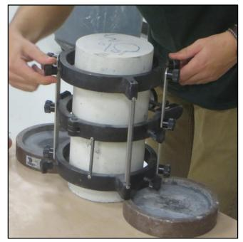
Figure D-7 Modulus of Elasticity Setup
