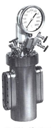
2000 mL Stirred Reactor with Two Elliptical Quartz Windows
