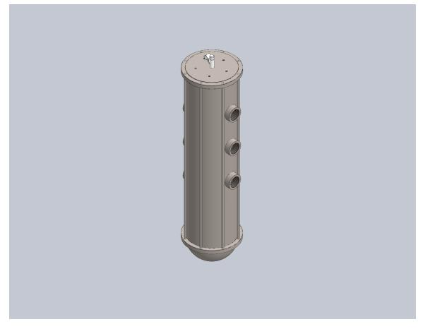
Figure 40: Final Design of Pressure Vessel Model Initially, the top lid was designed as a dome shape to increase the manufacturability. However, this approach was not viable because of the mounting and installation of the fuel injector. Figure 41 shows a sectional view which is cut directly in
