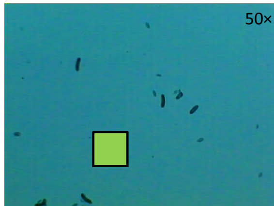
Figure 5-32. An overlay of the confocal fluorescence microscope's field of view ( 40\ \mu\text{m} \times 40\ \mu\text{m} ) on an image of an etched sample that reveals subsurface defects illustrates the possibility of missing defects without thorough sampling.
