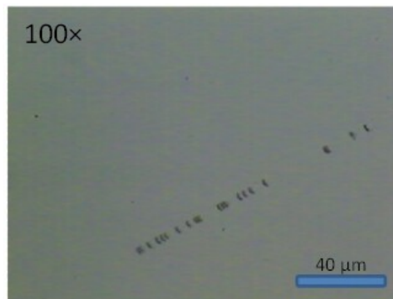
2-12. Glass sample etched to reveal SSD 'chatter marks' characteristic of dynamic stresses around a traveling abrasive.
