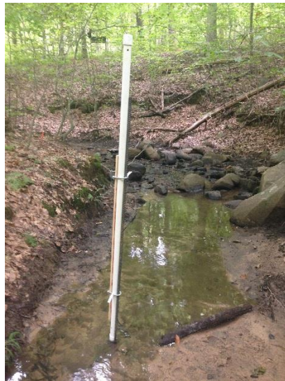
Figure 6: Crest gage installation example
