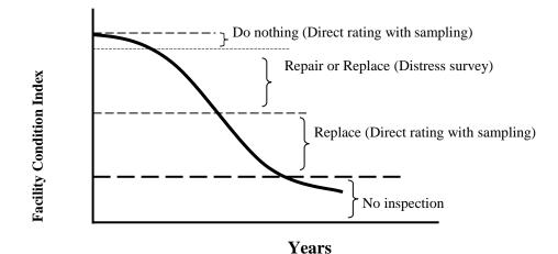
Figure 5: Life cycle repair vs replacement needs adapted from Uzarski (2007)
