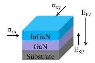
Figure 2.12: SP and PZ polarization of InGaN grown on Ga-faced GaN
