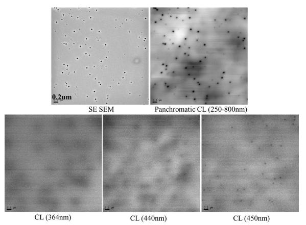
Figure 6.18: SE SEM, panchromatic CL, and monochromatic CL (at 362nm and 452nm) images of MQW sample A3 at 8keV EB voltage and 30um aperture size
