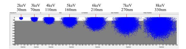
Figure 5.6: Schematic of the diffusion of EB into the MQW sample A3
