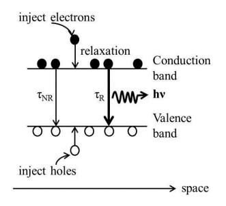
Figure 2.1: General schematic of luminescence in semiconductor materials
