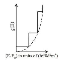
Figure 2.10: Step like density of states for a quantum well
