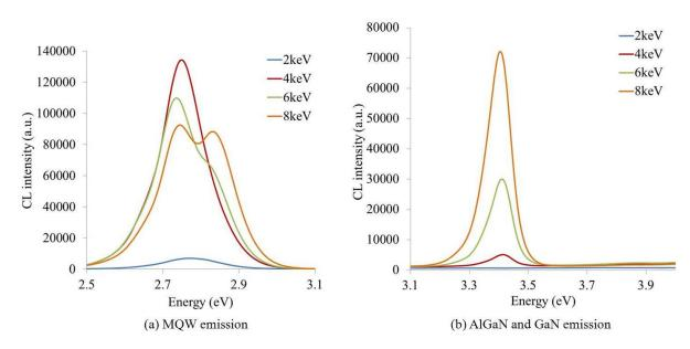
Figure 6.34: CL spectrums at MQW, AlGaN and GaN emissions at 2, 4, 6 and 8keV EB voltages for sample A2
