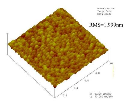
Figure 3.8: AFM image of GaN nucleation layer
