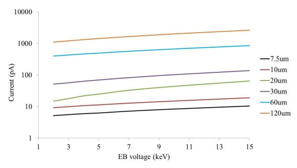
Figure 5.5: CL beam current versus EB voltage and aperture size
