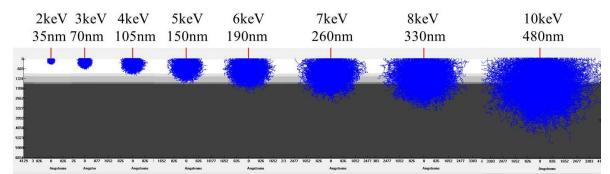
Figure 6.41: EB penetration volume in LED sample A1 simulated by EFS
