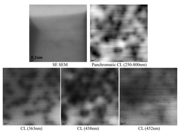
Figure 6.38: SE SEM, panchromatic CL, and monochromatic CL images of A2 at 8keV EB voltage and 30um aperture size
