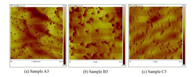
Figure 6.9: AFM images of MQW samples A3, B3 and C3
