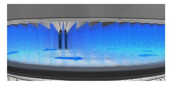
Figure 3.3: The schematic cross section of the Uniform Flow Flange® with separate alkyl and hydride slits. The blue dots represent the pathway for the hydrides, while red dots represent pathway for alkyls
