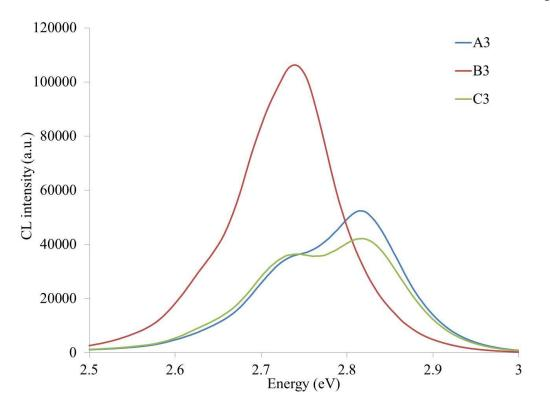
Figure 6.22: CL spectrum at 8keV EB voltage and 30um aperture size for sample A3, B3 and C3
