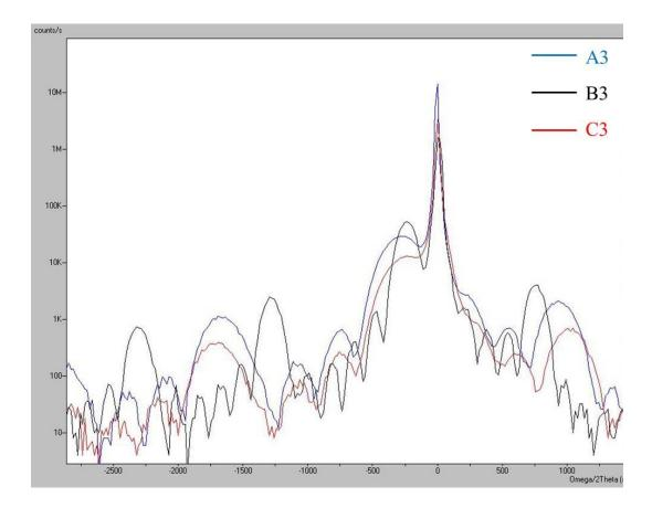
Figure 6.10: Triple axis XRD scan of MQW samples A3, B3 and C3
