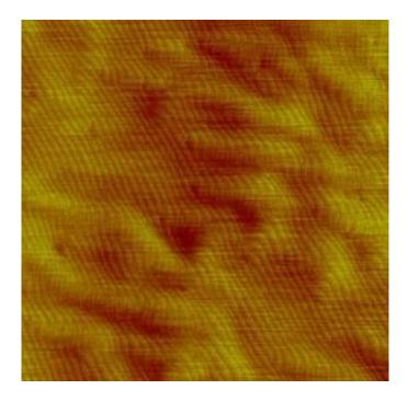
Figure 3.14: 5um by 5um AFM of p-AlGaN capped MQW structure
