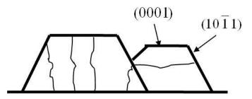
Figure 3.10: Schematic of the coalesced 3D islands
