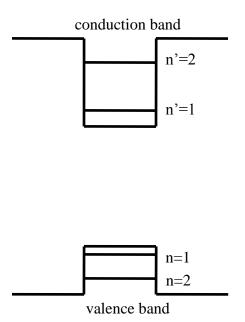
Figure 2.9: Energy levels in the quantum well
