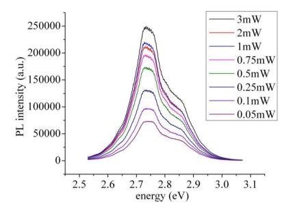
Figure 6.11: Room temperature power dependent PL spectrum of sample A3
