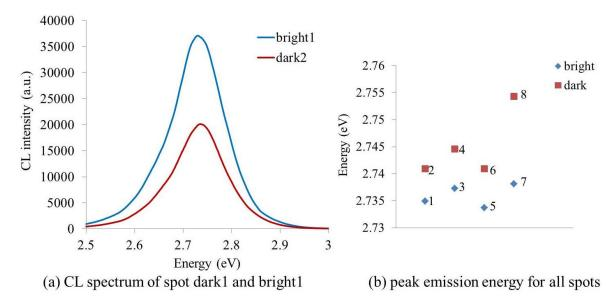
Figure 6.20: (a) CL spectrum of spot b1 and d1 and (b) the peak emission energies of all 8 spots
