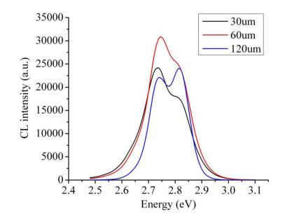
Figure 6.24: CL spectrum at 30um, 60um and 120um aperture sizes at 6keV EB voltage
