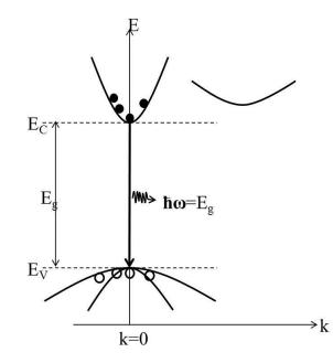
Figure 2.2 Interband luminescence process in a direct bandgap semiconductor
