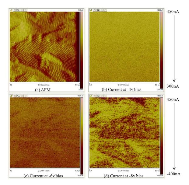
These point defects cause leakage and deteriorate the device performance [64].
