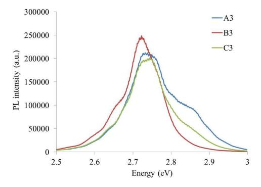
Figure 6.12: Room temperature PL spectrums of sample A3, B3 and C3 at 2mW pulse power
