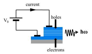
Figure 2.5: Circuit diagram for a MQW LED structure
