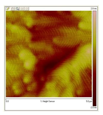
Figure 6.32: AFM images of AlGaN capped MQW sample A2
