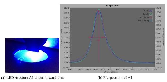
Figure 6.39: Picture of LED As-grown sample A1 at forward bias (a) and measured EL spectrum at 20mA driving current (b)
