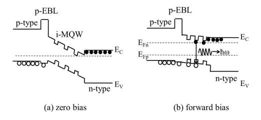
Figure 2.6: Band diagrams of a MQW LED with p-type EBL at (a) zero bias, and (b) forward bias
