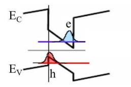
Figure 1.11: Bending of the band diagram due to QCSE
