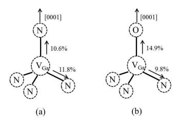
Figure 6.31: Atomic geometry of the  $V_{Ga}^{3-}$  and  $(V_{Ga}-O_N)^{2-}$  complex
