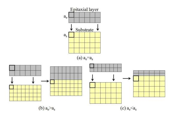
Figure 2.7: Accommodation of lattice between epitaxial layer and substrate
