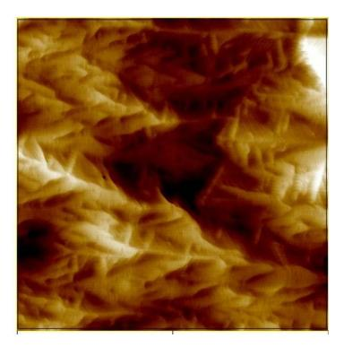
Figure 3.16: 5um by 5um AFM of the full LED structure
