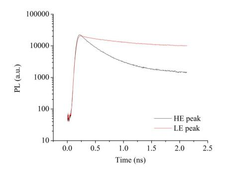
Figure 6.25: Time resolved PL curves at room temperature at HE and LE peak energies with a 5nm bandpass
