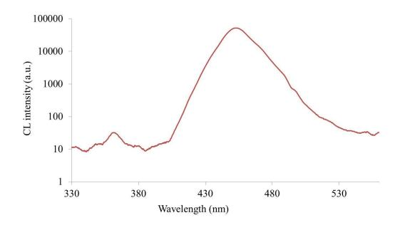
Figure 6.13: CL spectrum of A3 at 2keV EB voltage and 30um aperture size
