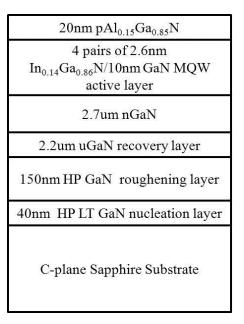
Figure 5.3: Schematics of pAlGaN capped MQW structure A2
