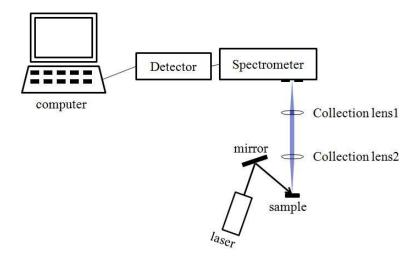
Figure 2.4: Photoluminescence test setup
