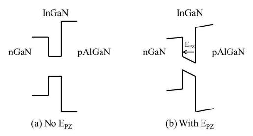
Figure 2.13: Schematic of the band structure of an InGaN SQW structure (a) without and (b) with PZ effects
