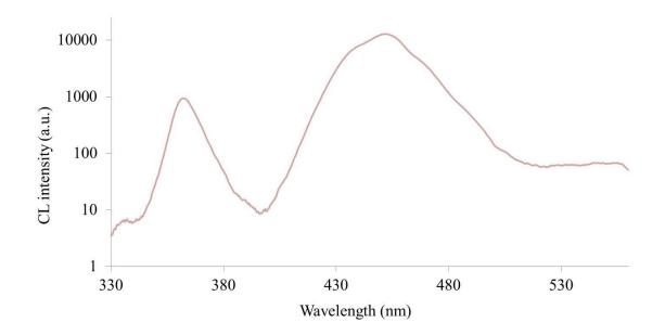
Figure 6.15: CL spectrum of A3 at 4keV EB voltage and 30um aperture size
