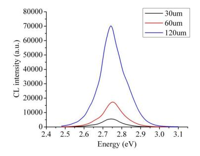
Figure 6.23: CL spectrum at 30um, 60um and 120um aperture sizes at 3keV EB voltage
