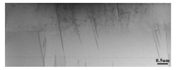
Figure 6.7: Cross-section STEM image of GaN A4
