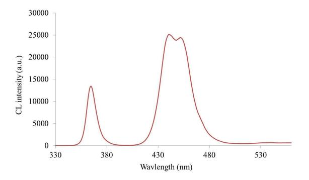
Figure 6.17: CL spectrum of A3 at 8keV EB voltage and 30um aperture size
