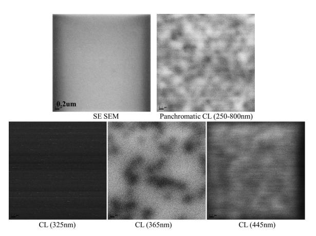
Figure 6.43: SE SEM, panchromatic CL, and monochromatic CL (at 325nm, 365nm and 445nm) images of LED A1 at 10keV EB voltage and 30um aperture size
