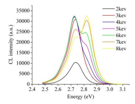
Figure 6.21: CL spectrum at 2-8keV EB voltages at 30um aperture size
