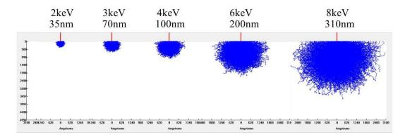
Figure 6.3: EB penetration volume in bulk nGaN simulated by EFS
