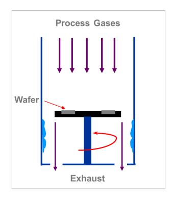
Figure 3.1: The schematics of vertical rotating disc growth chamber
