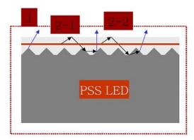
Figure 3.7: schematic of light extraction from LED grown on PSS
