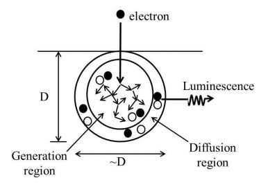
Figure 4.1: Schematic of electron cascade process
