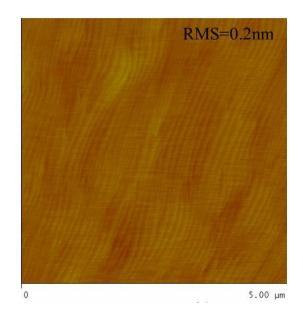
Figure 3.11: AFM of nGaN layer
