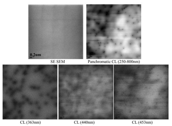
Figure 6.37: SE SEM, panchromatic CL, and monochromatic CL images of A2 at 6keV EB voltage and 30um aperture size
