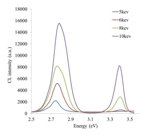
Figure 6.42: CL spectrums at 5, 6, 8 and 10keV EB voltages for LED structure A1
