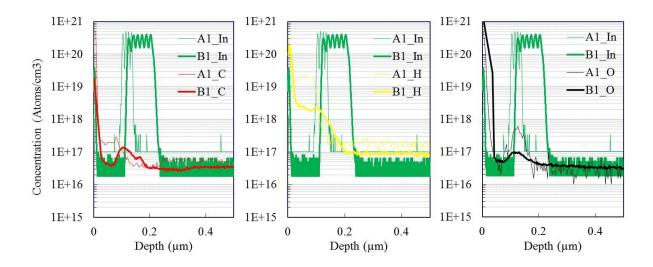
Figure 6.30: SIMS profile for In, C, H, and O on LED sample A1 and B1
