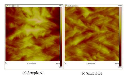
Figure 6.40: AFM images of LED sample A1 and B1
