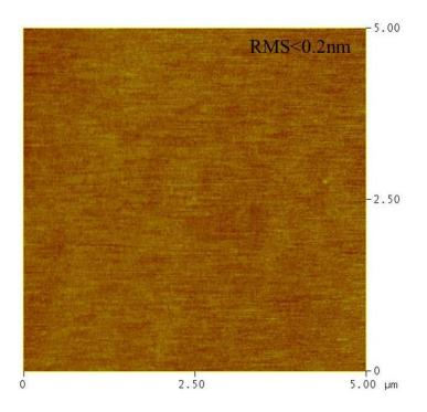
Figure 3.6: AFM image of c-plane sapphire substrate
