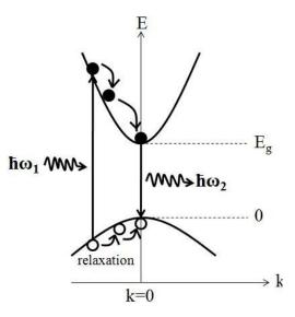
Figure 2.3: Photoluminescence in a direct bandgap semiconductor
