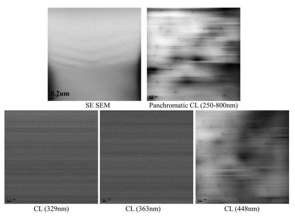
Figure 6.35: SE SEM, panchromatic CL, and monochromatic CL (at 329nm, 363nm and 448nm) images of AlGaN capped MQW sample A2 at 2keV EB voltage and 30um aperture size
