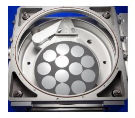
Figure 3.2: 12x4" SiC Coated Graphite Platter loaded with sapphire wafers
