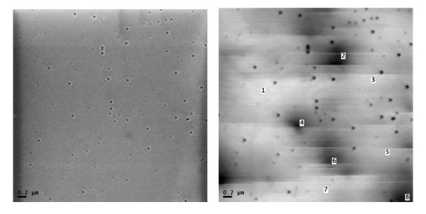
Figure 6.19: SEM (left) and panchromatic CL (right) images at 2keV EB voltage and 30um aperture size. In the CL image, spots 1, 3, 5, and 7 are from bright regions, and 2, 4, 6, and 8 dark.
