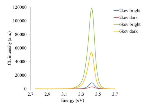
Figure 6.6: CL spot spectrums at bright and dark spots at 2keV and 6keV EB voltages on sample A4
