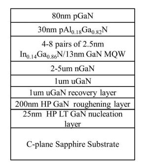
Figure 3.5: Schematic of a typical InGaN/GaN MQW LED structure grown by MOCVD
