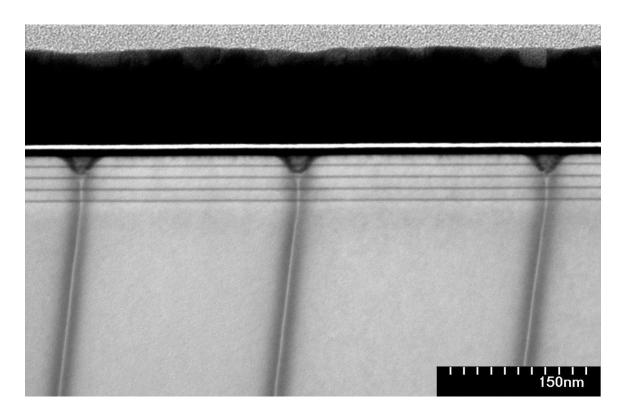
Figure 3.13: Cross section STEM image of V-pit on InGaN/GaN MQW
