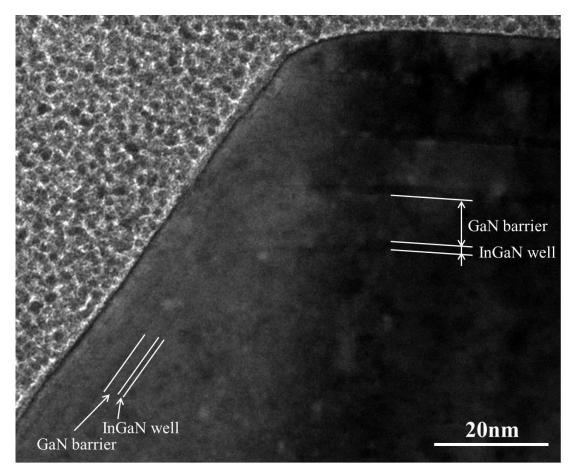
Figure 6.29: Cross section TEM image of MQW A3 at a V-pit
