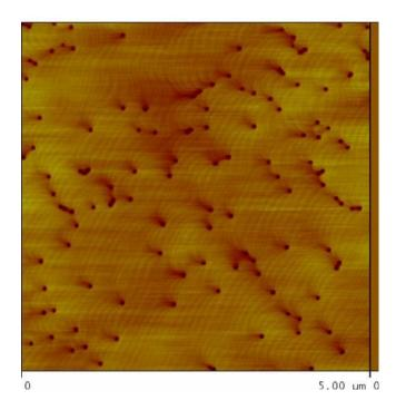
Figure 3.12: AFM of InGaN/GaN MQW layer
