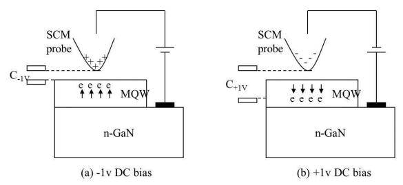
Figure 6.28: Schematic of the SCM system when the DC bias is at -1v (a) and +1v (b)
