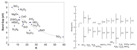
Figure 5. Diagrams illustrating (a) a relationship between band gap and dielectric constant of candidate oxides, and (b) conduction and valence band offset with respect to silicon.[9]
