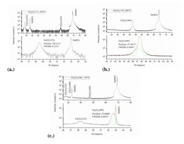
Figure 15. XRD patterns of three possible growth mode of the  $Gd_2O_3$  on Si(100) grown at (a.) 150°C, (b.) 600°C and (c.) 450°C
