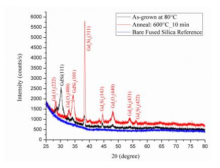
Figure 22. XRD patterns of an 80 nm-thick Gd<sub>2</sub>O<sub>3</sub> deposited on fused silica substrate at 200°C before and after annealing in furnace with N<sub>2</sub> ambient
