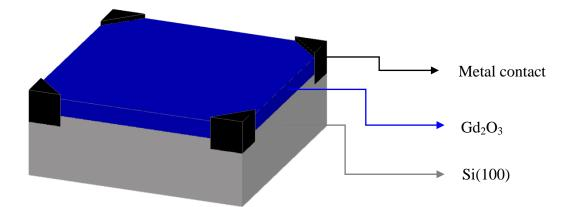
Figure 14. Van der Pauw configuration for Hall measurement
