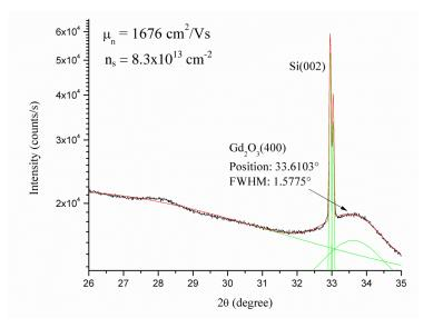
Figure 30. Hall mobility measurement of the 30 nm-thick poly crystal with a predominant  $Gd_2O_3(100)$  grown on n-type Si(100) with the amorphous silicon capping layer (50 nm)
