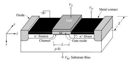
Figure 1. Schematic diagram of a planar MOSFETs structure [1]
