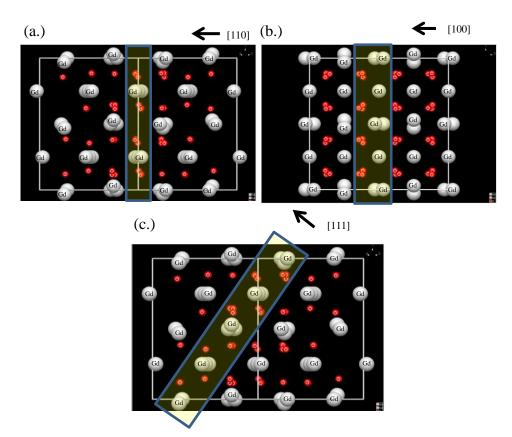
Figure 9. Illustration of the (a.) (110) plane, (b.) (100) plane and (c.) (111) plane within the Gd<sub>2</sub>O<sub>3</sub> cubic bixbyite structure [56]
