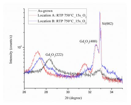
Figure 21. XRD patterns of the 60 nm-thicked  $Gd_2O_3$  deposited on n-type Si(100) at 175°C, before and after RTA at different location.
