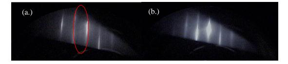
Figure 13. RHEED pattern of the Si(100) surface at 200°C before the growth with the temperature ramp of (a.) 20°C and (b.) 10°C.
