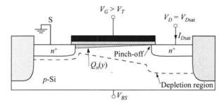
Figure 3. Schematic diagram illustrating pinch-off of the inversion layer at  $V_D = V_{Dsat} = V_G - V_T$ . [1]
