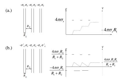
Figure 10. Diagrams illustrating relationships between electric field, electrostatic potential and a thickness in the direction perpendicular to the surface of the (a.) uncompensated and (b.) compensated polar surface. [34]
