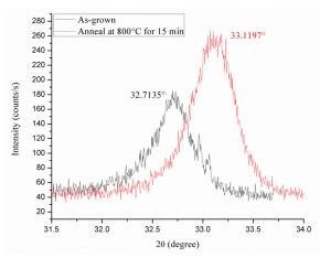
Figure 18. XRD pattern illustrating the strain relaxation of the 150nm-thick Gd<sub>2</sub>O<sub>3</sub>(100) grown on p-type Si(100) after the annealing at 800°C for 15 min
