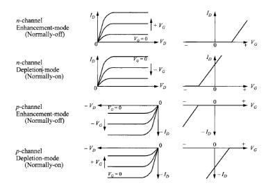
Figure 2. Relationship between the drive current  $(I_D)$ , drain bias  $(V_D)$  and gate bias  $(V_G)$  of n- and p-channel MOSFETs in enhancement and depletion mode [1]
