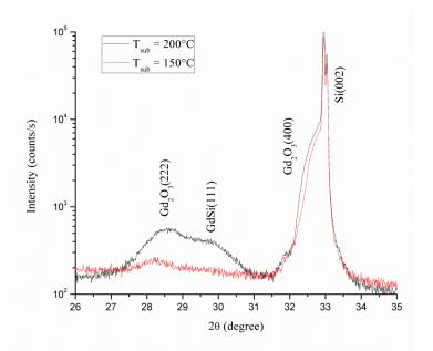
Figure 20. XRD patterns of the polycrystal with predominant  $Gd_2O_3(100)$  structure grown on the intrinsic Si(100) illustrating the suppression of the silicide formation through a low growth temperature.
