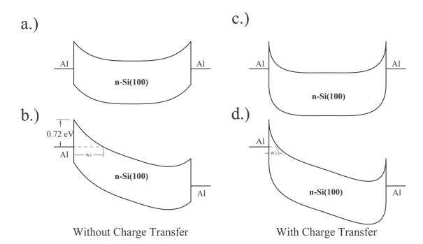
Figure 25. Interface Band diagrams between two Al contacts without the charge transfer (a, b) and with the charge transfer (c, d) at equilibrium and with applied bias.
