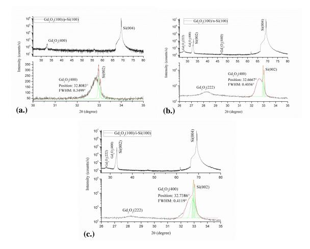
Figure 17. XRD patterns showing different structure obtained from different substrate. a.) p-type Si(100), b.) n-type Si(100), c.) intrinsic Si(100)
