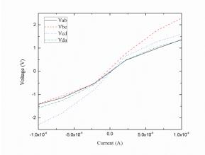
Figure 33. IV curve showing a decent ohmic characteristic between the four Al contacts on n-type substrate with the  $Gd_2O_3(110)$  deposited on top
