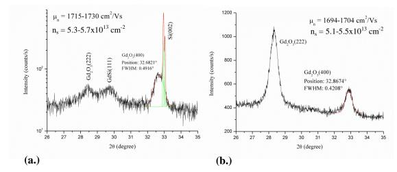
Figure 28. Degradation of Hall mobility due to different structural composition of the (a.) 90-nm and (b.) 80-nm thick polycrystalline Gd<sub>2</sub>O<sub>3</sub> grown on the n-type substrate
