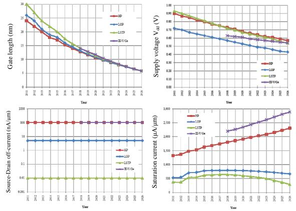
Figure 4. ITRS 2011 scaling trend of logic technologies with year; (a.) Gate length, (b.) Supply voltage, (c.) Off-current, (d.) Saturation on-current. (HP = High Performance, LOP = Low Operating Power, LSTP = Low Standby Power) [7]
