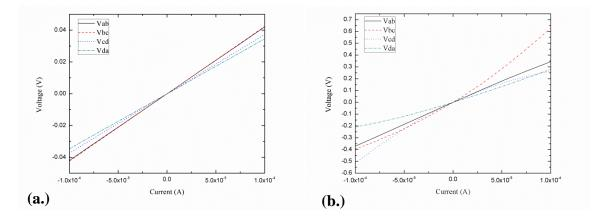
Figure 24. IV curve showing an ohmic characteristic between the four Al contacts on (a.) p-type and (b.) n-type substrate
