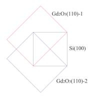
Figure 7. Illustration of alternative lattice matching between two domain of  $Gd_2O_3(110)$ and Si(100)
