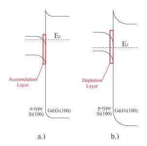
Figure 12. Band diagrams illustrating the accumulation in the conduction band of the n-type silicon (a.) and the compensation in the valence band of the p-type silicon (b.).
