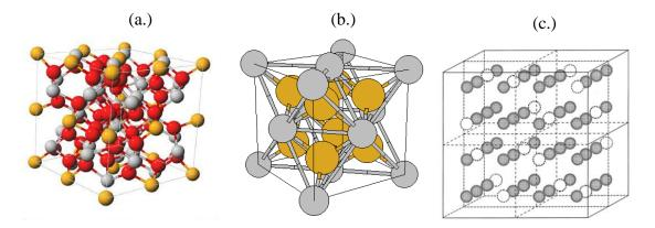
Figure 6. Illustration of (a.) cubic bixbyite structure [Gray =  $Gd^{3+}$ , Red =  $O^{2-}$ , Yellow = surface  $Gd^{3+}$ ], (b.) fluorite structure [Gray = cation (Ce<sup>2+</sup> or Ca<sup>2+</sup>), Yellow = anion (O<sup>2-</sup> or F<sup>2-</sup>)], and (c.) positions of oxygen (gray sphere) and oxygen vacancies (hollow sphere) within the cubic bixbyite unit cell [39-41]
