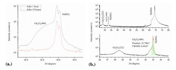
Figure 19. XRD pattern illustrating (a) the instability of the 30 nm-thicked  $Gd_2O_3(100)$  grown on the intrinsic Si(100) substrate through the disappearance of the  $Gd_2O_3(400)$  peak over a course of 19 hours, and (b) a stable  $Gd_2O_3(100)$  on i-Si(100) with a lower crystalline quality.
