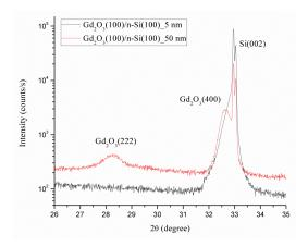
Figure 16. XRD pattern of the growths on n-type Si(100) comparing a single crystal  $Gd_2O_3(100)$  and the polycrystal with a predominant  $Gd_2O_3(100)$  structure. The thicknesses for each sample are 5 and 50 nm, respectively.
