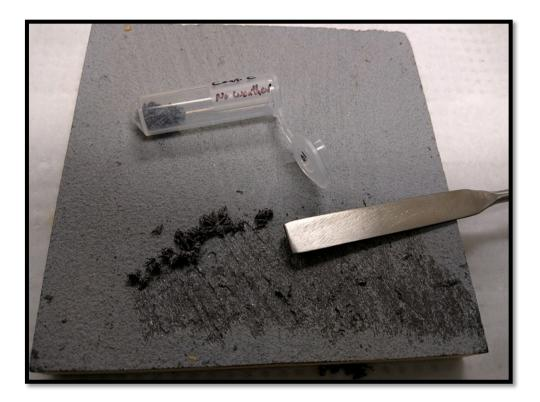
Figure 3.8. Sample collection for SDT tests- coating C
