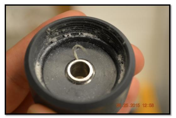
Figure 3.6. Desiccant holder cap after testing
