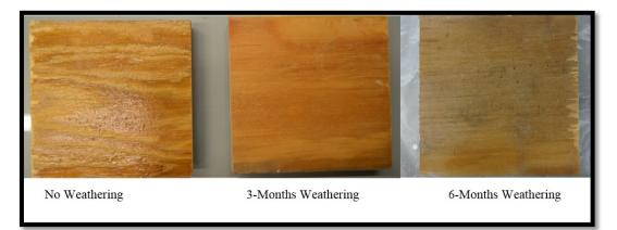
Figure 4.1. Visible weathering effects on coating A
