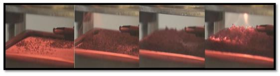
(1) 5s (2) 10s (3) 15s (4) 20s Figure 4.28.a. Coating C- north- 6-months weathered-  $HF=70 \text{ kW/m}^2$
