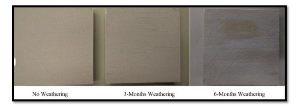
Figure 4.3. Visible weathering effects on coating C
