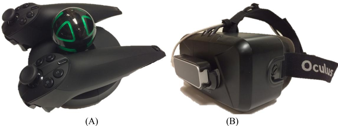
Figure 6.2: (A) The Razer Hydra game controller. (B) The Oculus Rift DK2 with Leap Motion VR Setup.
