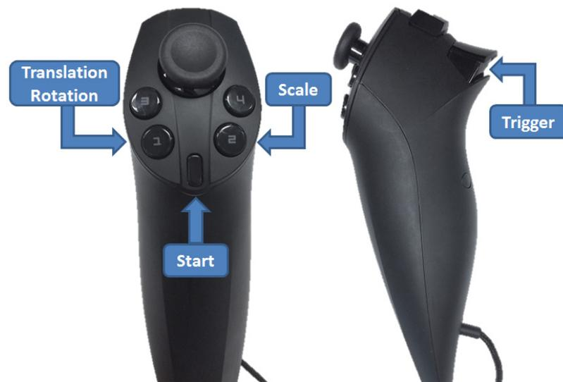
Figure 7.5: Button usage on the Razer Hydra Controller.
