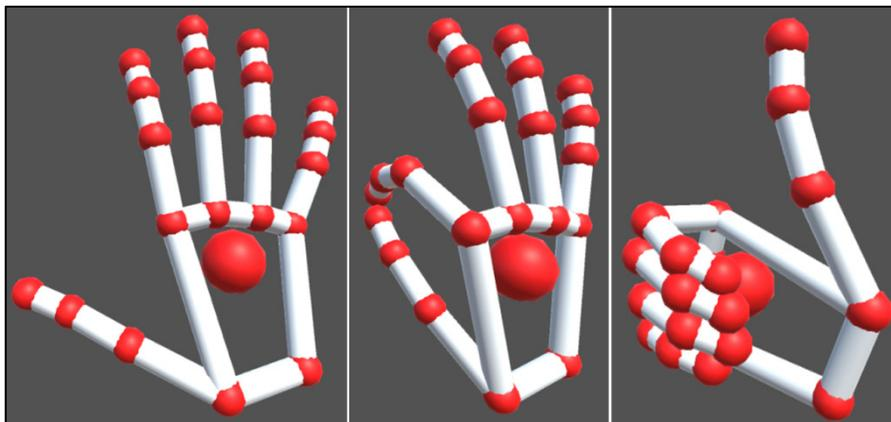
Figure 7.6: Gestures used in the experiment with the Leap Motion controller. From left to right: open hand, pinching and thumb up.
