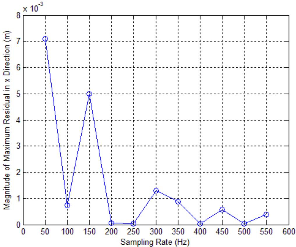
FIGURE 5.12: Maximum residual magnitude for  $x$ -direction displacement in the planar structure verification, as time step size decreases
