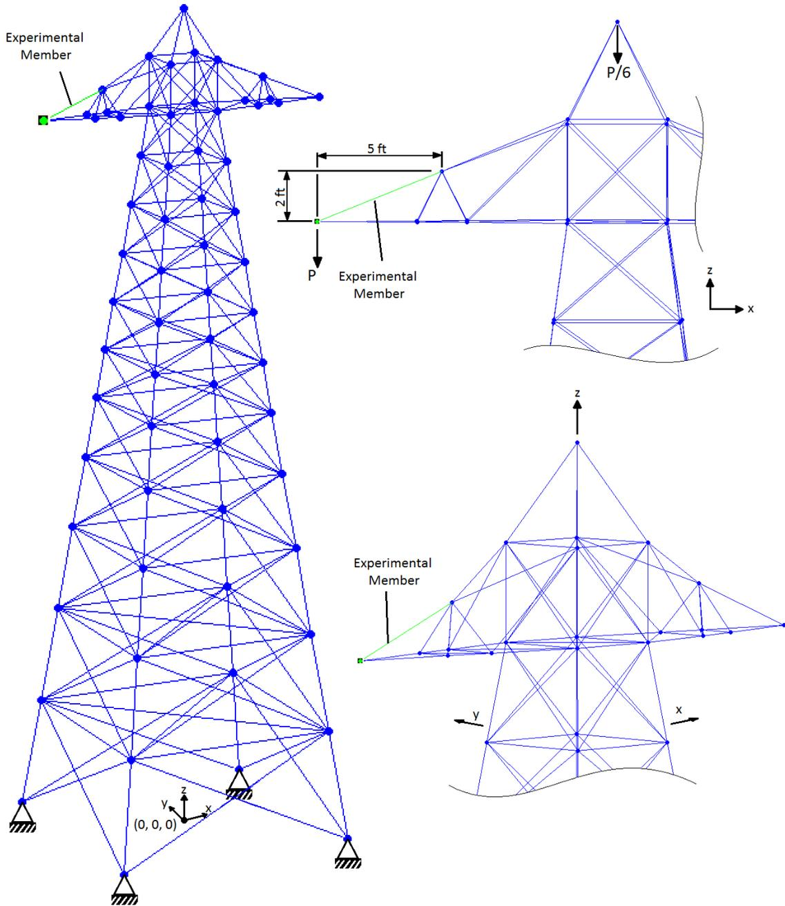
FIGURE 6.2: Transmission tower model subjected to hypothetical galloping conductor and ground wire for experimental validation
