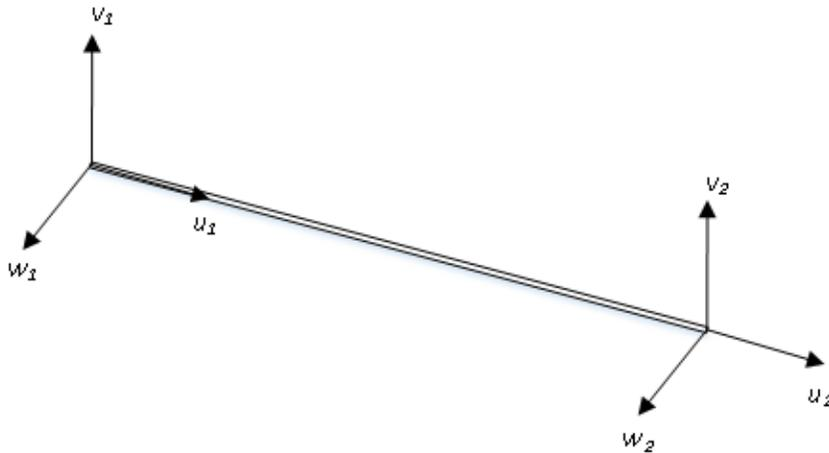
FIGURE 3.1: Local degrees of freedom for elements in example model
