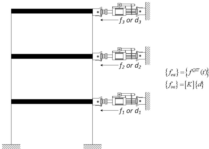
FIGURE 2.1: Quasi-static testing methodology
