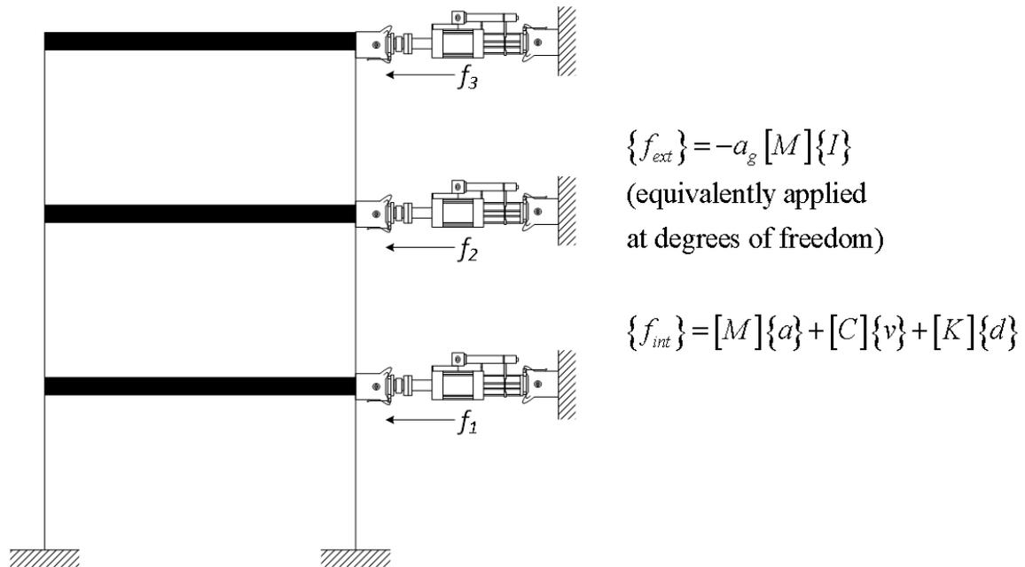
FIGURE 2.3: Effective force testing methodology
