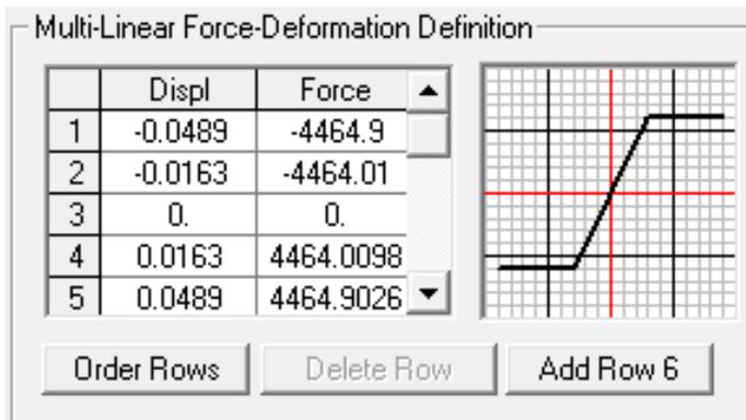
FIGURE 5.1: Multilinear elastic material model assignment in SAP2000
