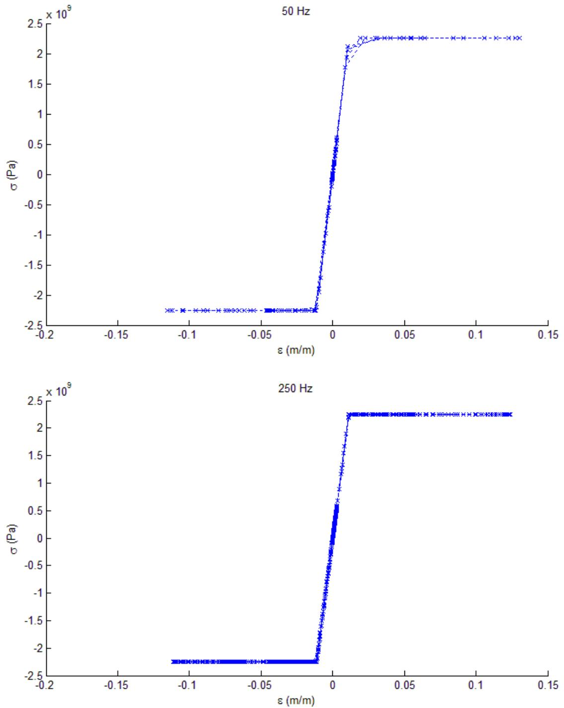
FIGURE 5.13: Stress-strain curves produced in the HSF for the 50 Hz and the 250 Hz sampling cases
