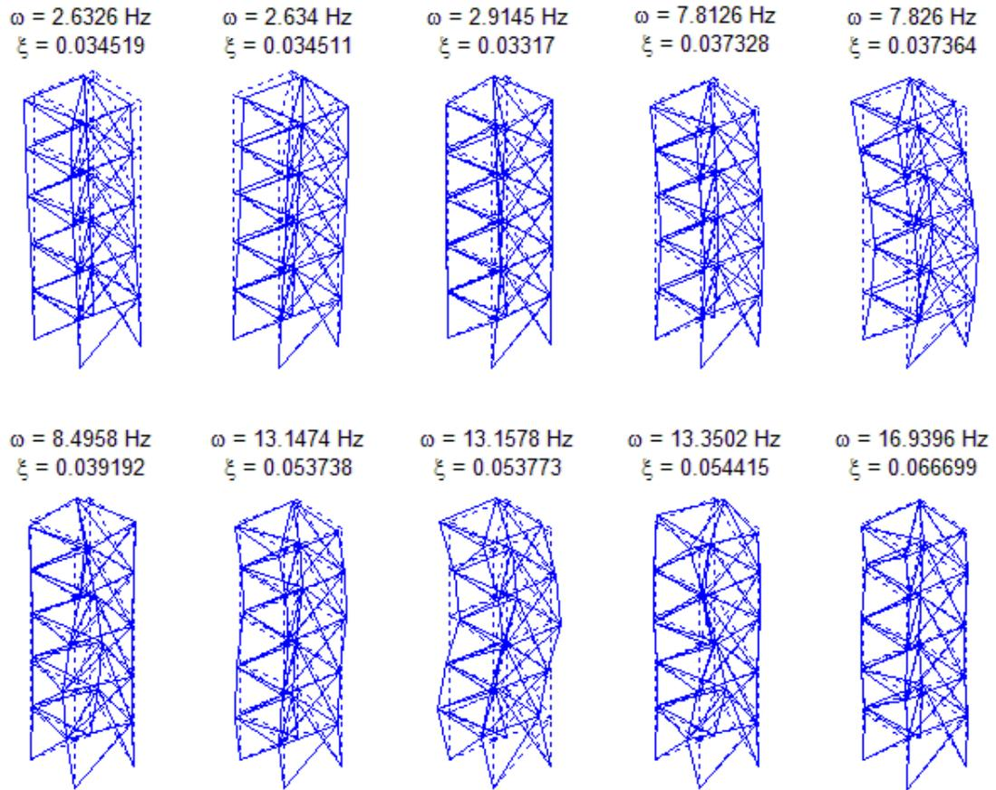
FIGURE 5.9: Mode shape plots for each of the first ten natural frequencies of the three-dimensional model
