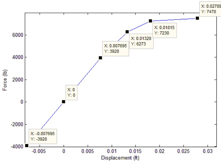
FIGURE 6.8: Force-displacement relationship definition used in SAP2000 to perform *ex post facto* analysis for comparison to experimental nonlinear simulation
