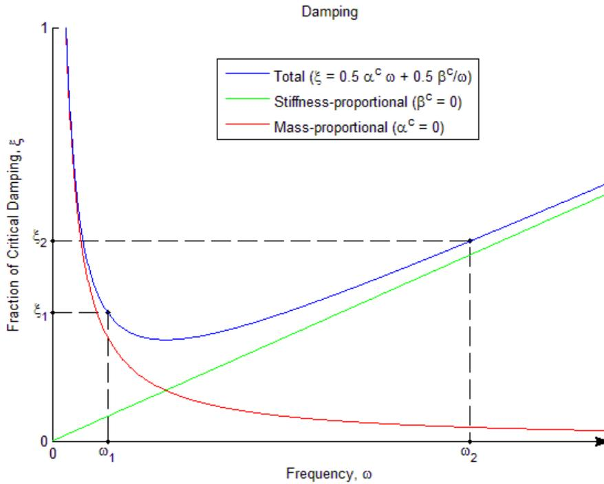
FIGURE 4.2: Proportional damping and critical damping ratios as functions of frequency, adapted from textbook [Cook, 1974]
