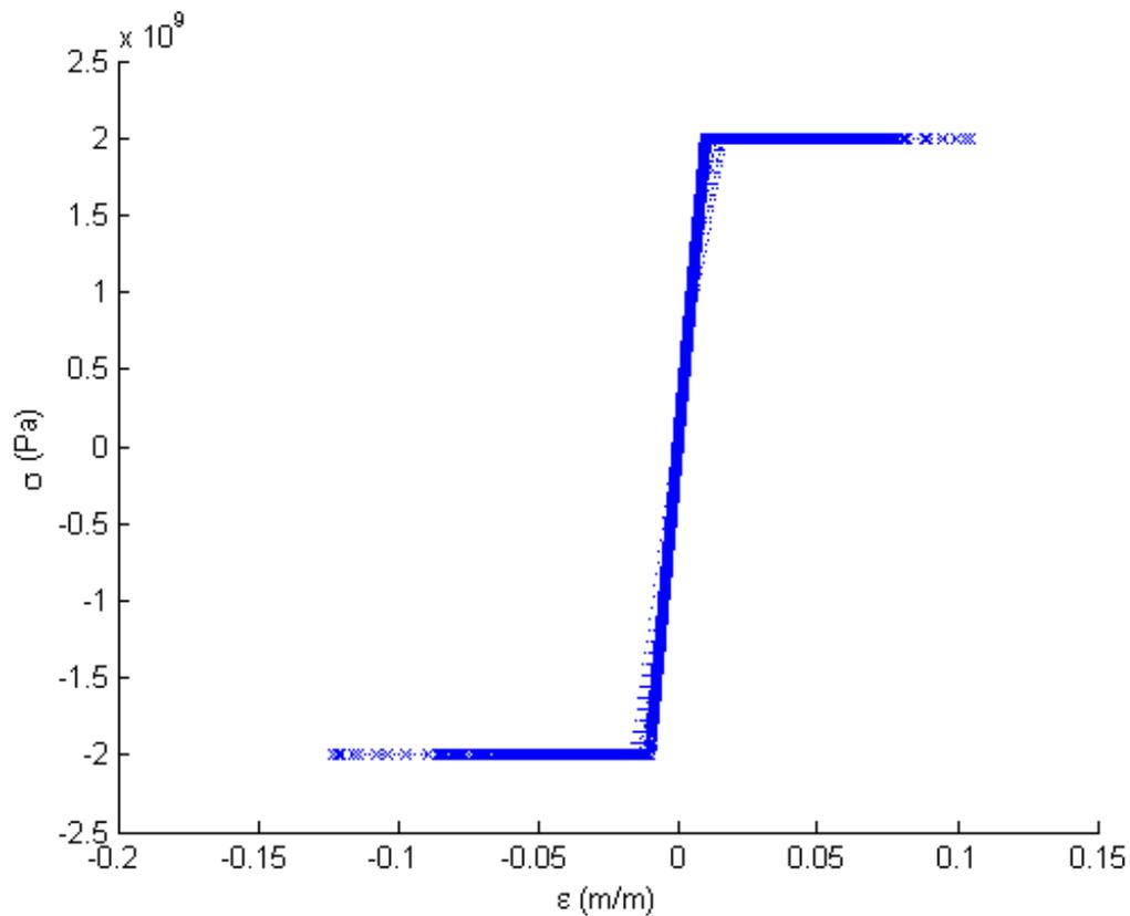
FIGURE 5.11: Stress-strain plot for experimental member in three-dimensional model
