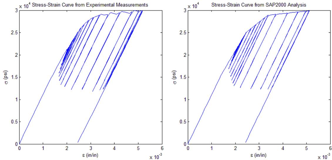
FIGURE 6.9: Experimentally-observed hysteresis and analytically-simulated hysteresis
