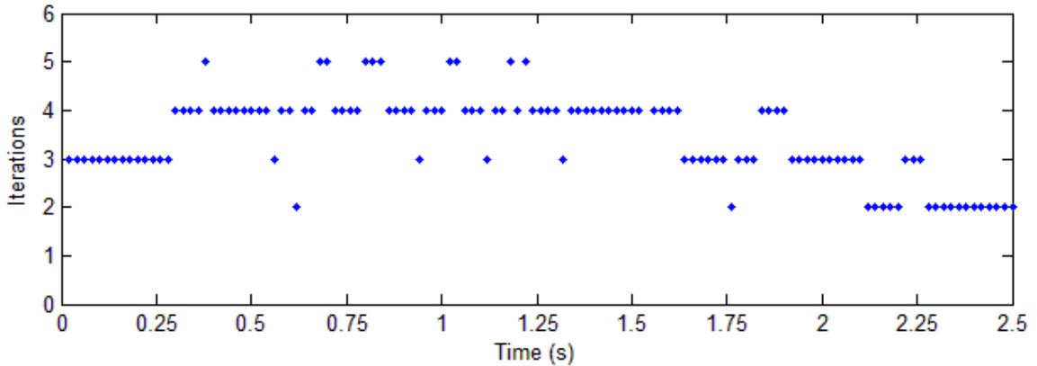
FIGURE 5.6: Iterations required for convergence throughout time history of NLMNLG case
