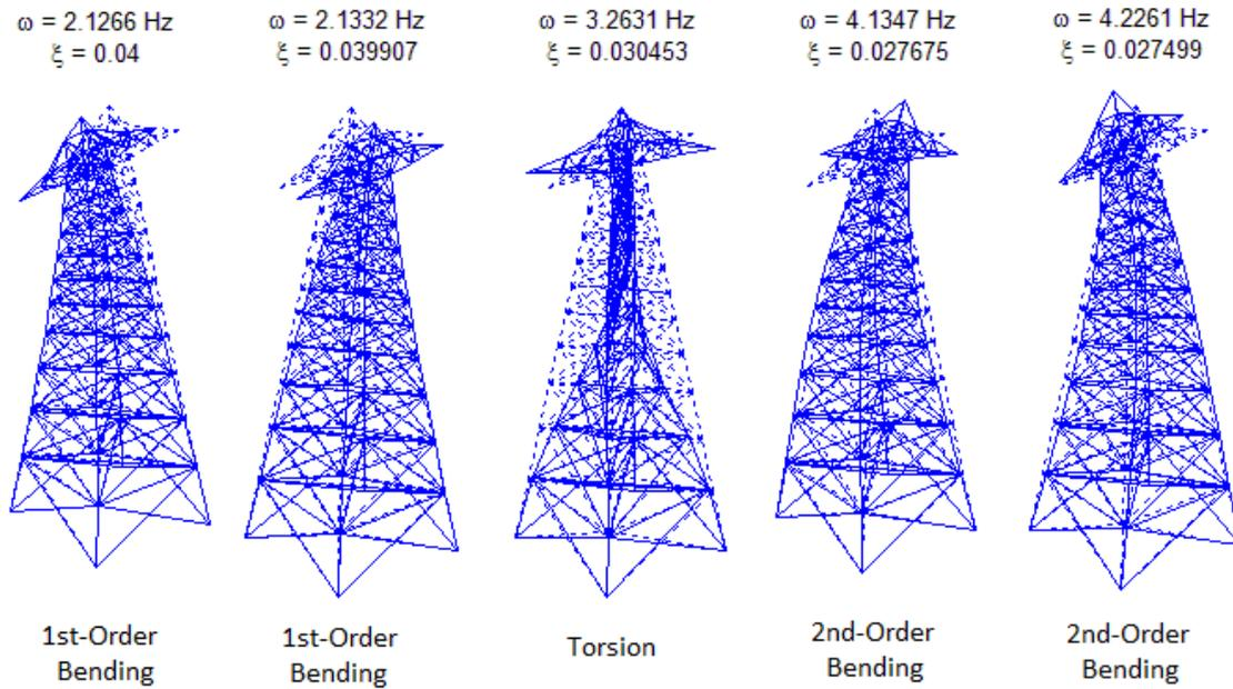
FIGURE 6.3: First five vibration modes for transmission tower model
