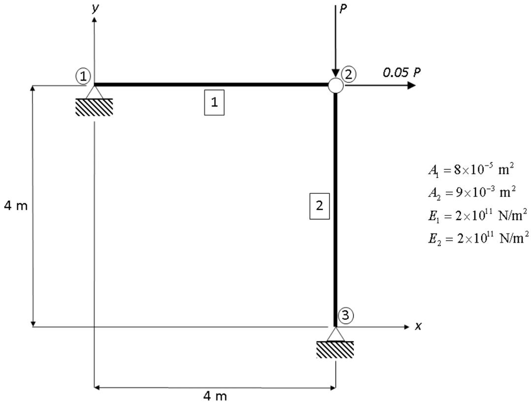
FIGURE 3.2: Two-degree-of-freedom truss model used for geometrically nonlinear analysis
