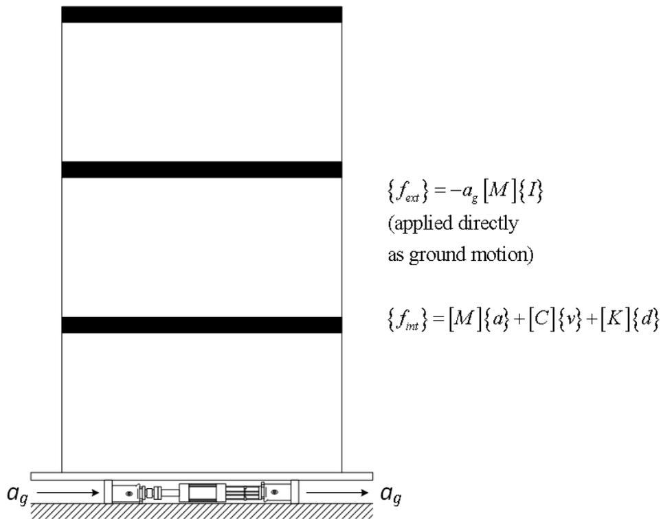
FIGURE 2.2: Shake table testing methodology
