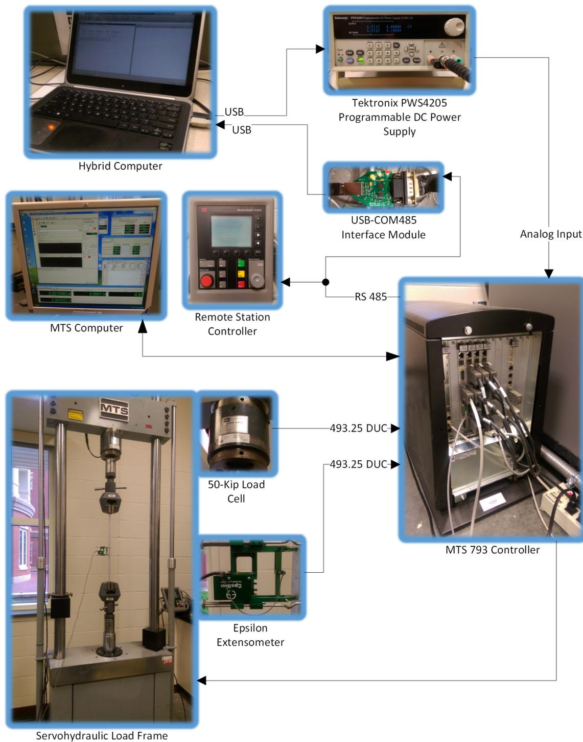
FIGURE 6.1: Schematic of hardware and interfaces used to establish the hybrid testing experimental demonstration
