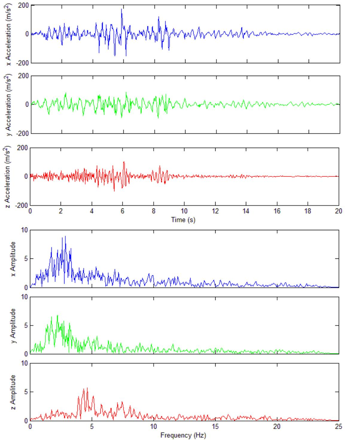
FIGURE 5.8: Northridge ground accelerations and amplitude spectra, scaled by a factor of 10
