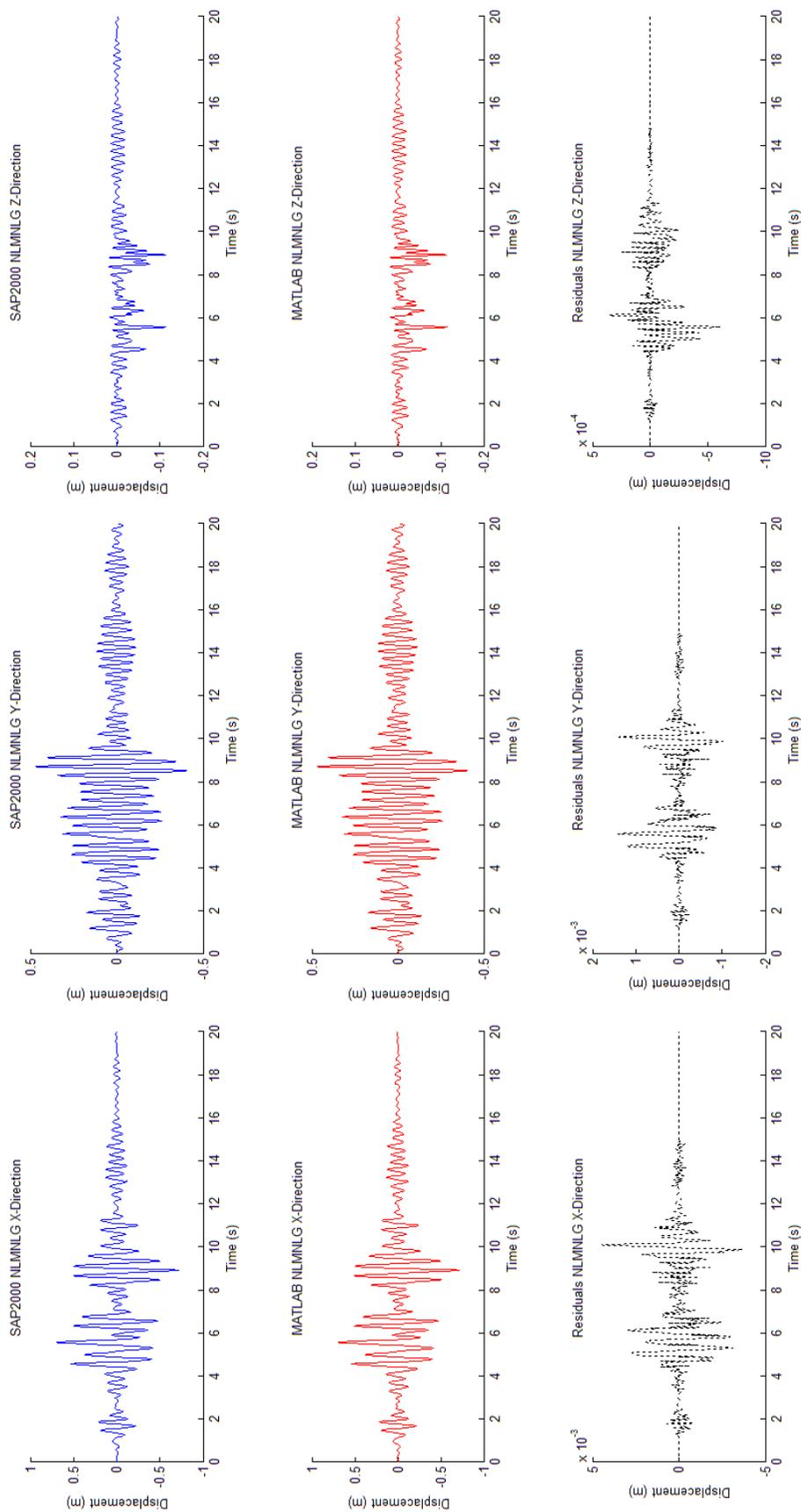
FIGURE 5.10: Verification results for base excitation of a three-dimensional structure with nonlinear material and geometric effects
