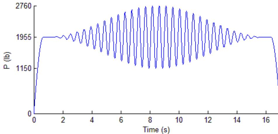
FIGURE 6.5: Load  $P$  applied to transmission tower model for nonlinear simulation
