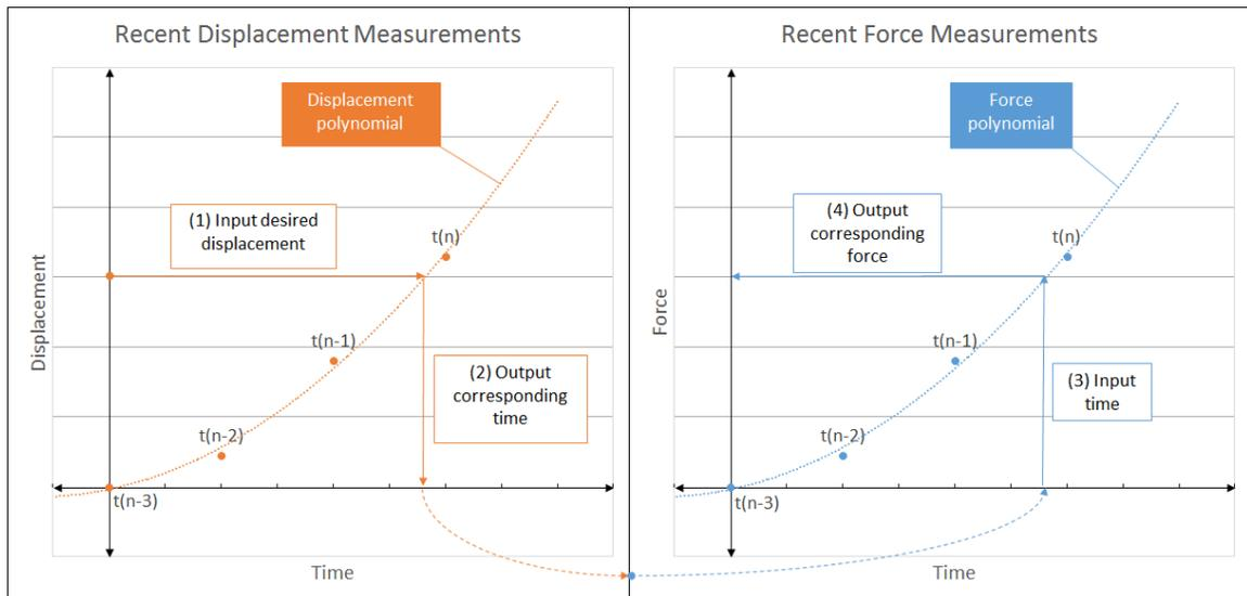
FIGURE 4.3: Estimation procedure using fitted polynomials, adapted from Mosqueda and Ahmadizadeh [Mosqueda and Ahmadizadeh, 2011]
