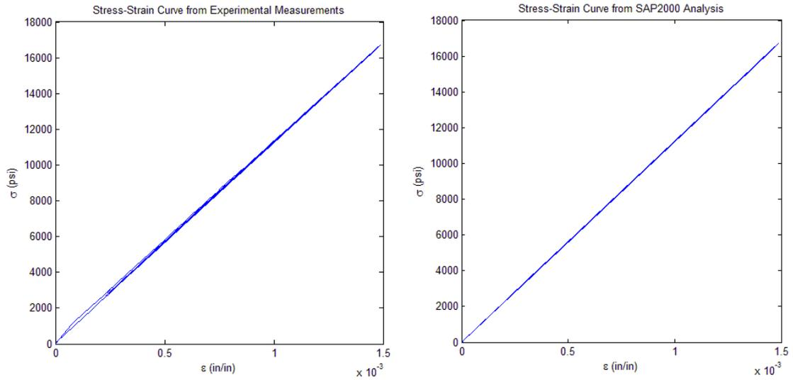
FIGURE 6.6: Experimentally-observed stress-strain relationship and analytically-simulated stress-strain relationship
