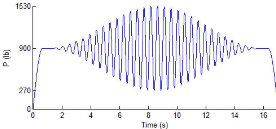
FIGURE 6.4: Load  $P$  applied to transmission tower model for linear elastic simulation
