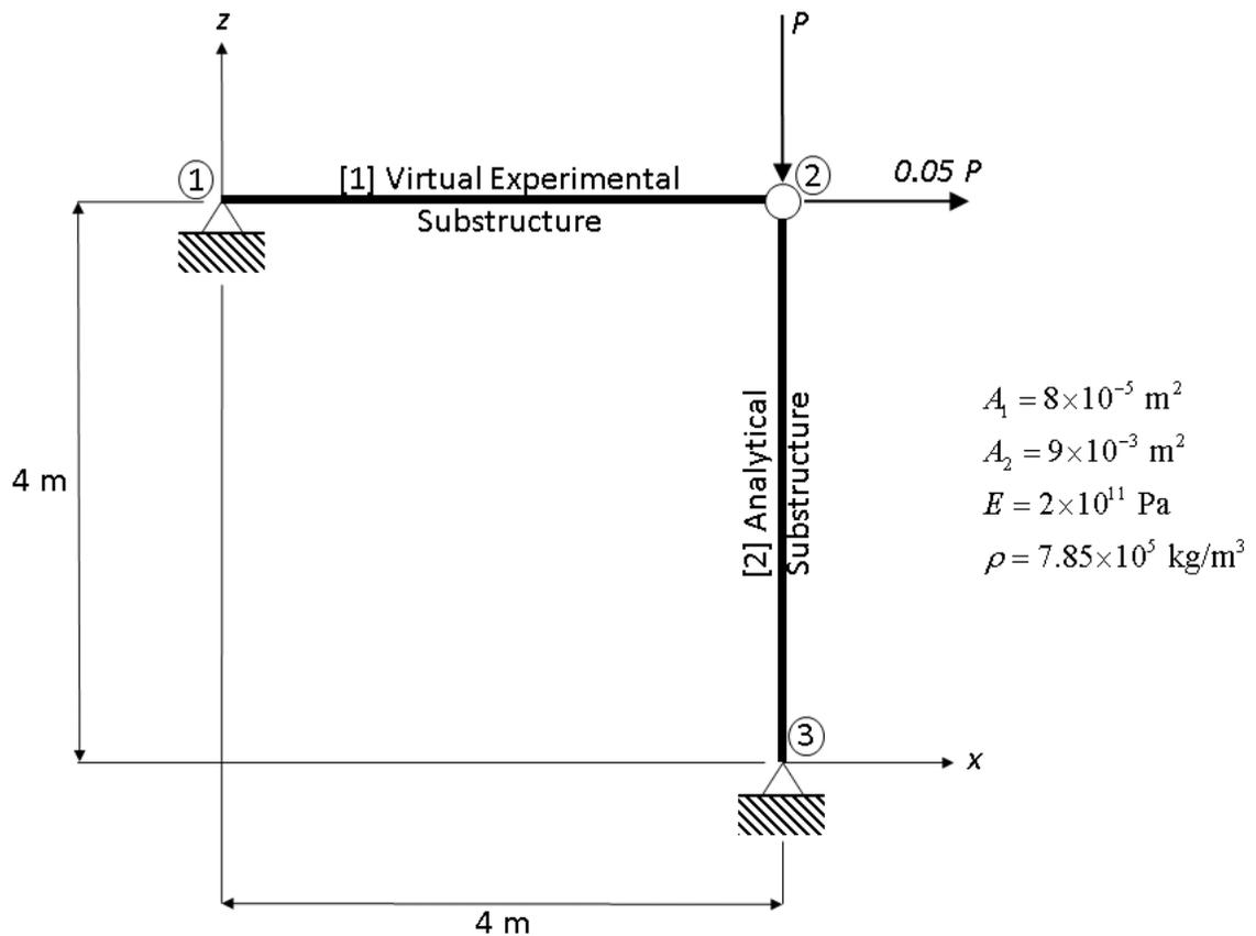
FIGURE 5.2: Simple two-dimensional truss model
