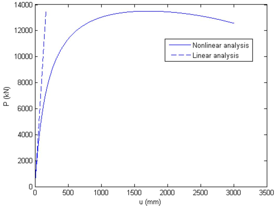
FIGURE 3.3: Load-displacement curves for static analysis of structure in Figure 3.2
