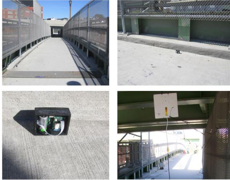
FIGURE 3.7: Sensors on bridge deck (top left). Individual accelerometer (top right). Wireless accelerometer (bottom left). Receiving antenna (bottom right)
