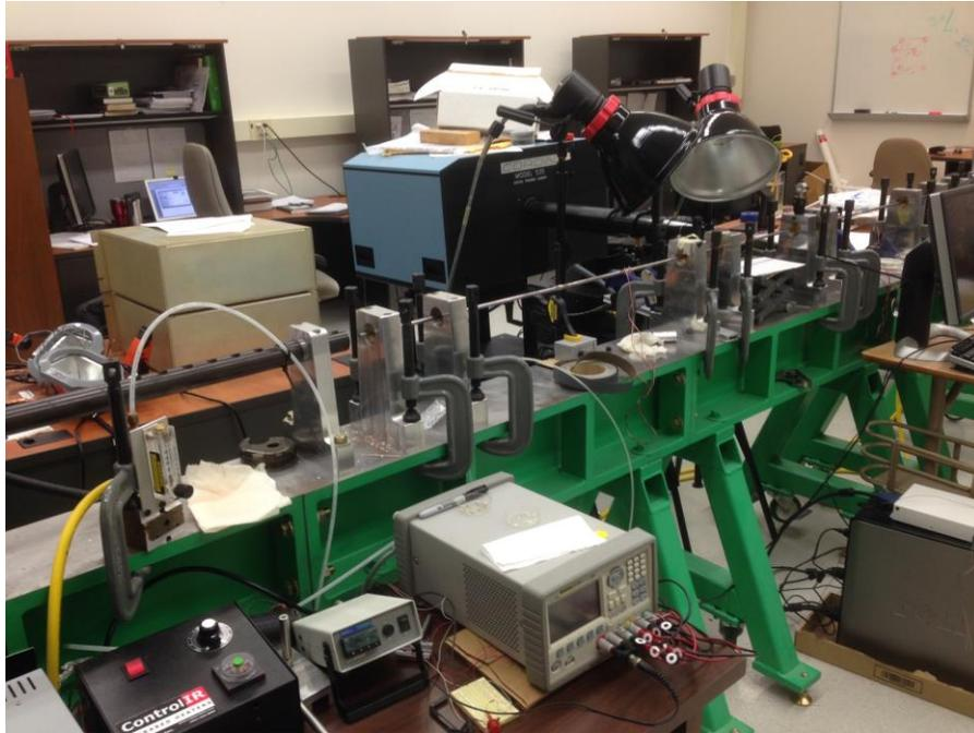
Figure 2.2: Picture of the Kolsky bar, high strain rate compression test setup used in this investigation.
