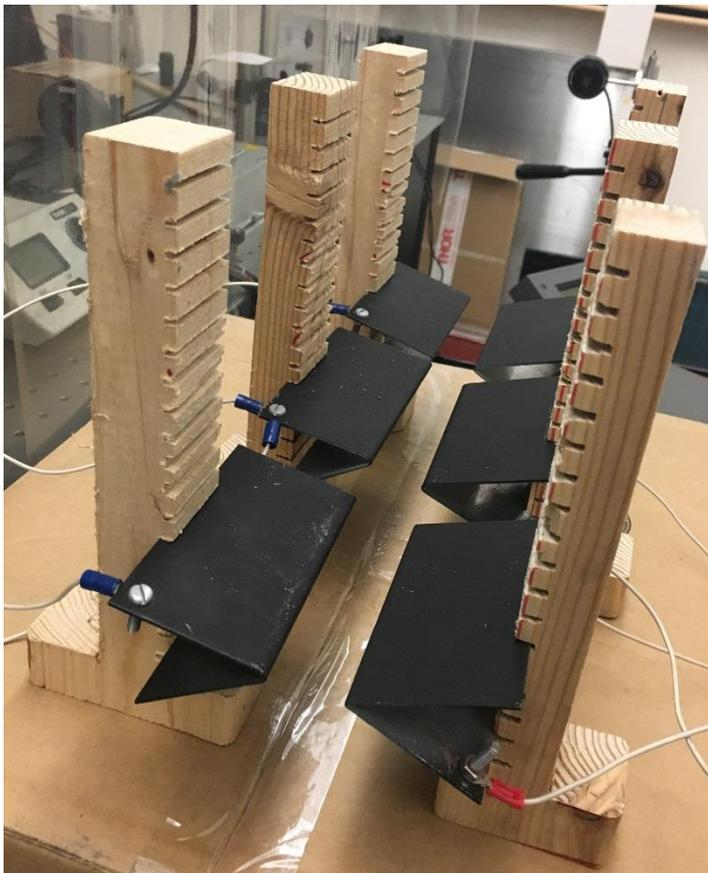
Fig. 14. 'V' shaped electrode system
