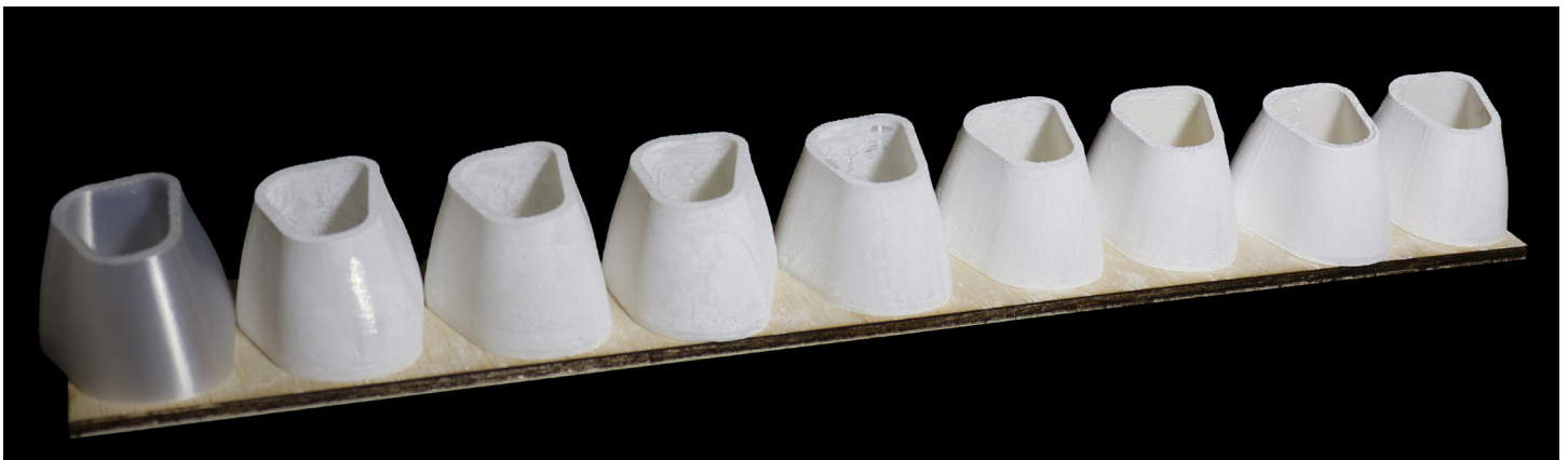
A SERIES OF CELLS WITH DIFFERENT AMOUNTS OF TiO 2 APPLIED FROM THE LEFT HAVING NONE TO THE RIGHT HAVING THE MOST.
