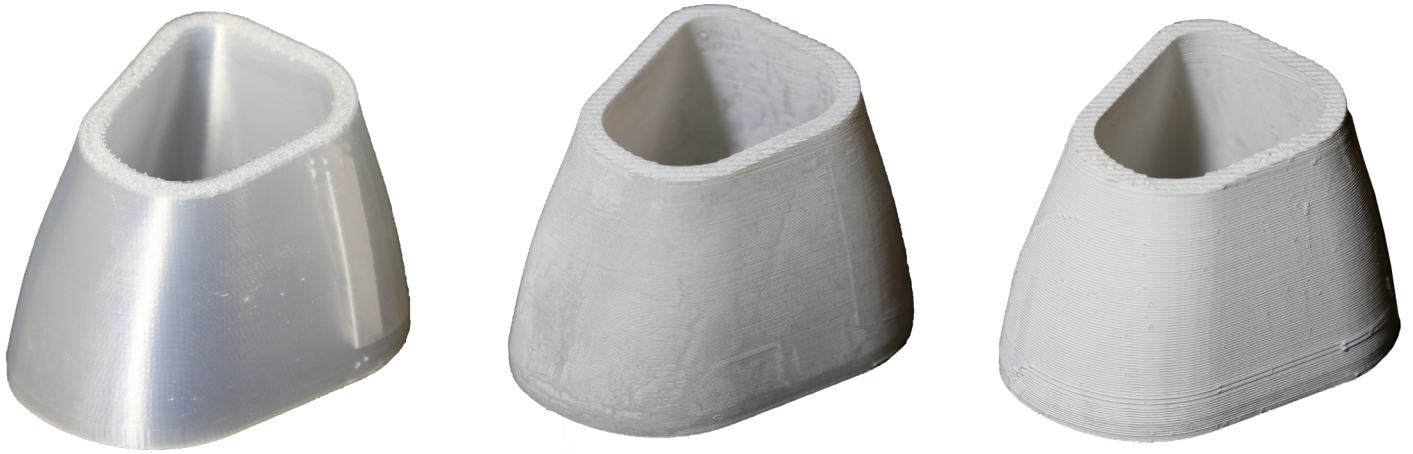
A THREE CELL STUDY MODEL OF THE PHYSICAL DIFFERENCE OF THE VISCOSITY OF THE TITANIUM DIOXIDE APPLIED TO A SINGLE CELL (TiO 2 ). LEFT IMAGE HAS NO TiO 2 . MIDDLE IMAGE HAS A LIGHT AMOUNT OF TiO 2 FROM A WATER-LIKE MIXTURE. RIGHT IMAGE HAS THE MOST TiO 2 WITH A PASTE LIKE MIXTURE.
